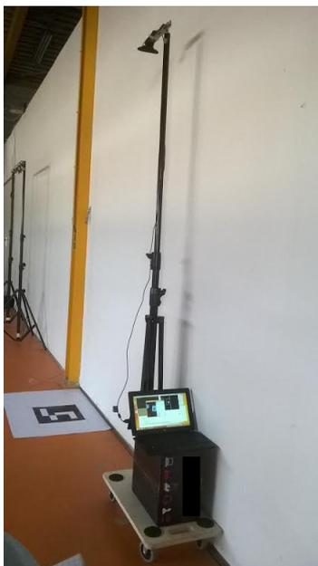
Figure 8: Camera mounted on a pole on a cart. The camera is connected to a mobile computer that processes the computer vision application.
