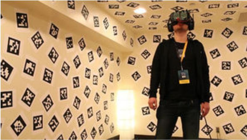
Figure 2: Inside-out tracking. A camera mounted on the head mounted display allows for pose estimation of the person's head. (image source: <https://www.oculus.com/en-us/blog/welcome-atman-binstock-chief-architect/>)
