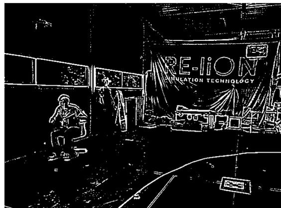
*Figure 23: the result of the adaptive threshold. One marker is present in the bottom right corner of the image.*
