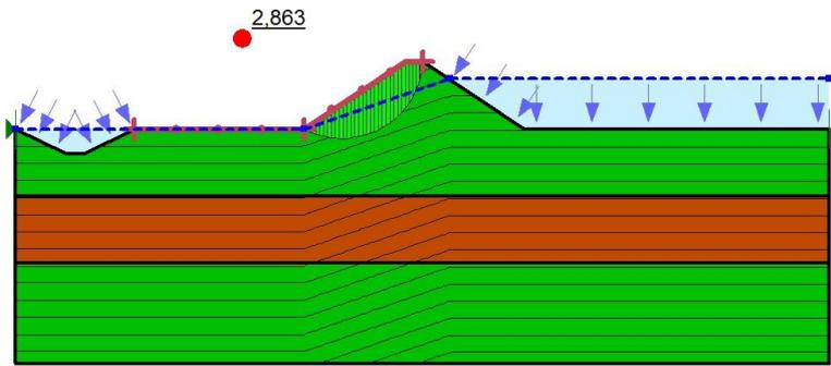
Figure 21: Result of the starting situation with 1.5 m of water and suspended particles.
