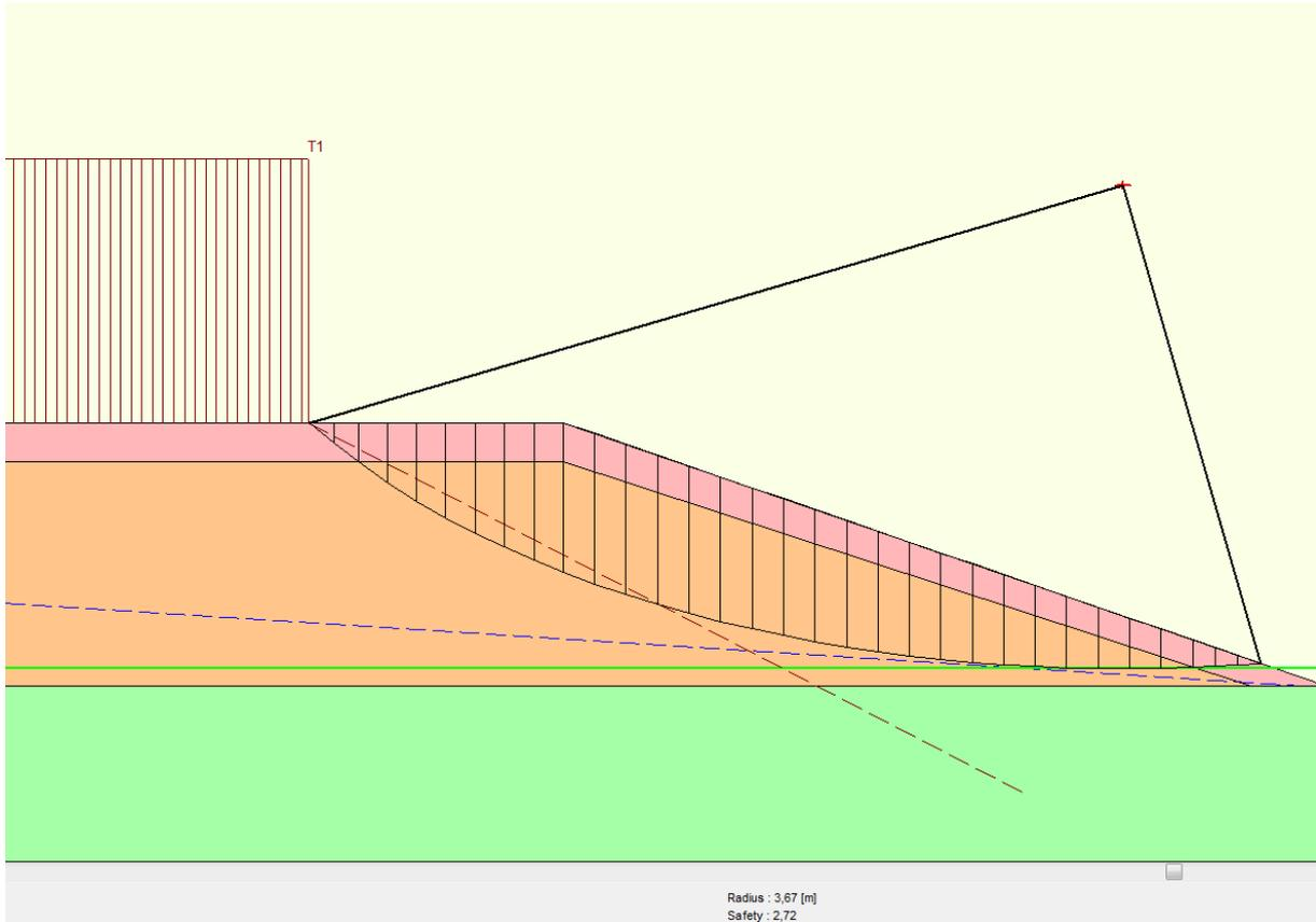
Figure 43: Model's calculation of the same manual slip surface.
