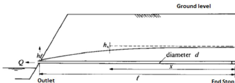
Figure 11: Decline of hydraulic head in a drainage series. Obtained from: (Cultuurtechnische vereniging, 2011, p. 532).
