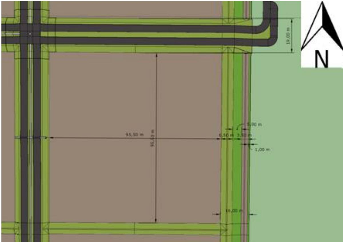
Figure 20: Dimensions near one test section.
