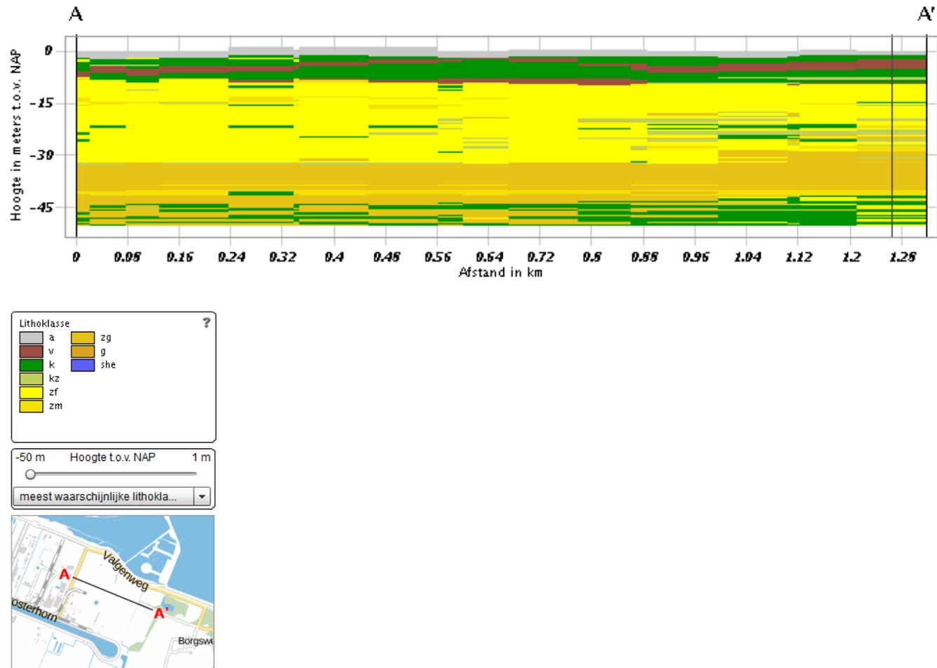
Figure 33: Most likely soils at the Delfzijl testing ground based on the GeoTOP model. Obtained from: (TNO, n.d.).
