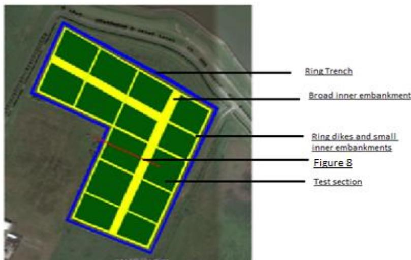
Figure 7: Top view preliminary layout testing ground at Delfzijl. Adapted from: (Ecoshape, 2016, p. 9).
