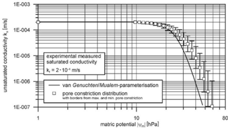
Figure 4: Dependency between unsaturated conductivity and matric potential of the weak gravelly sand. Obtained from: (Scheuermann & Bieberstein, 2007, p. 431).
