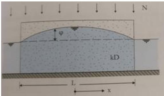
Figure 10: Parabolic shape of a horizontal discharge flow. Obtained from: (Brakenhoff, 2017).
