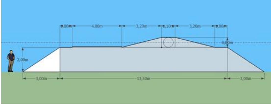
Figure 14: Profile of design two, very steep slope.
