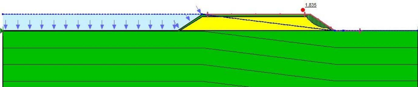
Figure 25: Stability inner sand dike covered by a 0.3m clay layer.
