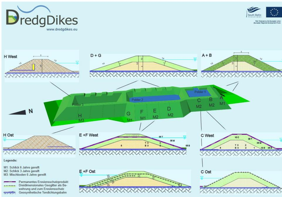
Figure 1: Test dike setup Rostock (German). Obtained from: (Dredgedikes, n.d.).
