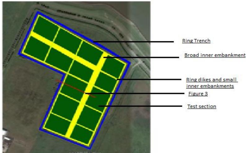
Figure 28: Current design of testing ground Delfzijl. Obtained from: (Ecoshape, 2016, p. 9).
