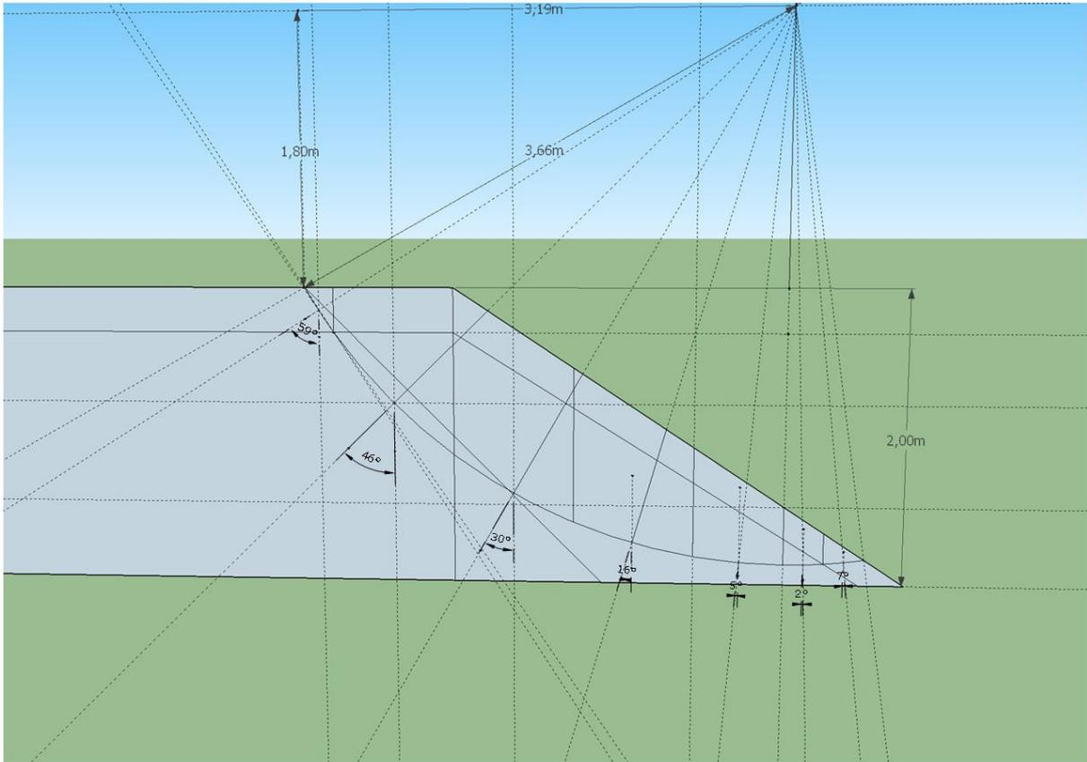
Figure 42: Dimensions used for the manual slip surface computation using Bishop.
