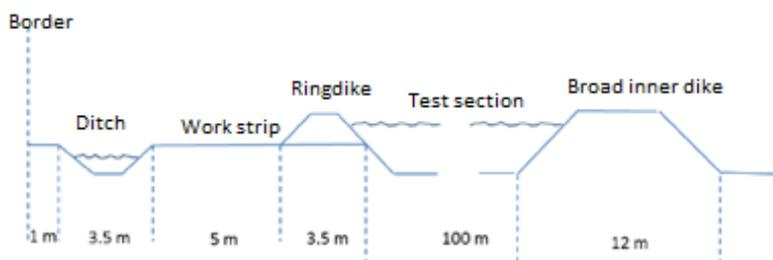
Figure 8: Cross section at red line of current Design Delfzijl. Adapted from: (Ecoshape, 2016, p. 9).
