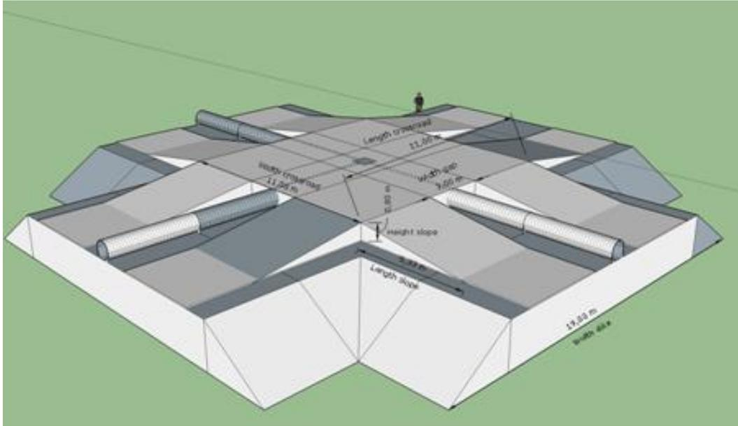
Figure 18: Crossroad of broad inner dike. Top left is North-side.
