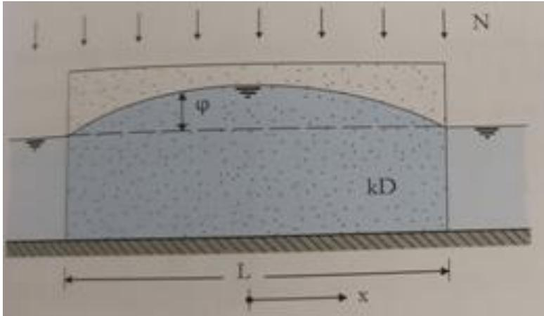
Figure 44: Horizontal discharge of the test section. Obtained from: (Brakenhoff, 2017).
