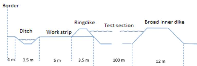
Figure 29: Profile red line of current design Delfzijl. Obtained from: (Ecoshape, 2016, p. 9).
