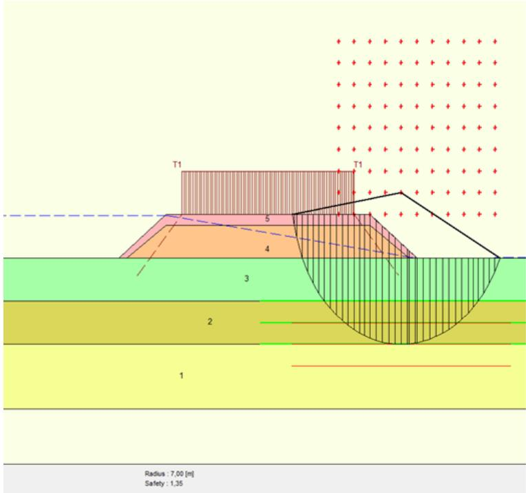
Figure 26: Stability dike with combination of vertical load and water pressure.
