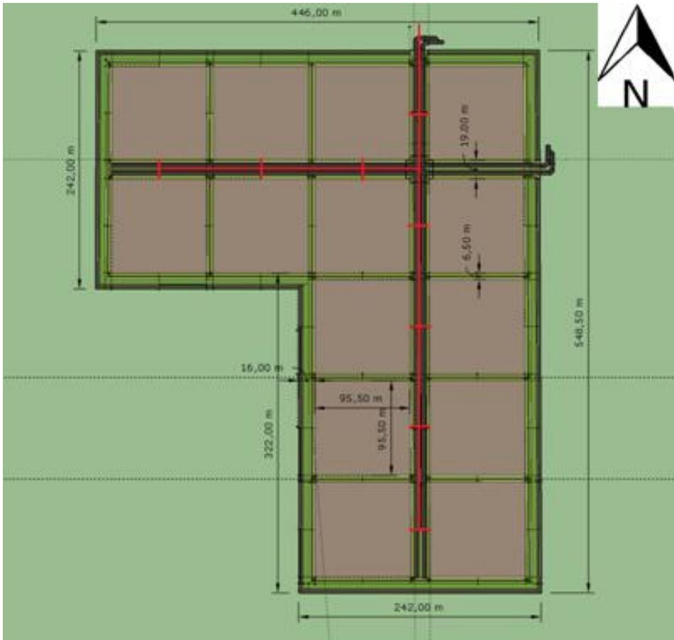
Figure 19: Dimensions of testing ground. The pipeline has been accentuated by the red line.
