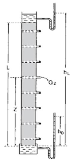
Figure 5: Measurement of hydraulic conductivity profiles down soil monoliths using interceptor drains. Obtained from: (Youngs, 2001, p. 12).
