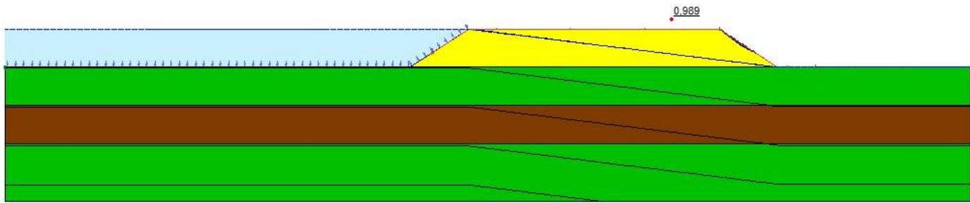
Figure 24: Stability inner sand dike.
