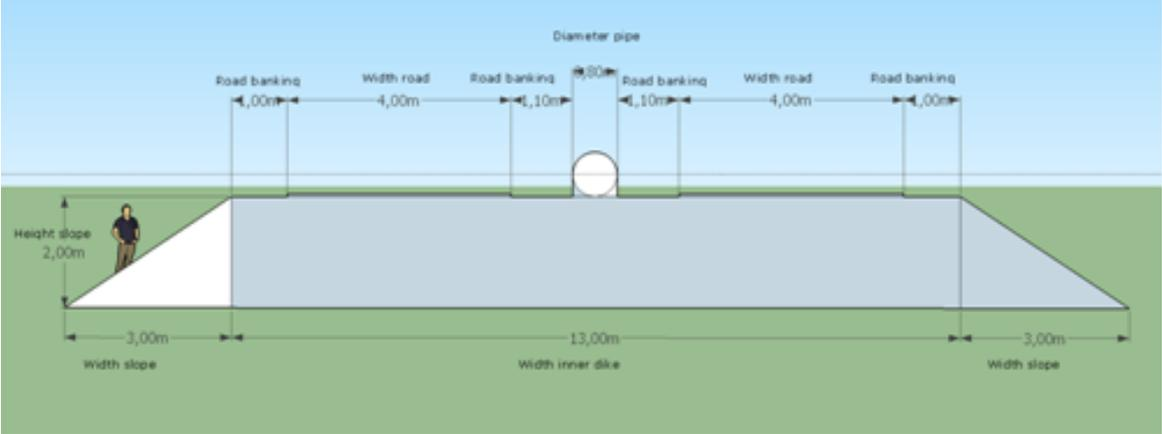
Figure 13: Profile of design one, broad inner dike.
