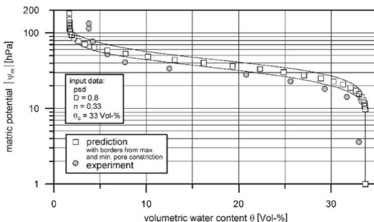
Figure 3: Dependency of the matric potential on the volumetric water content for weak gravelly sand. Obtained from: (Scheuermann & Bieberstein, 2007, p. 428).
