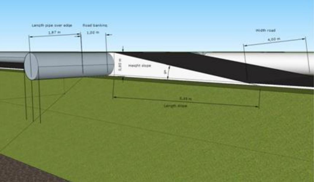
Figure 16: Slope over crossing pipeline on broad inner dike.
