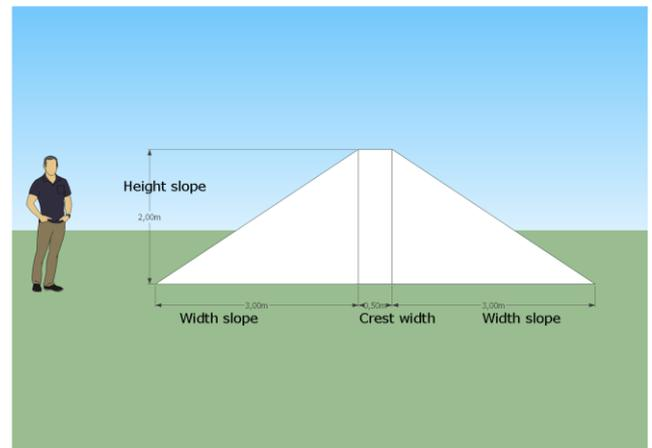
Figure 12: Dimensions ringdike & small inner embankment.
