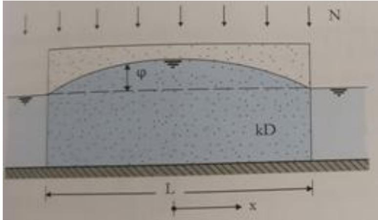
Figure 36: Horizontal discharge of the test section. Obtained from: (Brakenhoff, 2017).
