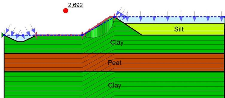
Figure 22: Result of a scenario where the silt has settled and the water has reached a height of 2 m instead of 1.5 m.
