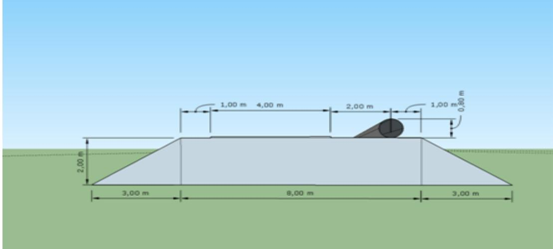
Figure 15: Profile of design three, no vehicles can cross the pipe during the compartment filling.
