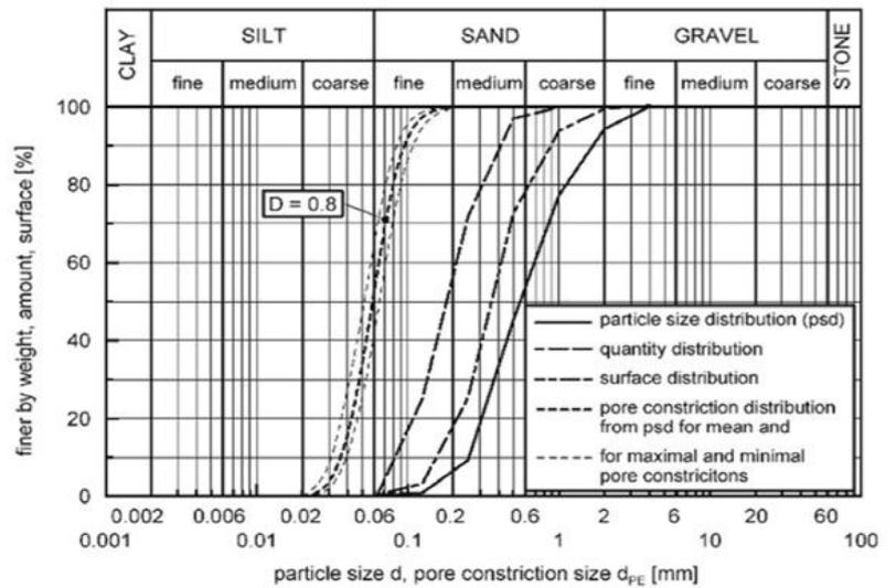
Figure 2: Particle size distribution for a weak gravelly sand as well as pore constriction distributions for mean pore constrictions for a relative density of  $D=0.8$ . Obtained from: (Scheuermann & Bieberstein, 2007, p. 426).
