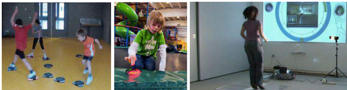
Figure 5. The jump patterns of children is motivated by the colour patterns of the tangible tiles (left) (Rijnbout, Graaf, & Schouten, 2015). The center image shows sensors on the trampoline foil that track jumper positions and adjust their LED's accordingly to signal the current game rules (Karoff, Elbæk, & Hansen, 2012). On the right Different equipments working together to allow jumping rope over distance (Denic & Charalambous, 2007).
