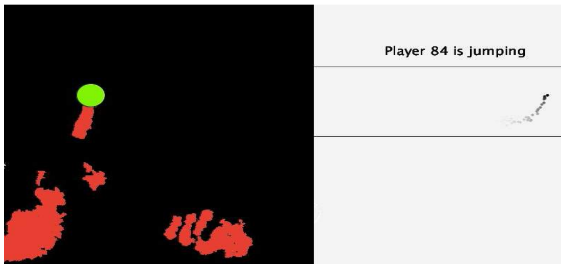
Figure 28, simulating jumps through finger movements, tracked by a Kinect.
