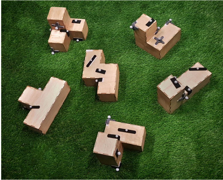
Figure 6.4: Blocks with OptiTrack markers attached to them.
