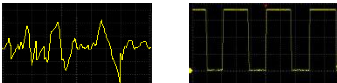
Figure 24: The output the IPM-165 sensor gives, left when no object is detected, right when an object is detected.
