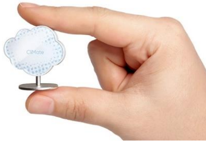
Figure 15: CliMate, a small device that can measure the immediate environment of the user [88]
