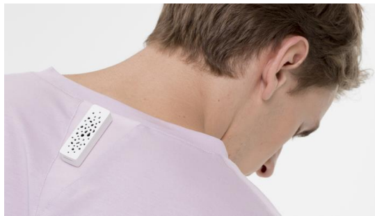
Figure 18: SynapseWear measures motion and the immediate environment of the user and can be attached to clothing [91]
