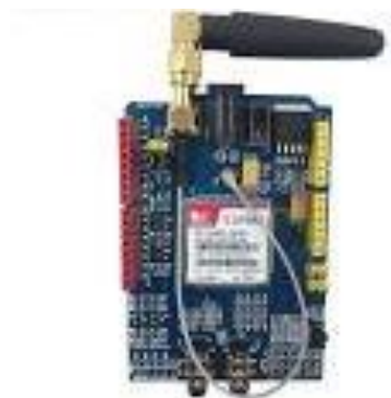
Figure 40: gsm/gps module can be used instead or together with a mobile phone
