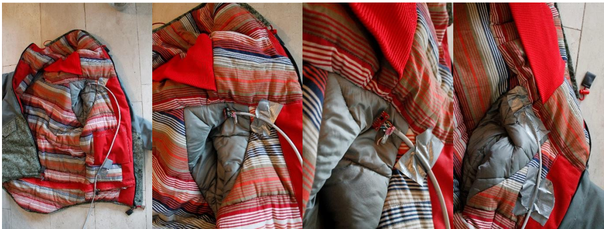
Figure 88: Position of the accelerometer at the left shoulder of the Sheltersuit
