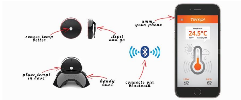
Figure 17: TempI can measure the temperature and humidity of the immediate environment of the user [90]
