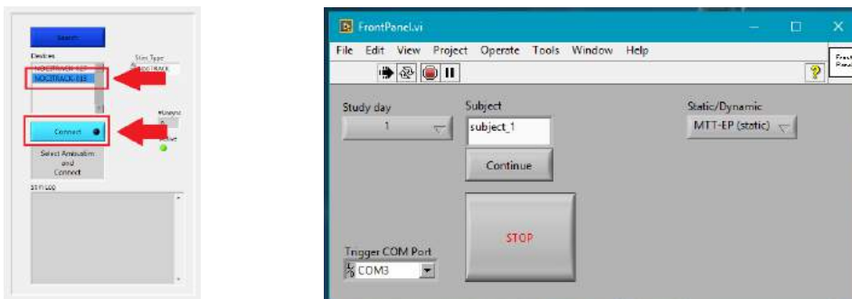
Figure 5: Left, the Bluetooth connection interface for the NociTRACK AmbuStim stimulator. First, press ‘Search’. If the correct stimulator device has been found (doublecheck with the number on the stimulator), press ‘Connect’. Right, the initial interface of the experimental application. Fill in the subject ID, confirm the COM port of the trigger generator in ‘Device Manager’, and press ‘Continue’.
