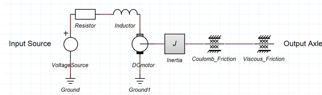
**Figure 2.1:** Standard ideal physical model of a motor
