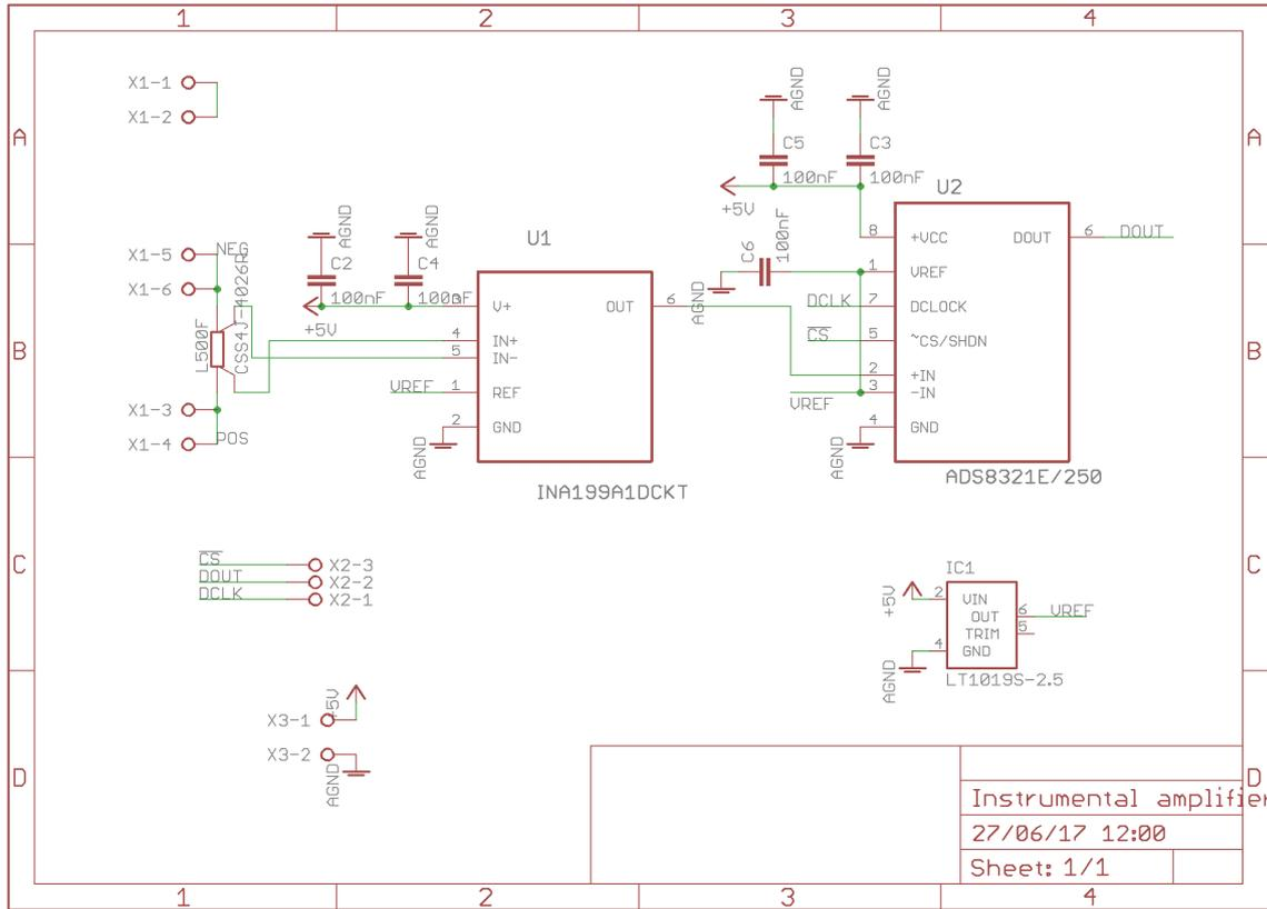
Figure A.1: Schematic of the current sensor
