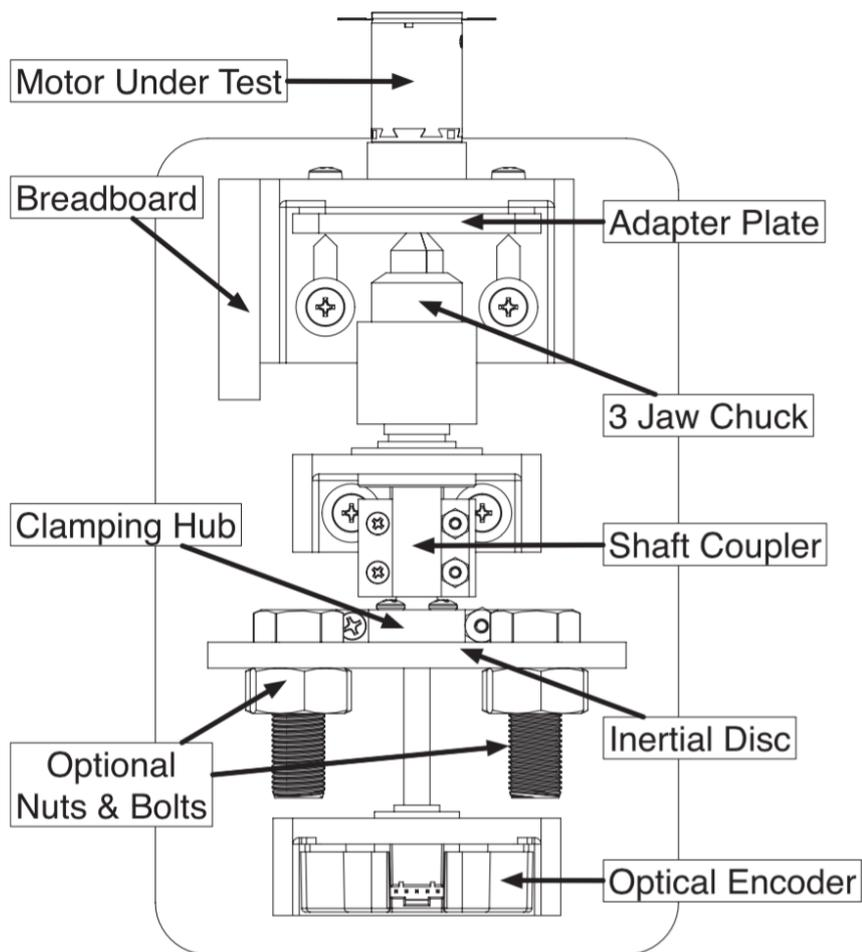
**Figure 1.2:** Labeled overhead drawing of RAPID assembly.
