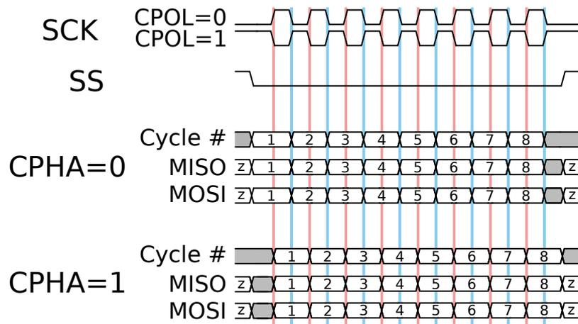
**Figure C.1:** Timing diagram showing clock polarity and phase, the red line represents CPHA=0 and the blue line CPHA=1
