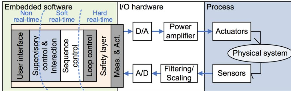
**Figure 2.5:** Diagram showing the general architecture of robotic control systems.
