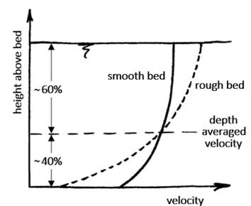
Figure 2.1: General vertical velocity profile of longitudinal component, adapted after Nortier and de Koning (1996).
