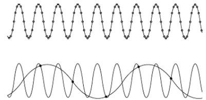
Figure 2.13: Principle of aliasing, where the upper signal is adequately sampled and the lower one is aliased due to undersampling.
