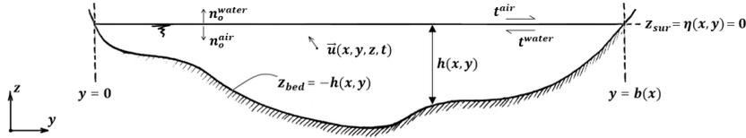
Figure 2.5: Arbitrary cross-section of a river and its parametrisation.
