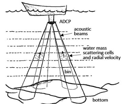
Figure 2.7: Acoustic beams of an ADCP, with bins and suspended particles, adapted after Simpson (2001).
