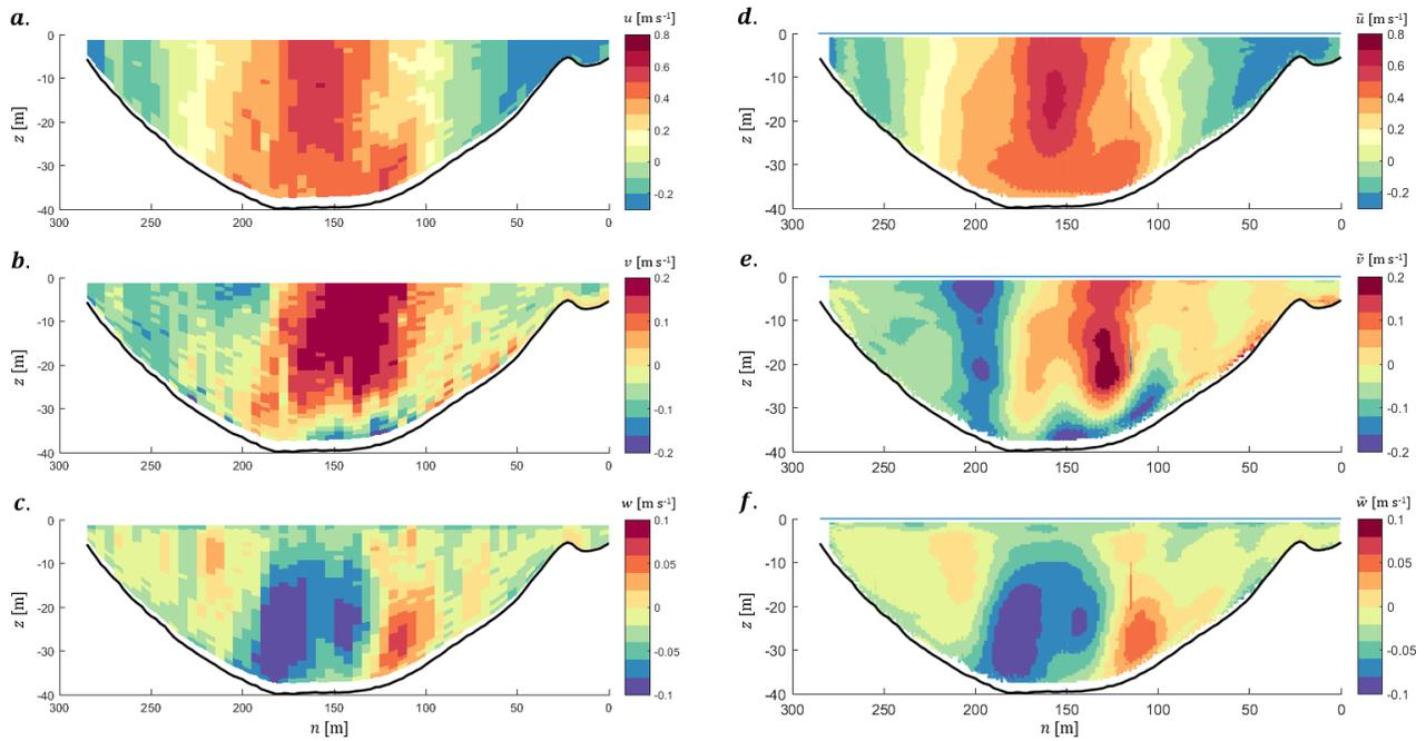
Figure 4.25: Decomposed processed velocity data of the third transect, which shows the processed (a) longitudinal, (b) lateral and (c) vertical velocity on the left. The modelled velocity in transect 3 for truncating at  $M = N = 16$  is shown on the right, where (d) shows the longitudinal, (e) the lateral and (f) the vertical velocity.
