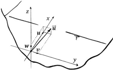
Figure 2.2: Vectorial velocity ( $\vec{u}$ ) with decomposed velocity components ( $u$ ,  $v$  and  $w$ ).
