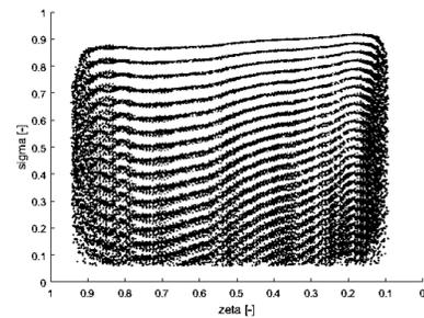
Figure 4.5: Normalised coordinates for all velocity locations in transect 1, without showing the actual magnitude of the measured velocity.
