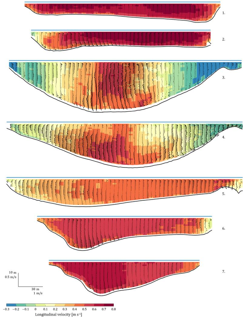
At transect 3 (Figure 4.2), located at the scour hole, the longitudinal flow is concentrated at the center, with two recirculating zones next to it. About 75% of the cross-sectional area and about 50% of the measured river width is discharging downstream. The remain part flows upstream along the edges mainly caused by the sudden increase in the cross-sectional area that results in an adverse water surface gradient (Vermeulen et al., 2015). Vertical shear
