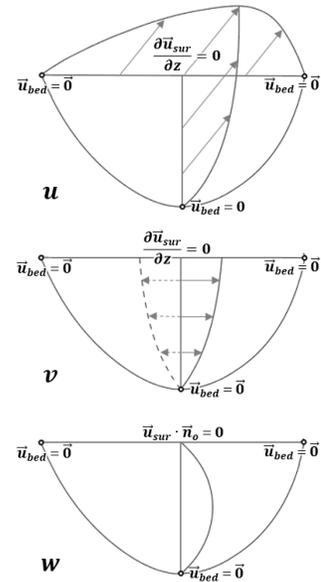
Figure 2.6: General river velocity profile with visualisation of boundary conditions for the three velocity components ( $u$ ,  $v$  and  $w$ ).
