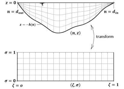
Figure 3.4: Transformation of  $nz$ -plane into  $\sigma$ - and  $\zeta$ -coordinates to obtain the normalised  $(\zeta, \sigma)$ -system.
