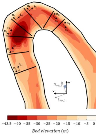
Figure 3.3: Average transect ( $nz$ -)planes with normal and tangential unit vectors of the transects in  $s$ - and  $n$ -direction, and an example of the principle of "rotation" for transect 1.
