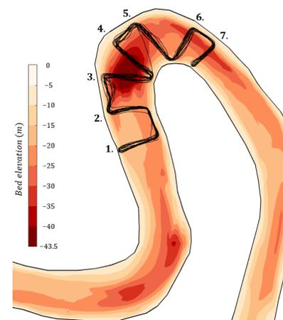
Figure 4.1: Measured track of the vessel with bed elevation and location of transects.
