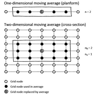
Figure 2.10: Schematic diagram of a spatial averaging procedure employed by VMT, after Parsons et al. (2013). Here,  $n_h$  and  $n_v$  represents the horizontal and vertical smoothing window size.
