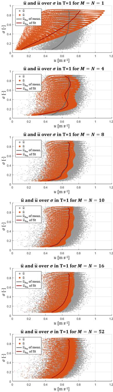
Figure 4.15: Measured and modelled longitudinal velocity over water depth with width averaged velocity over depth for different truncation numbers  $M$  and  $N$ .
