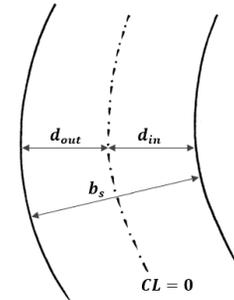
Figure 3.5: River bend with distance from centerline ( $CL$ ) to outer bank ( $d_{out}$ ) and from centerline to inner bank ( $d_{in}$ ), which results in the water surface width ( $b_s$ ) at a certain location.
