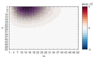
Figure 4.9: Values for amplitudes for the longitudinal velocity fit in transect 1, truncating at  $M = N = 52$ .
