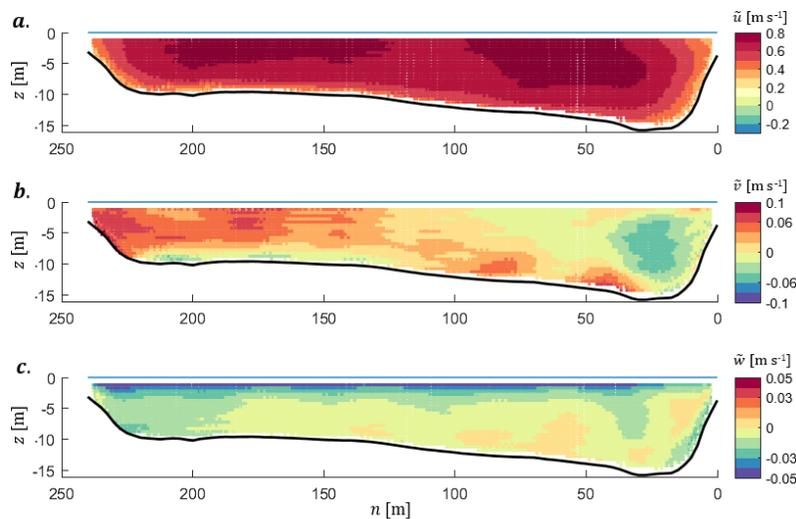
Figure 4.24: Modelled velocity in transect 1 for truncating at  $M = N = 16$ , where (a) shows the longitudinal velocity  $\tilde{u}$ , (b) the lateral velocity  $\tilde{v}$  and (c) the vertical velocity  $\tilde{w}$  in  $\text{m s}^{-1}$ .
