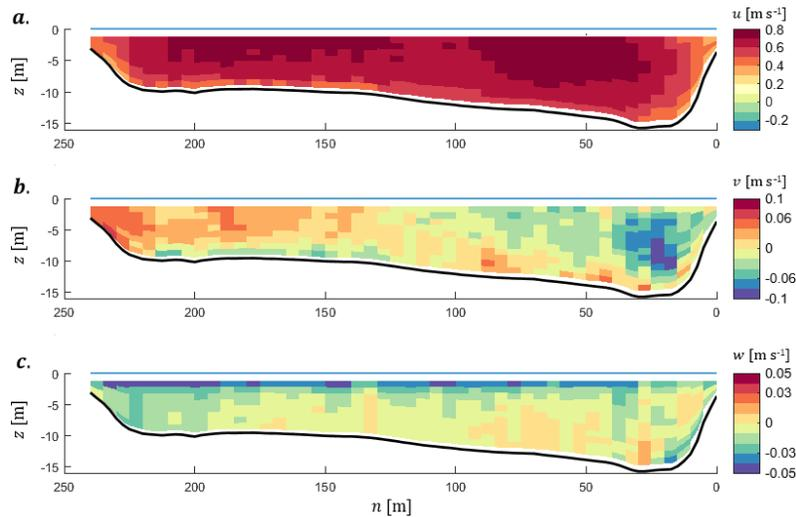
Figure 4.23: Decomposed velocity data of the first transect, which is processed according the proposed method of Vermeulen et al. (2014b). It shows the processed (a) longitudinal, (b) lateral and (c) vertical velocity.
