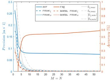
Figure 4.19: Accuracy and precision of longitudinal velocity fit ( $\bar{u}$ ) in transect 1.  $ser$  is the standard error of regression (in blue),  $rmse$  the root mean squared error (in blue), which is normalised as well (in red),  $rsq$  is  $R^2$  (in red). Maximum and minimum local averages of residuals ( $\bar{\epsilon}_z/\sigma_{max}/min$ ) are plotted in grey and pertain to the blue y-axis.
