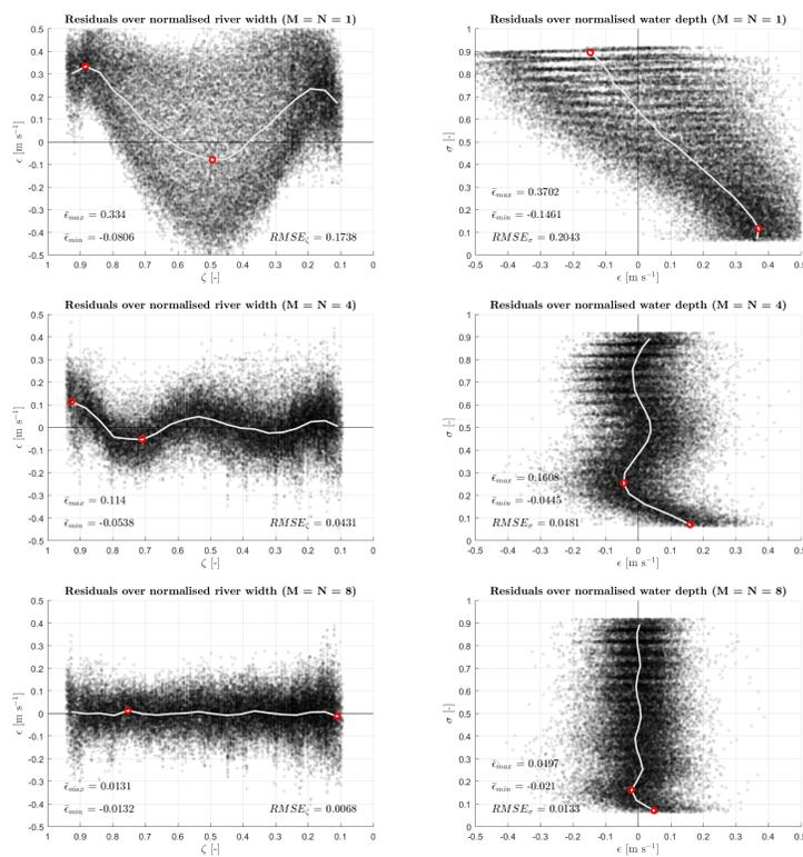
Figure 4.16: Residuals of longitudinal velocity fit over normalised width and depth for truncating at  $M = N = 1, 4$  and  $8$ .
