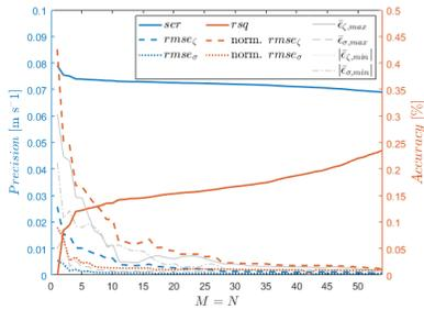
Figure 4.20: Accuracy and precision of lateral velocity fit ( $\bar{v}$ ) in transect 1.
