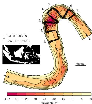
Figure 2.15: Overview of sharp river bend with bed elevation, the measured track and flow direction, adapted after Vermeulen et al. (2015).
