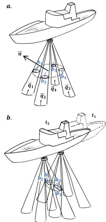
Figure 2.11: (a) Conventional flow data processing and (b) proposed method according to Vermeulen et al. (2014b).
