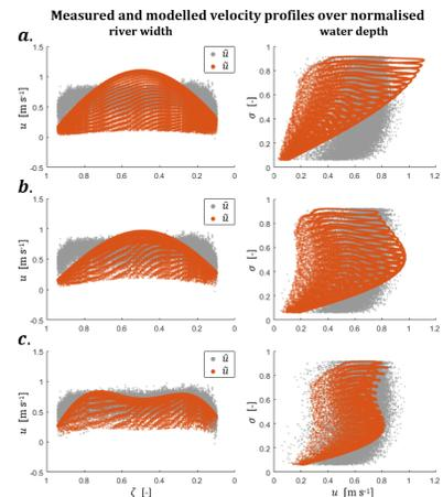
Figure 4.6: Principle of increasing truncation numbers for longitudinal velocity fit. Measured velocity ( $\hat{u}$ ) in grey and model fit ( $\bar{u}$ ) in red for (a)  $M = N = 1$ , (b)  $M = N = 2$  and (c)  $M = N = 3$ .
