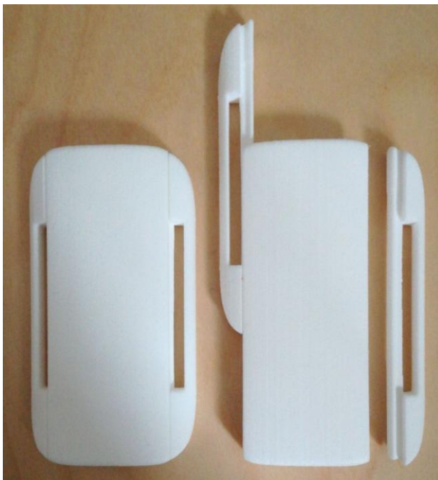
Picture 1, the redesigned sensor with the sides that can slide off
