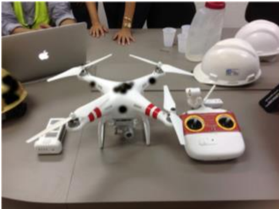
figure 2 - Example of simple multi-copter platform, DJI Phantom 2 (Irizarry & Costa, 2016)
