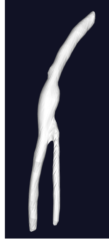
(b) Surface regularization by advection to the vessel wall and smoothing constraints
