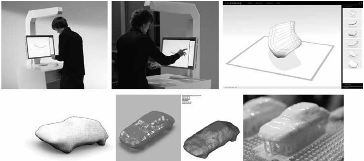
Fig. 4-7 Tacit-tangible modelling, virtual modelling, 3-D AM modelling, interface visualization and iterative process steps with RSFF tool.
