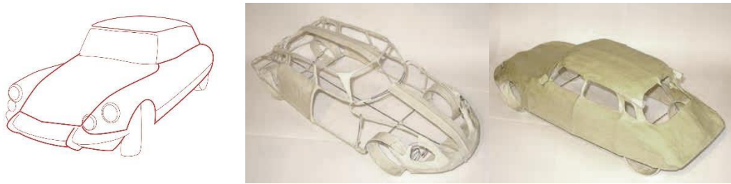
Fig. 2-12 Modelling in 3-D curved lines, shown is top-ranking model (see also Fig. 2-4 - DS1)
