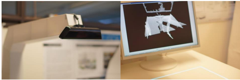
Fig. 4-13 Prototype Early Phase RSFF Tool with Kinect (left), Virtual Instances and Visualization
