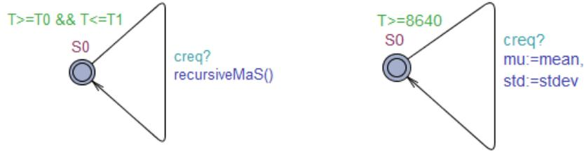
**Figure 5.9:** The two timed automata that were used to compute and to return the mean blood glucose concentration and corresponding standard deviation. The left automaton computes the mean blood glucose concentration and corresponding standard deviation between  $T_0$  and  $T_1$ . The right automaton writes the last computed values of the mean and standard deviation to the variables  $mu$  and  $std$ .
