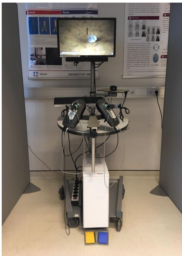
Figure 5. Showing the LapSim VR-Simulator including two ball-shaped elements with inserted endoscopes. On the display, the grasping task is shown.
