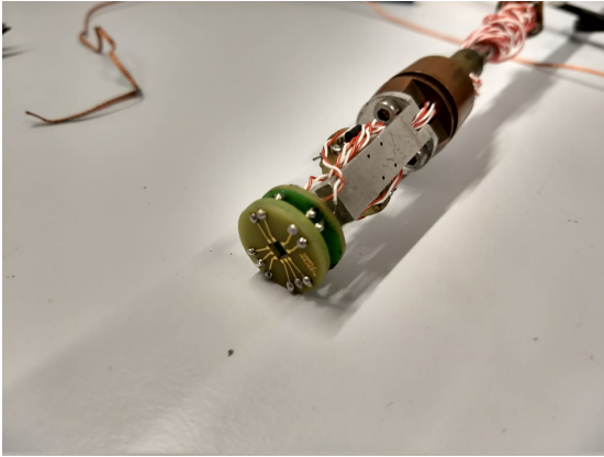
Figure 50. Close up of the PCB connected to the probe.
