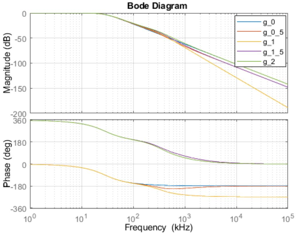
**Figure 3.8:** Bode plot of the transfer function of the model in Figure 3.1 with second order filter and different feedback gains  $g_0$ , 0.5, 1, 1.5 and 2
