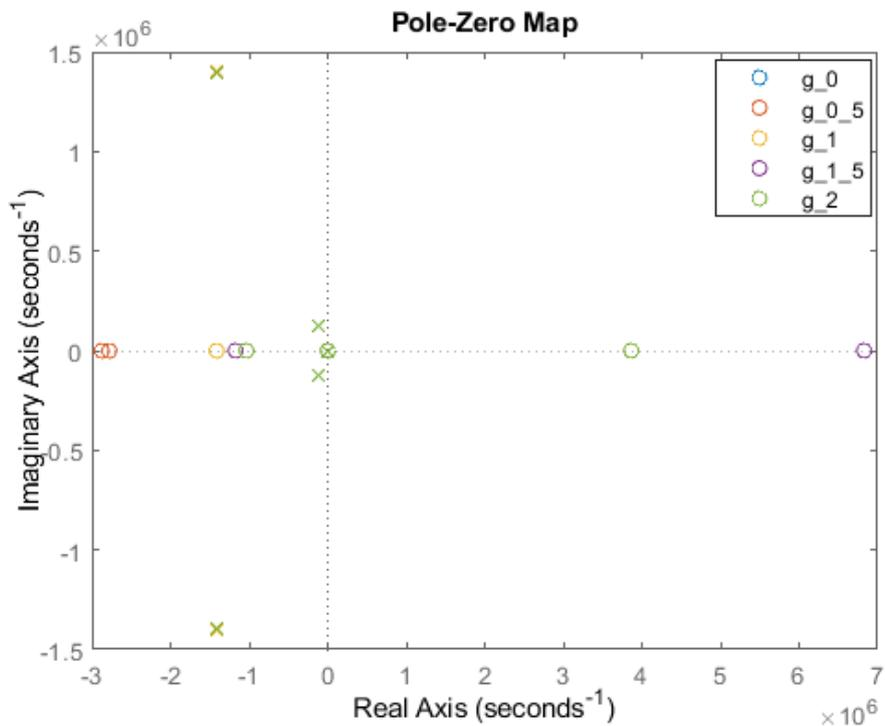
**Figure 3.9:** Pole-zero plot of the model in Figure 3.1 with second order filter and different feedback gains 0,1,10 and 50 (represented in angular frequency)
