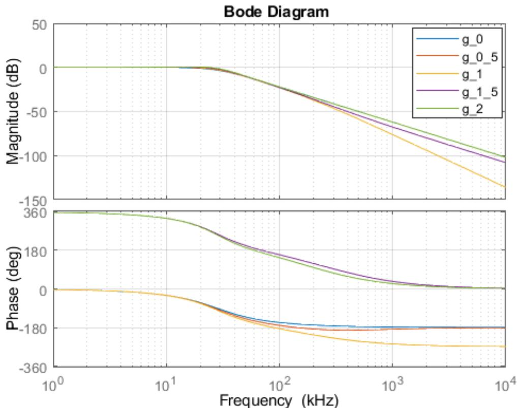
**Figure 3.2:** Bode plot of the transfer function of the model in Figure 3.1 with first order filter and different feedback gains  $g$  0, 0.5, 1, 1.5 and 2
