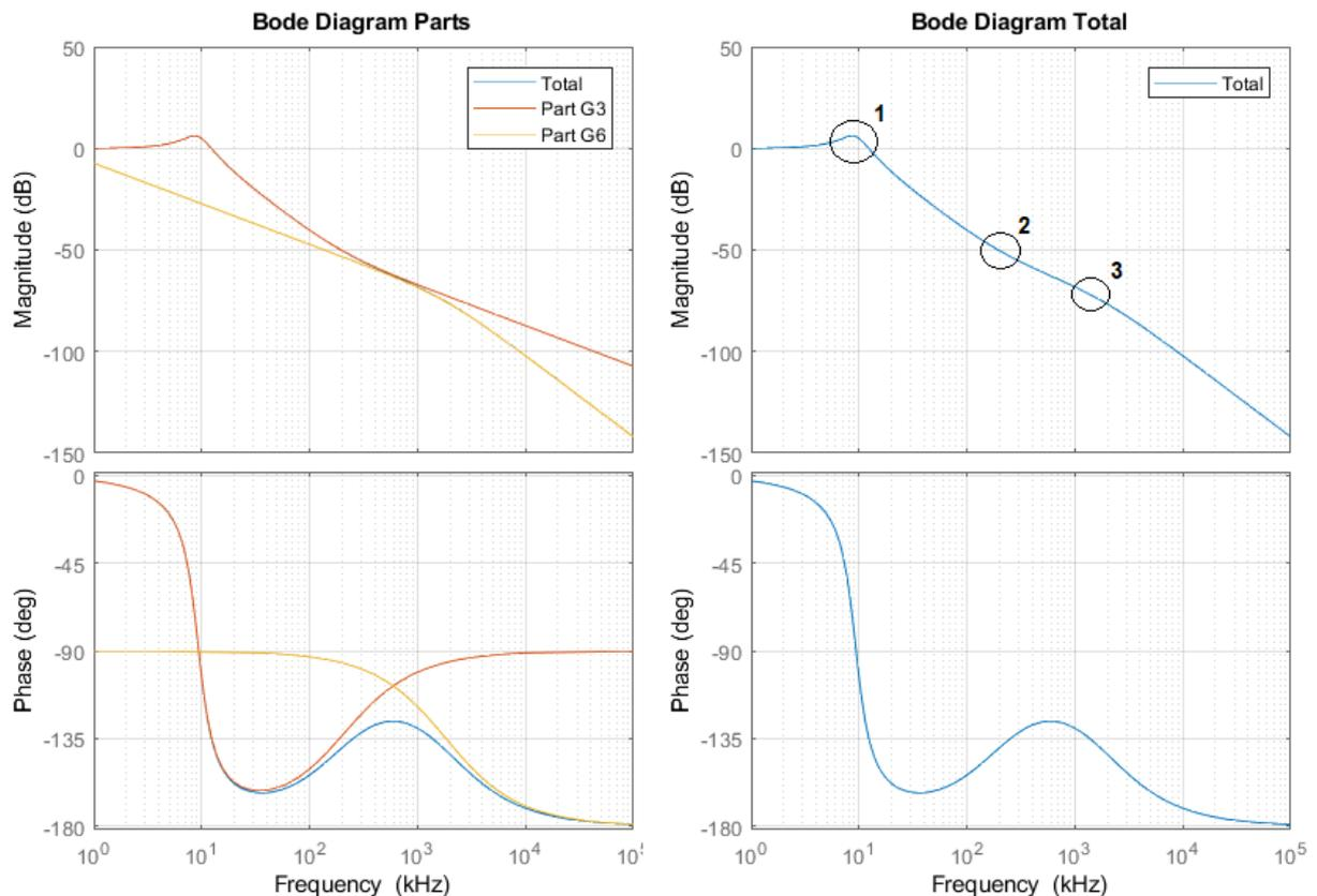
**Figure 2.5:** Bode plot of smaller transfer function which describe the transfer function of Equation 2.2(total) with a gain  $g$  of 10
