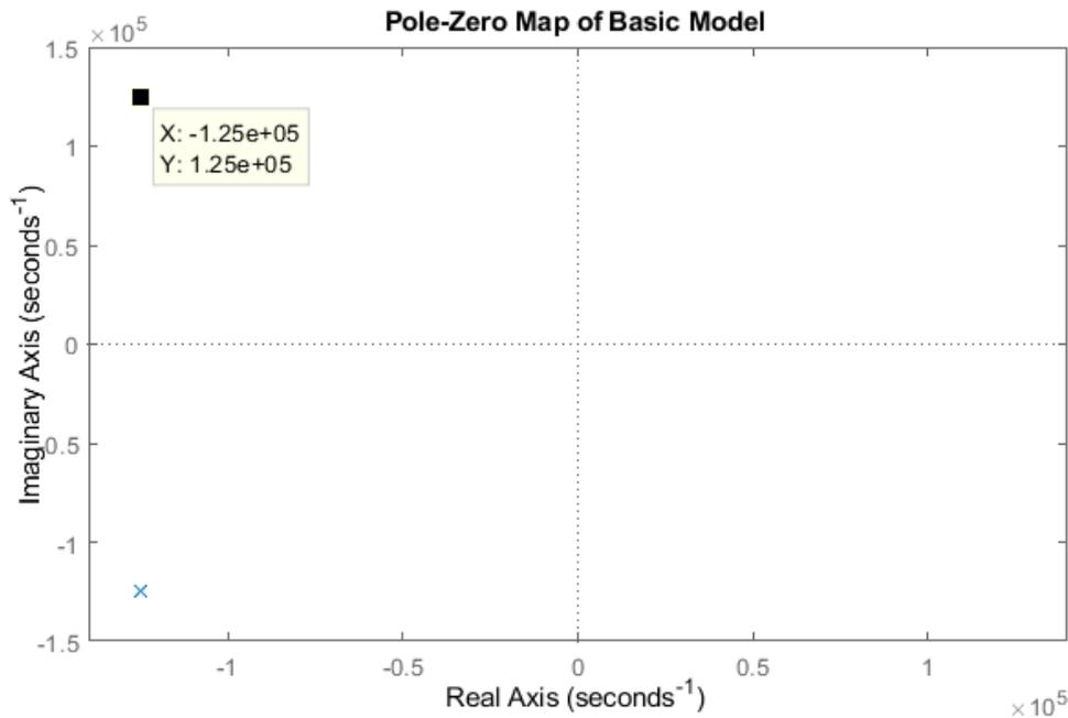
**Figure 1.3:** Pole-Zero plot of the model in Figure 1.1 (represented in angular frequency)
