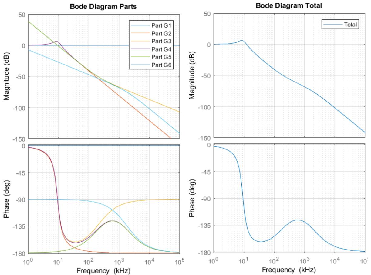
**Figure F.1:** Bode plot of all smaller transfer function of model 2.1 with a first order filter and gain  $g$  of 10
