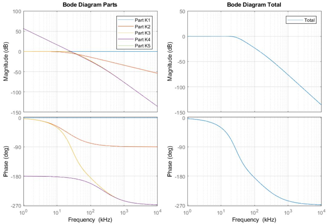
**Figure F.5:** Bode plot of all smaller transfer function of model 3.1 with a first order filter and gain  $g$  of 1
