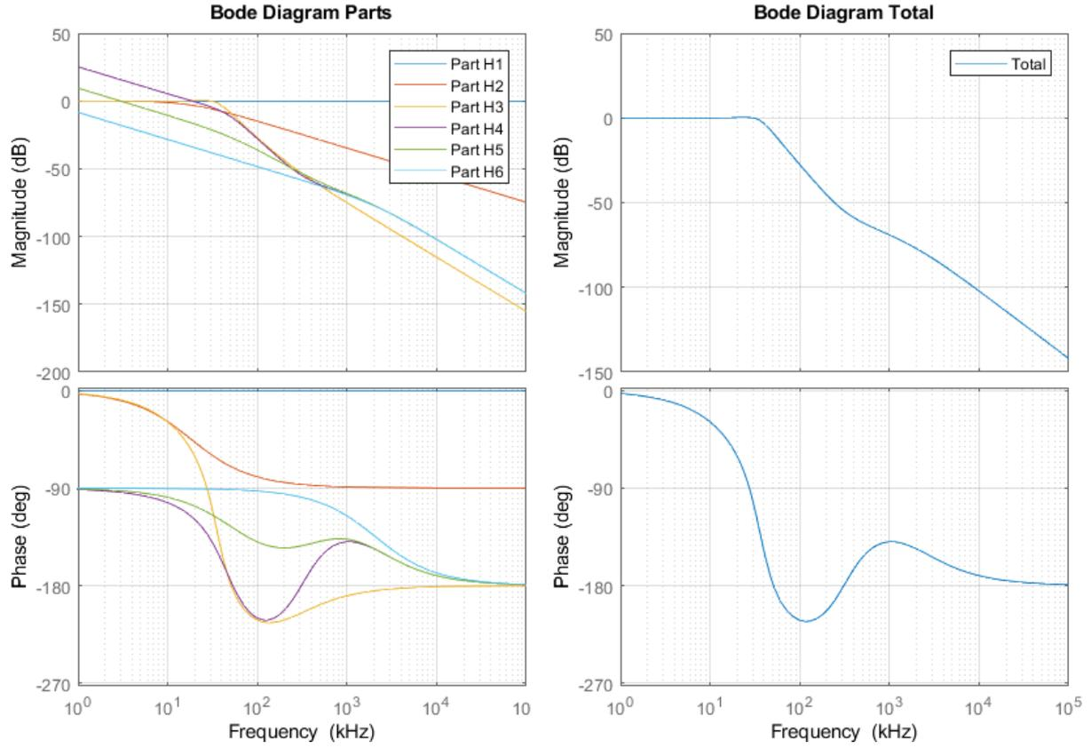
**Figure F.3:** Bode plot of all smaller transfer function of model 2.1 with a second order filter and gain  $g$  of 10
