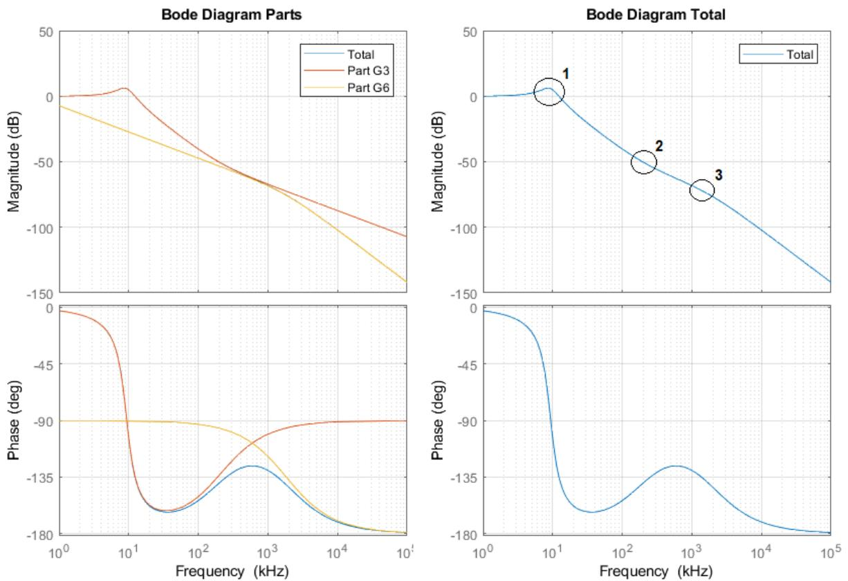
**Figure F.2:** Bode plot of final smaller transfer function of model 2.1 with a first order filter and gain  $g$  of 10
