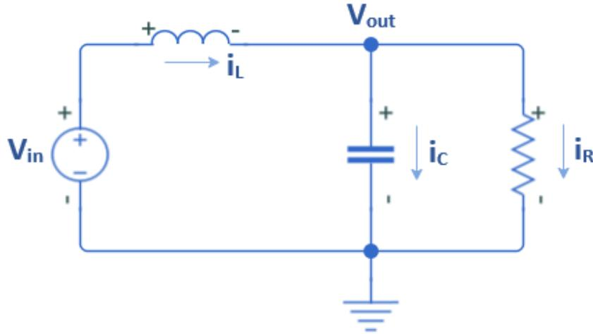
Figure A.1: Circuit model of a class D amplifier
