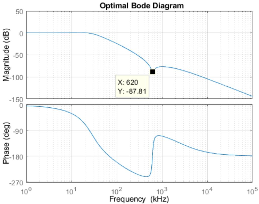
**Figure 2.13:** Optimal Bode plot of the model in Figure 2.1 with second order filter. Magnitude at 620 kHz is decreased from -53.7 dB till -87.8 dB.
