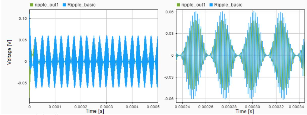
**Figure 2.8:** Optimal time domain plot of the model in Figure 2.1 with first order filter. The output voltage ripple amplitude is reduced from 60.8 mV (ripple\_basic) till 48.9 mV (ripple\_out1) .
