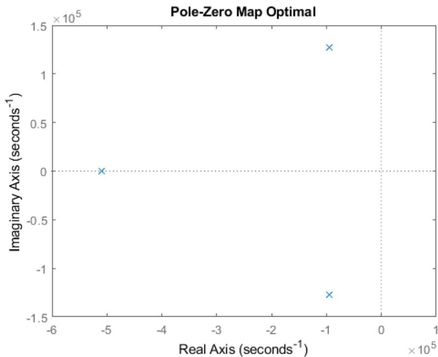
**Figure 3.6:** Optimal pole-zero plot of the model in Figure 3.1 with first order filter (represented in angular frequency)
