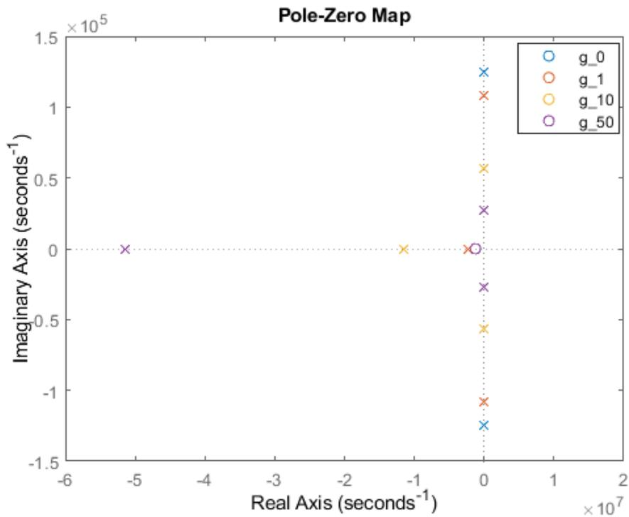
**Figure 2.3:** Pole-zero plot of the model in Figure 2.1 with first order filter and different feedback gains 0,1,10 and 50 (represented in angular frequency)
