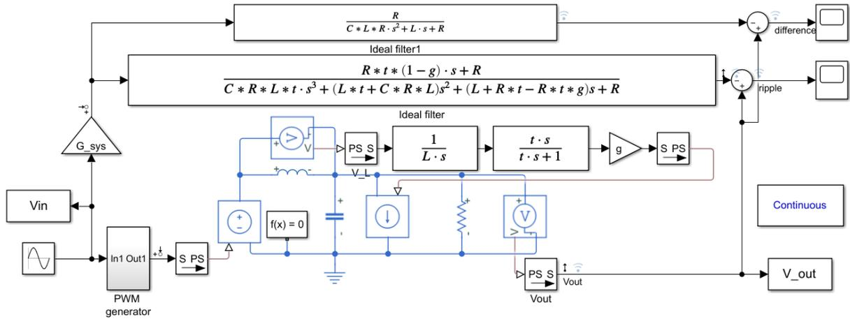
Figure E.4: Measured circuit model of first order inductor feedback
