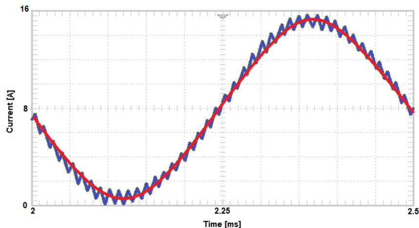
**Figure 2:** Red: signal current. Blue: signal current with the ripple current.
