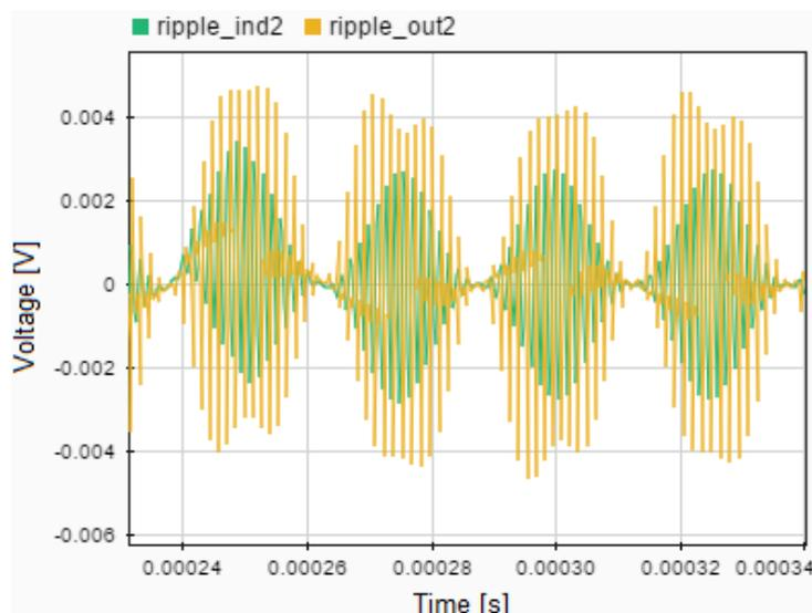
**Figure 4.2:** Output voltage ripple of Out2 and Ind2
