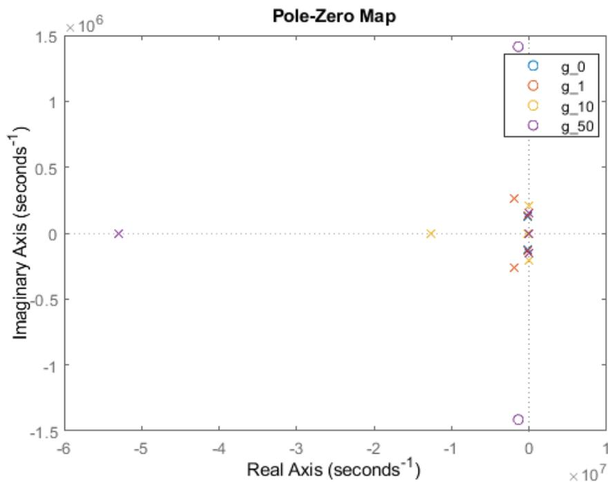
**Figure 2.10:** Pole-zero plot of the model in Figure 2.1 with second order filter and different feedback gains 0,1,10 and 50 (represented in angular frequency)
