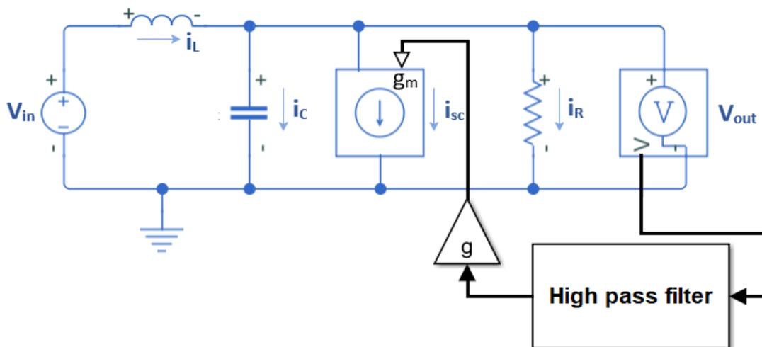
Figure 2.1: Circuit model of design with feedback from the output voltage
