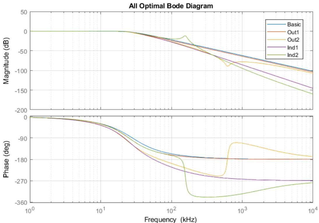
**Figure 4.1:** Optimized frequency responses. Basic = basic model. Out1 = model with feedback from the output voltage with first order filter. Out2 = model with feedback from the output voltage with second order filter. Ind1 = model with feedback from the inductor voltage with first order filter. Ind2 = model with feedback from the inductor voltage with second order filter.
