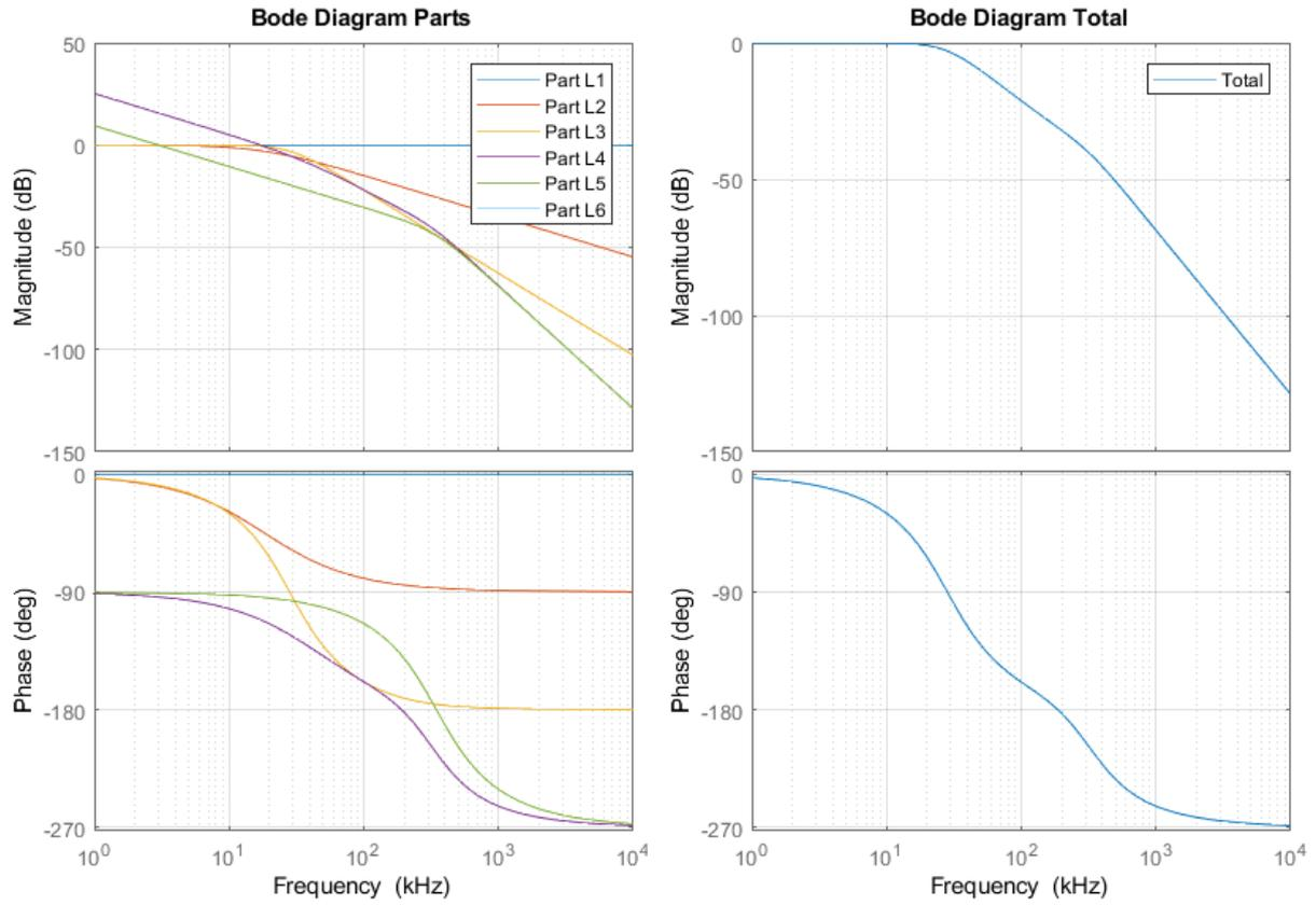
**Figure F.7:** Bode plot of all smaller transfer function of model 3.1 with a second order filter and gain  $g$  of 1
