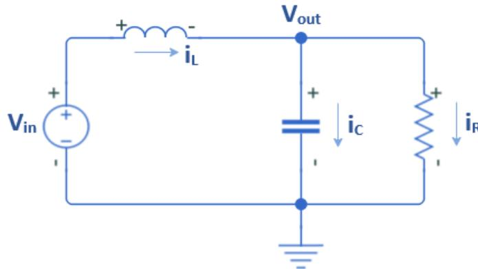
Figure 1.1: Circuit model of a class D amplifier
