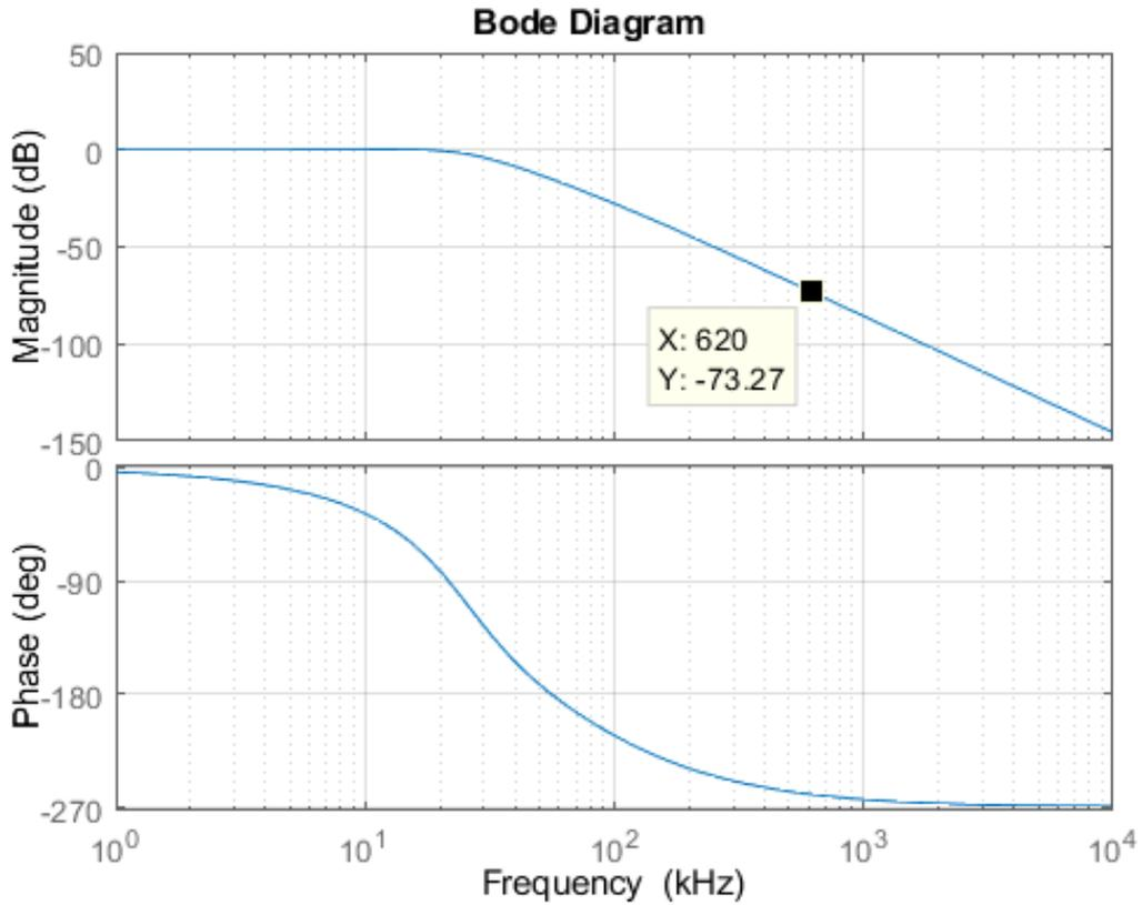
**Figure 3.5:** Optimal Bode plot of the model in Figure 3.1 with first order filter. The magnitude at 620 kHz decreases from -53.3 dB to -73.3 dB .
