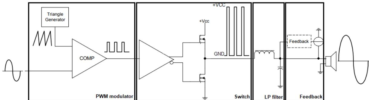
**Figure 1:** Class D amplifier with an active filter feedback
