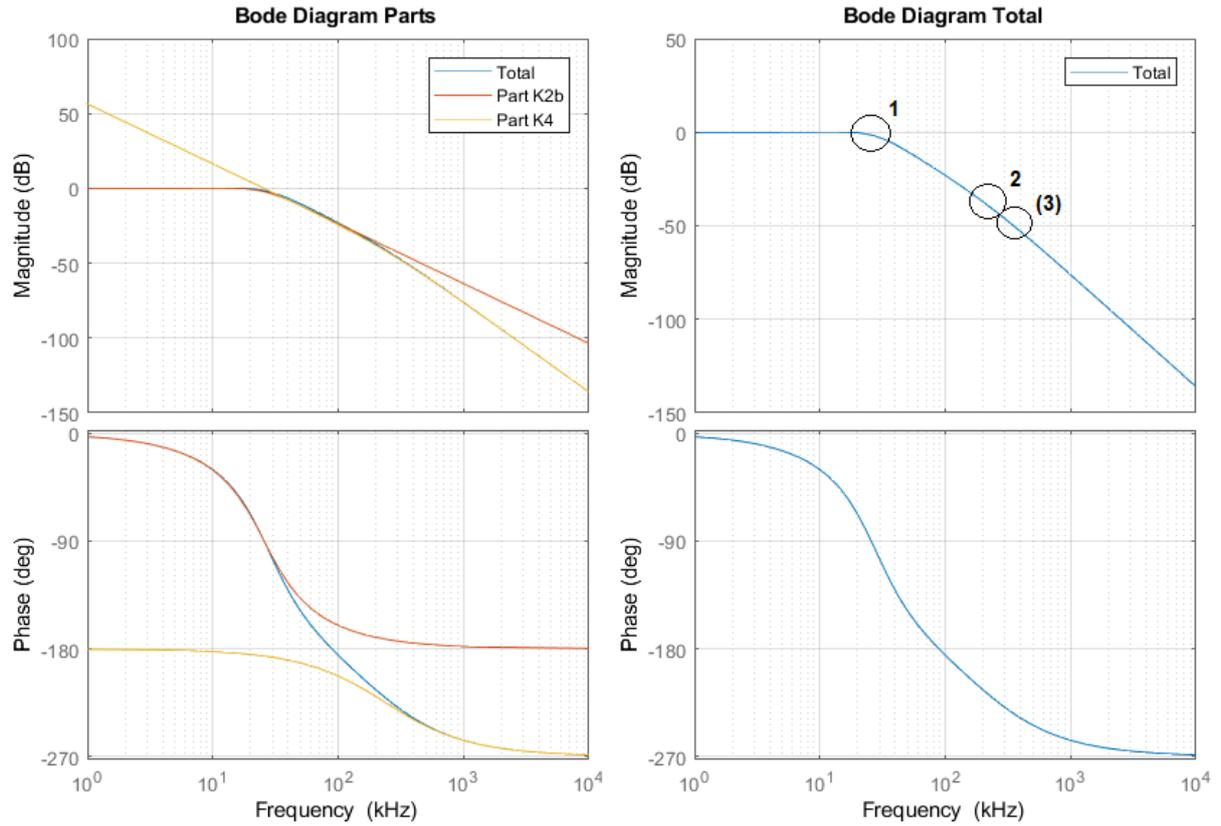
**Figure 3.4:** Bode plot of smaller transfer function which describe the transfer function of Equation 3.1(total) with a gain  $g$  of 1
