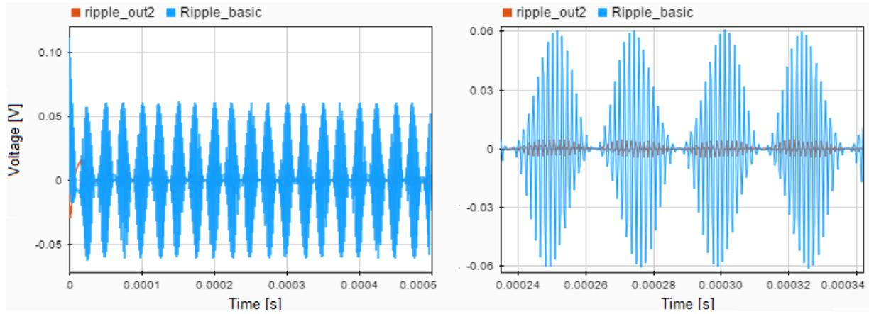
**Figure 2.15:** Optimal time domain plot of the model in Figure 2.1 with second order filter. Output ripple voltage amplitude is reduced from 60.8 mV (ripple\_basic) till 4.65 mV (ripple\_out2).
