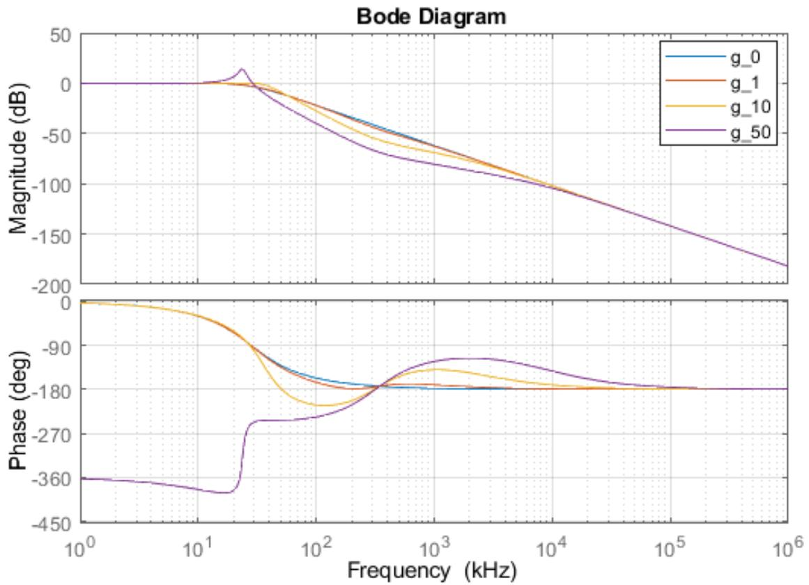
**Figure 2.9:** Bode plot of transfer function of model 2.1 with a second order filter and different feedback gains 0,1,10 and 50
