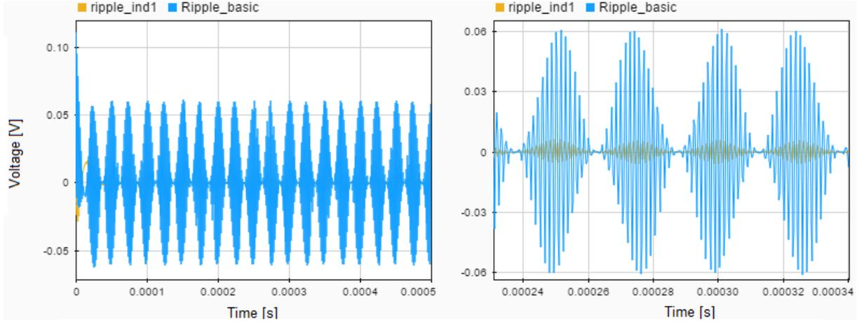
**Figure 3.7:** Optimal time domain plot of the model in Figure 3.1 with first order filter. The output voltage ripple amplitude is reduced from 60.8 mV (ripple\_basic) to 6.21 mV (ripple\_ind1) .
