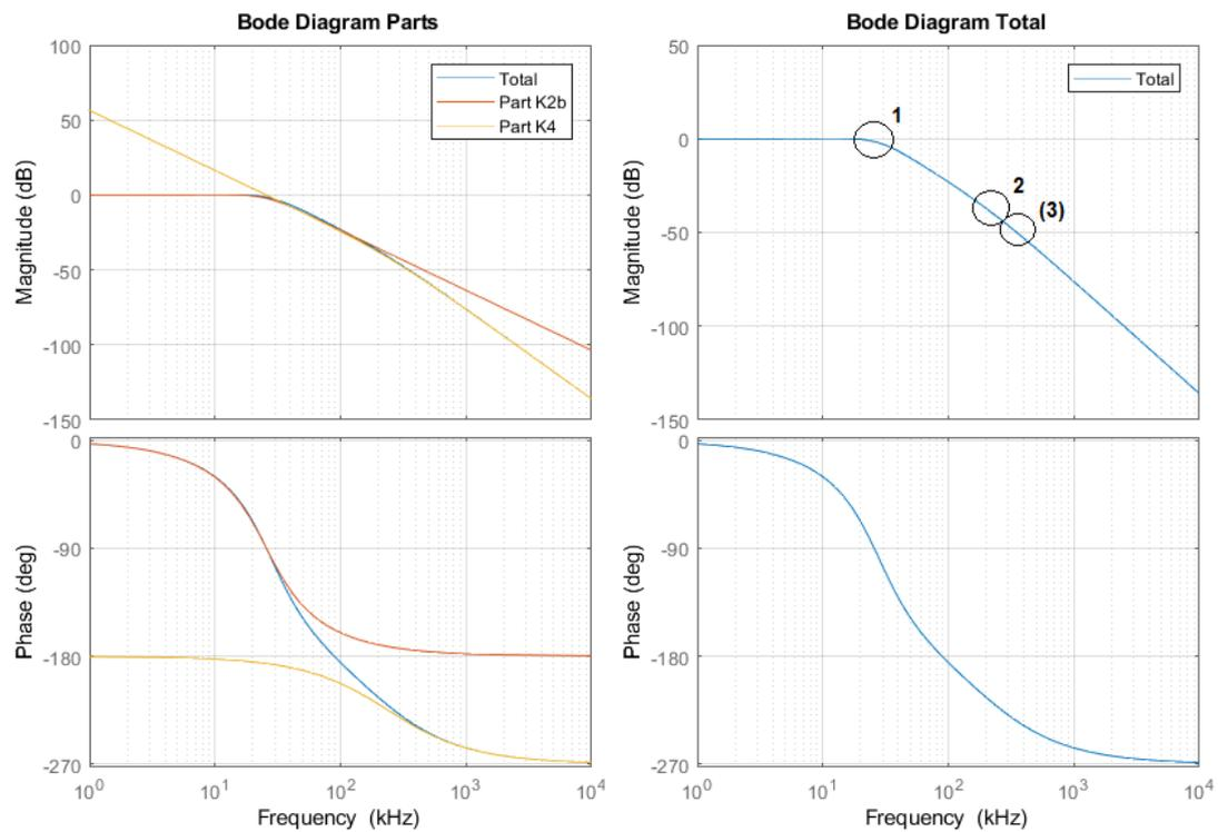
**Figure F.6:** Bode plot of final smaller transfer function of model 3.1 with a first order filter and gain  $g$  of 1
