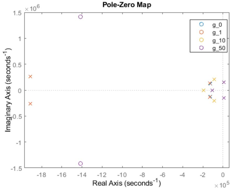
**Figure 2.11:** Zoomed in pole-zero plot of the model in Figure 2.1 with second order filter and different feedback gains 0,1,10 and 50 (represented in angular frequency)
