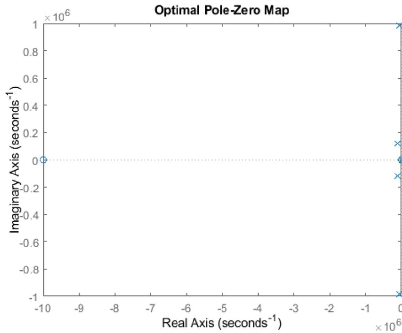
**Figure 3.12:** Optimal pole-zero plot of the model in Figure 3.1 with second order filter (represented in angular frequency)
