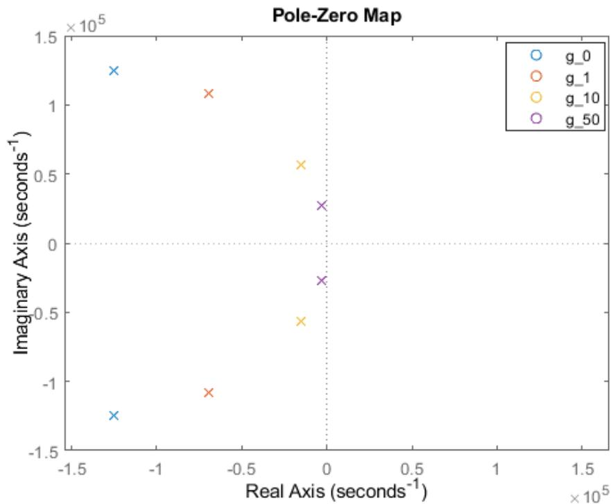
**Figure 2.4:** Zoomed in pole-zero plot of the model in Figure 2.1 with first order filter and different feedback gains 0,1,10 and 50 (represented in angular frequency)
