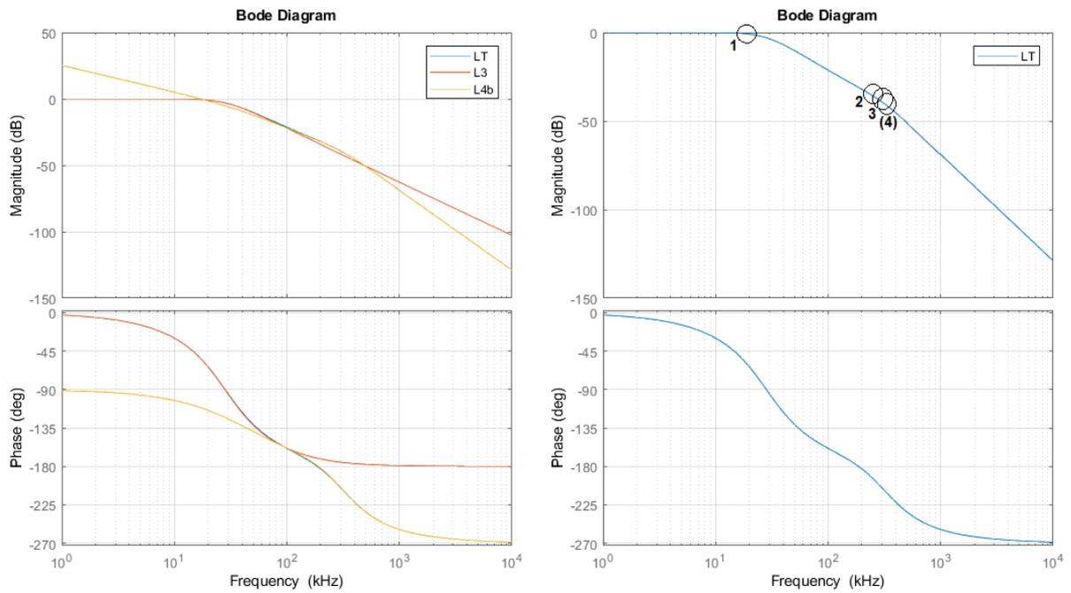
**Figure F.8:** Bode plot of final smaller transfer function of model 3.1 with a second order filter and gain  $g$  of 1
