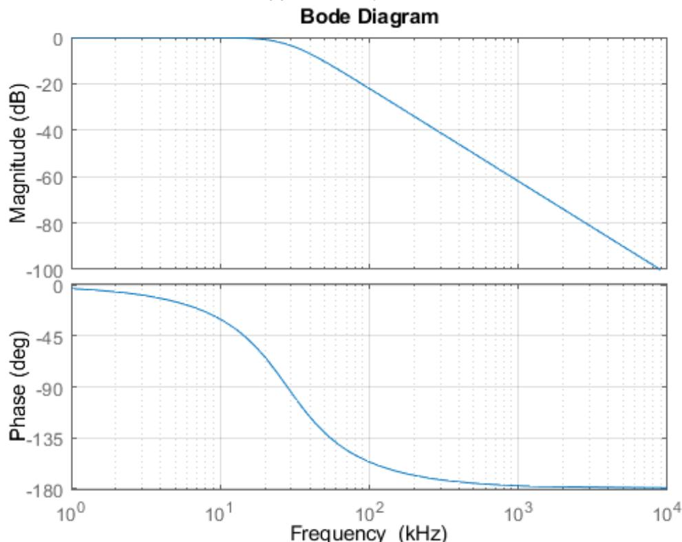
Figure 1.2: Bode plot of the transfer function of the model in Figure 1.1
