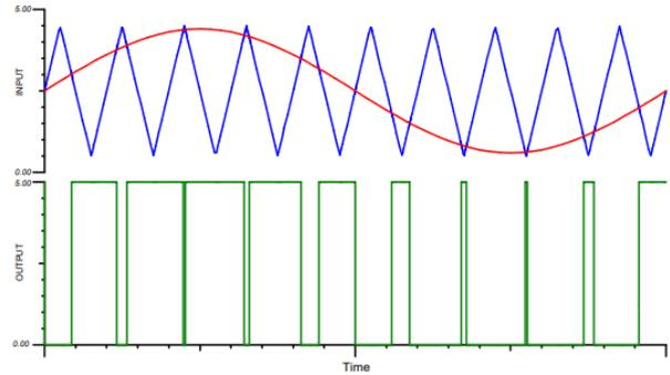
Figure E.9: How a PWM generator works shown with signals [14]
