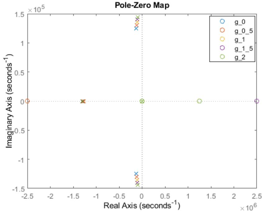
**Figure 3.3:** Pole-zero plot of the model in Figure 3.1 with first order filter and different feedback gains 0,1,10 and 50 (represented in angular frequency)
