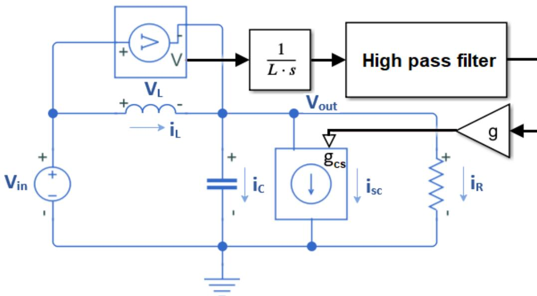
Figure 3.1: Circuit model of design with feedback from the inductor voltage
