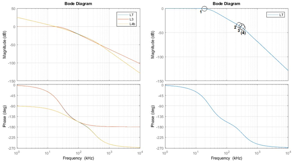
**Figure 3.10:** Bode plot of smaller transfer function which describe the transfer function of Equation 3.4(total) with a gain  $g$  of 1
