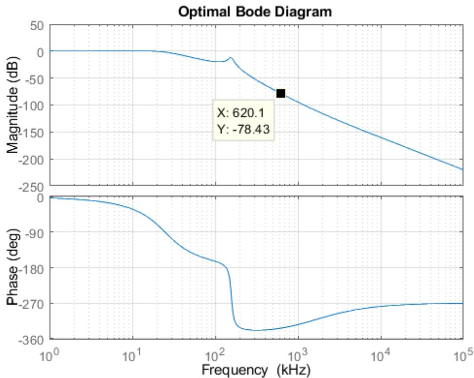
**Figure 3.11:** Optimal Bode plot of the model in Figure 3.1 with second order filter. The magnitude at 620 kHz is decreased from -53.7 dB to -78.4 dB .
