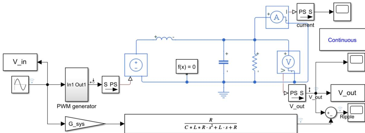
**Figure E.1:** Measured circuit model of a basic class D amplifier
