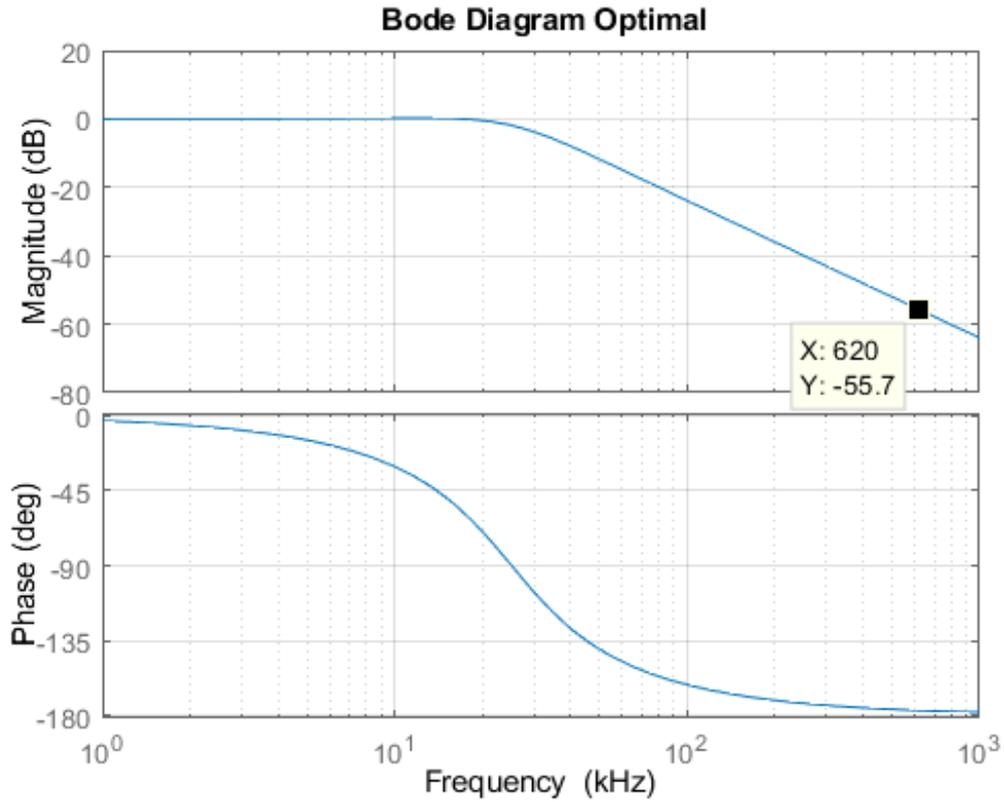
**Figure 2.6:** Optimal Bode plot of the model in Figure 2.1 with first order filter. The magnitude at 620 kHz is decreased from -53.7 dB till -55.7 dB .
