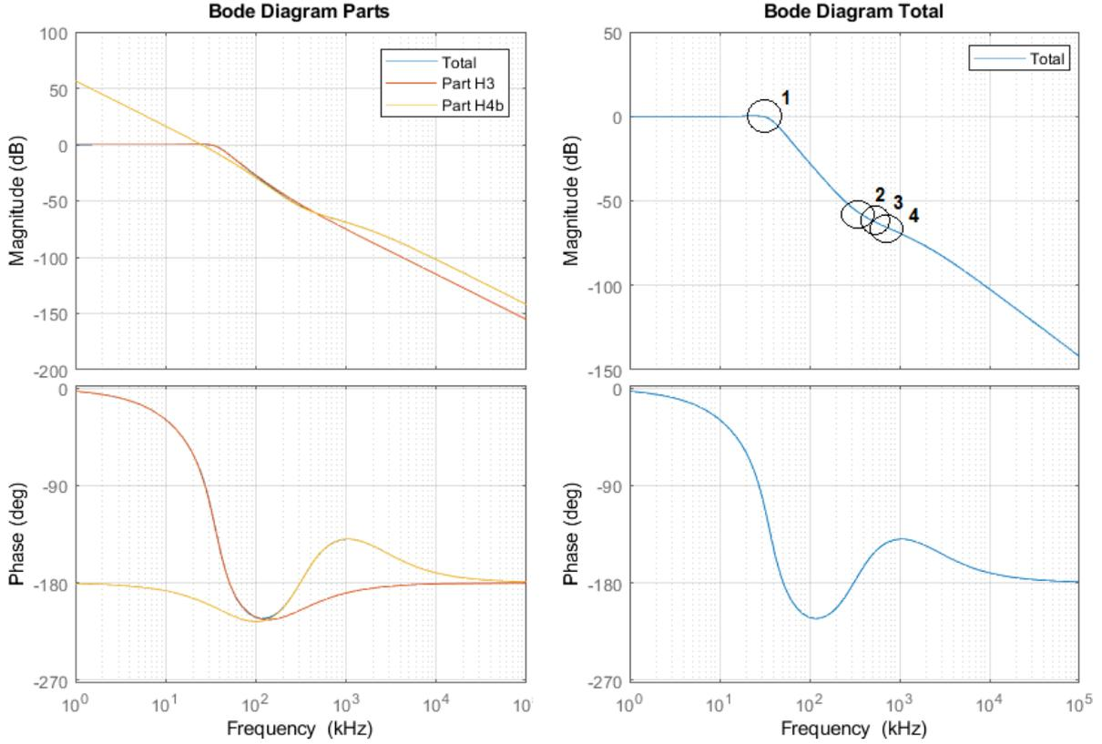
**Figure F.4:** Bode plot of final smaller transfer function of model 2.1 with a second order filter and gain  $g$  of 10
