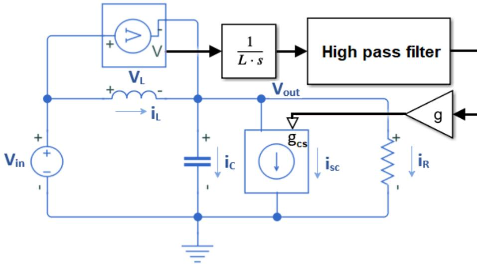
Figure D.1: Circuit model of design 4
