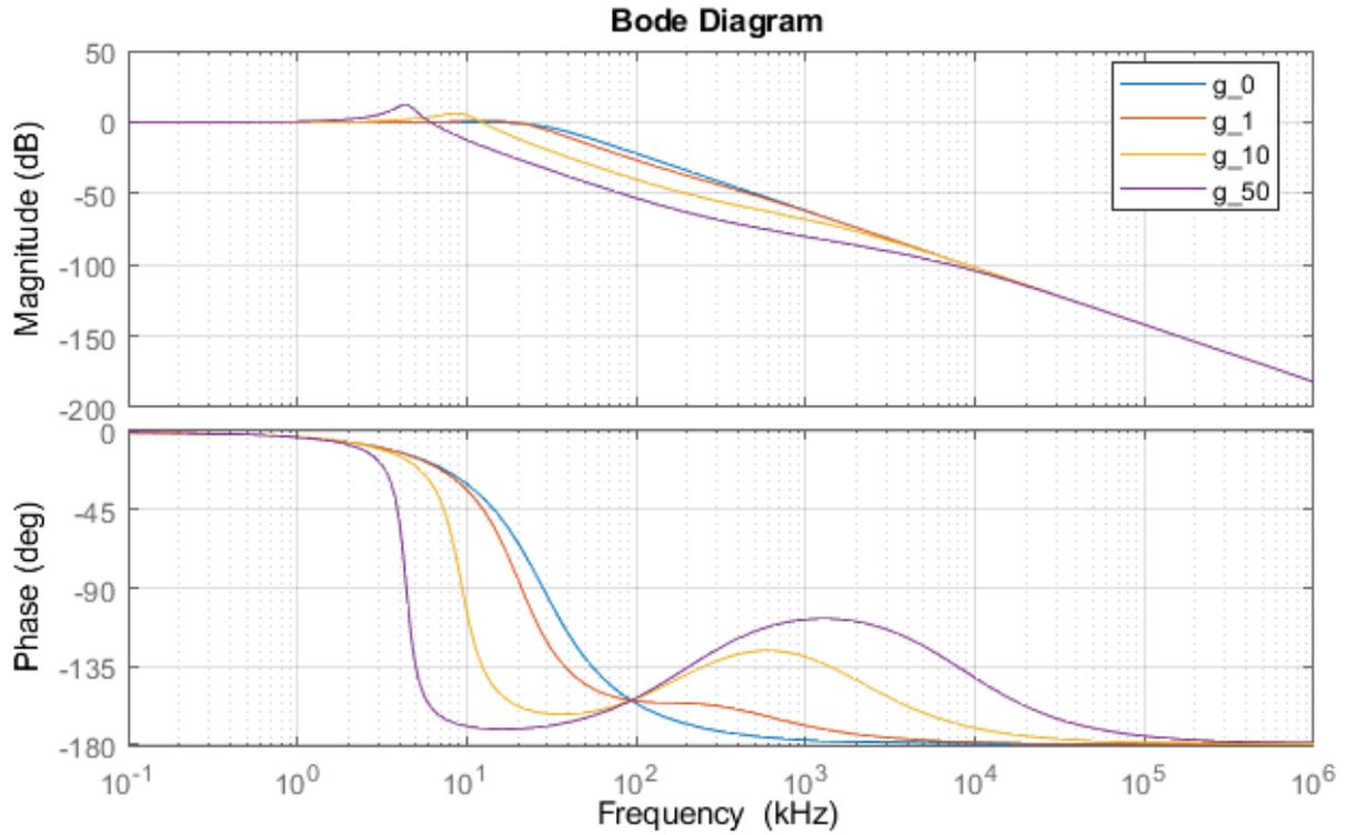
**Figure 2.2:** Bode plot of transfer function of model 2.1 with a first order filter and different feedback gains 0,1,10 and 50
