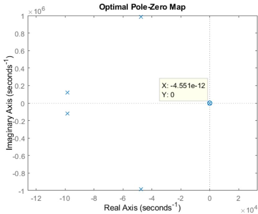
**Figure 3.13:** Optimal pole-zero plot of the model in Figure 3.1 with second order filter zoomed in (represented in angular frequency)
