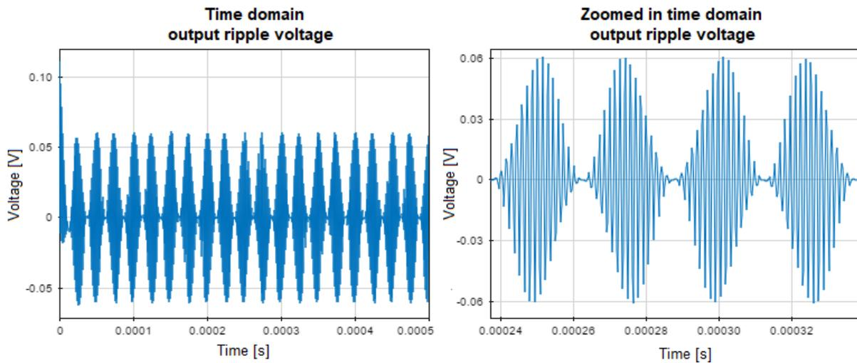
**Figure 1.4:** Time domain plot of the output ripple voltage with input frequency 20 kHz. Shows that the maximum amplitude of the output ripple voltage is 60.8 mV
