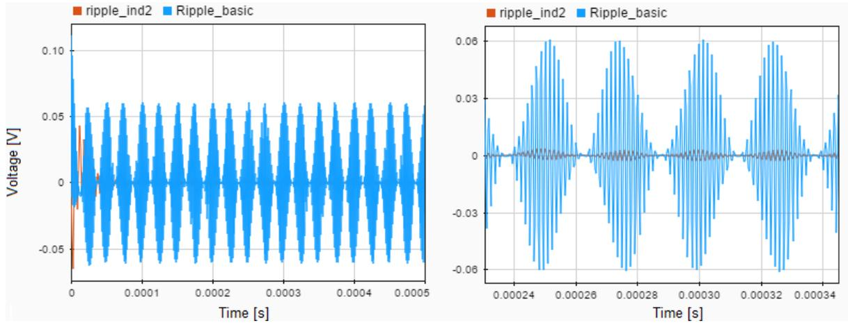
**Figure 3.14:** Optimal time domain plot of the model in Figure 3.1 with second order filter. The output voltage ripple amplitude is reduced from 60.8 mV (ripple\_basic) and 3.29 mV (ripple\_ind2)
