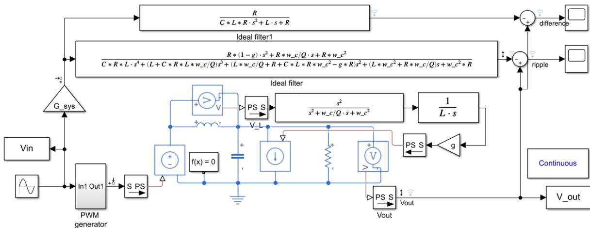
Figure E.5: Measured circuit model of second order inductor feedback
