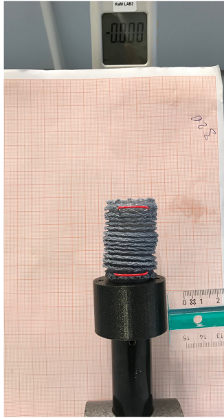
Figure 4.2: The calibration experimental set-up including the soft actuator module, scale (ruler), and pressure read-out.
