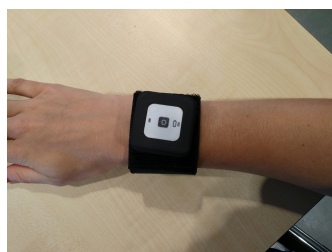
Figure 4.3: Placement of 2M motion logger with wristband on right wrist.
