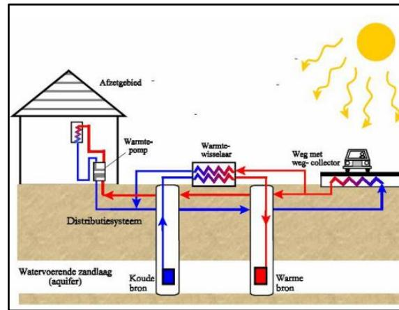
Figure 6: Visualization of heat- and cold transport
