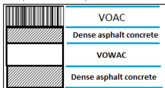
Figure 5: Cross-section asphalt construction with VOWAC-collector
