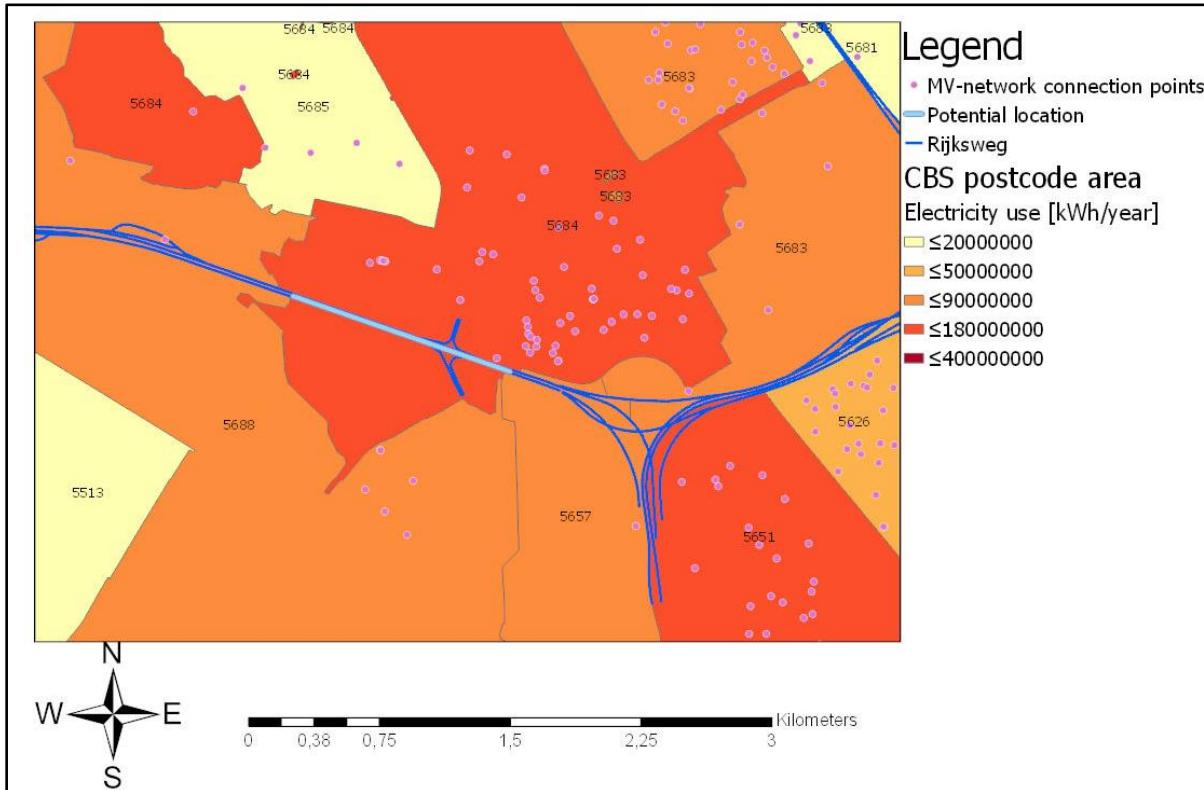
Figure 17: Potential location for the solar road
