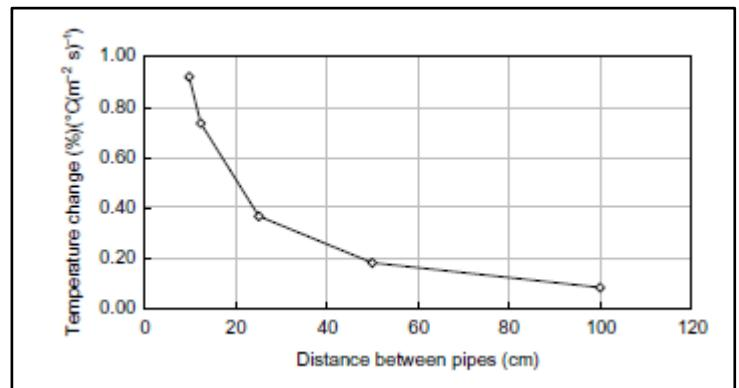
Figure 7: Effect of different distance between pipes on temperature change rate (Wang, Wu, Chen, & Zhang, 2010)
