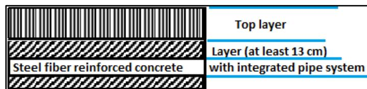
Figure 3: Cross-section asphalt construction with PIC-collector
