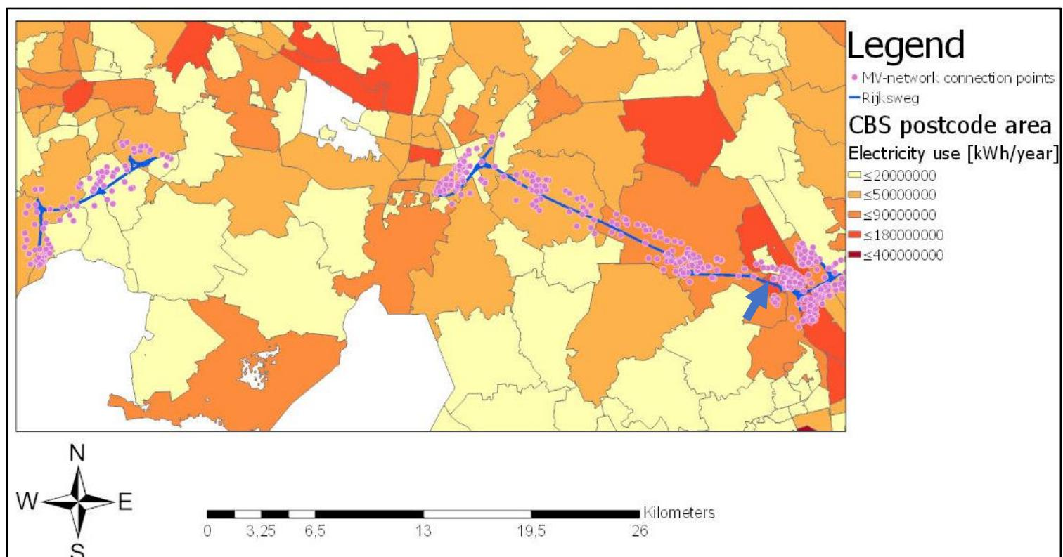
Figure 16: Electricity use and mv-network connection points around the study area
