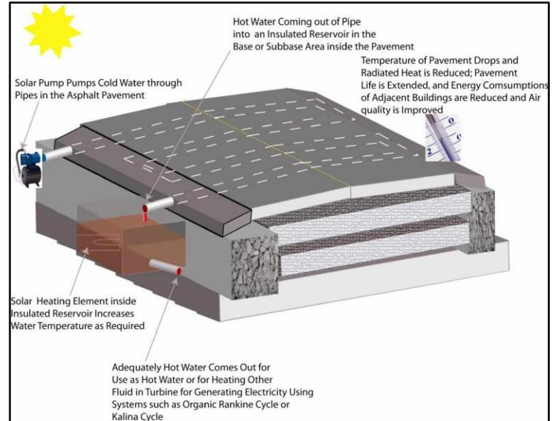
Figure 2: The structure of the asphalt collector with a pipe system (Todd, 2011)
