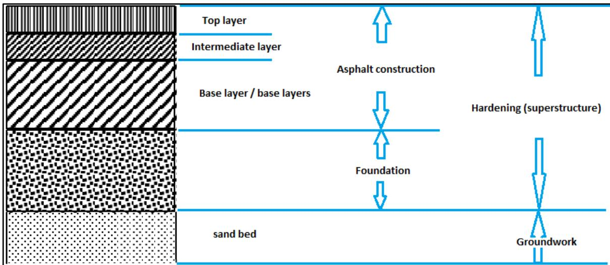
Figure 11: Cross-section of a standard asphalt construction (Erkens, 2015)
