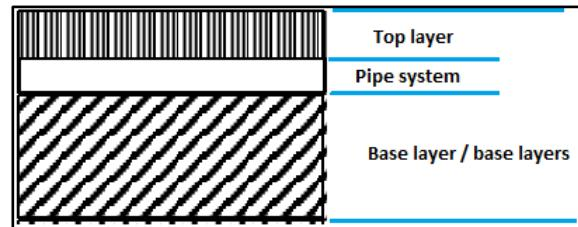
Figure 4: Cross-section asphalt construction with PIA-collector
