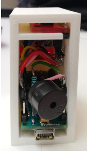
Figure 5.9. Electronic circuit placed in the casing of the prototype, shown from the front.
