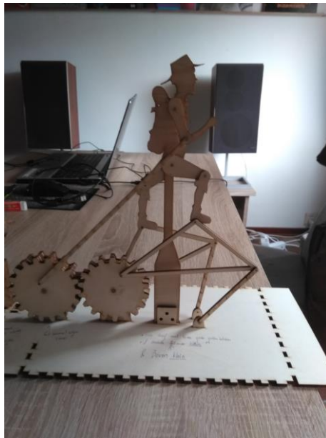
Figure 6.2.1 – First automata with leg bending the wrong way
