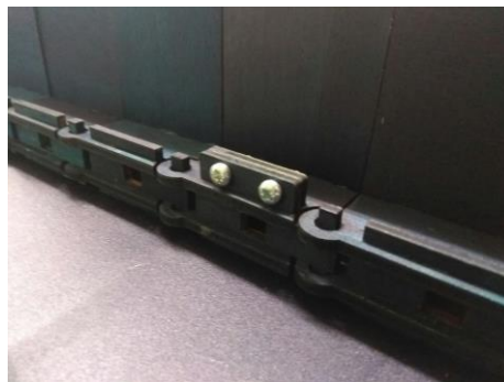
Figure 5.1.2 – Detaching mechanism that was added in a third iteration
