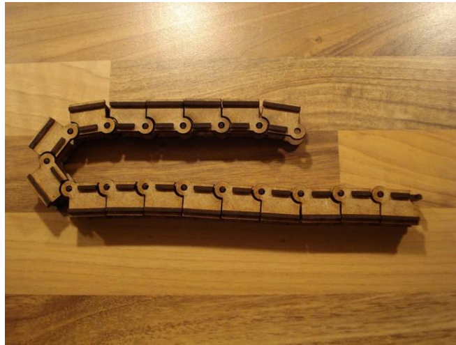
Figure 4.3.2.1 – Lasercut chain design by Msraynsford published on Thingiverse
