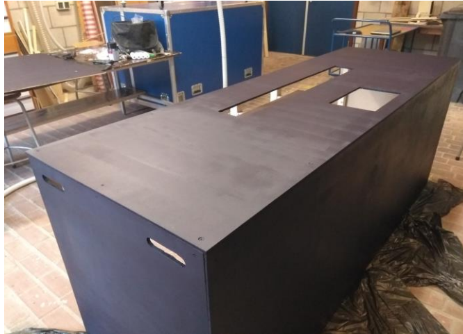
Figure 6.1.5 – Casing painted with three layers of acrylic paint
