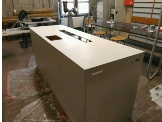
Figure 6.1.3 – Case painted with two layers of primer
