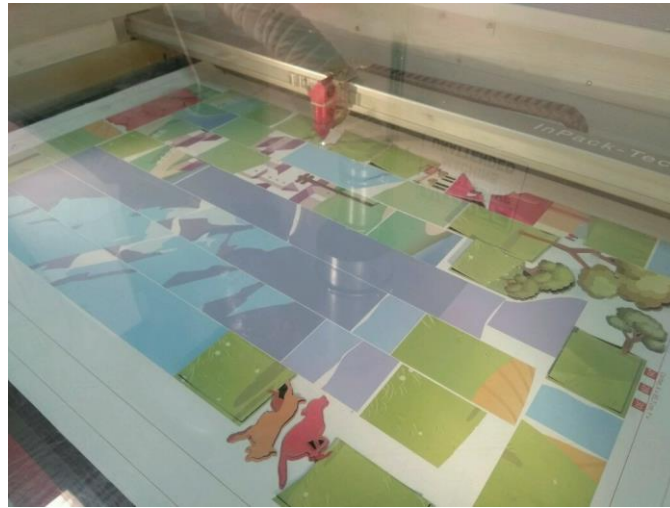
Figure 6.3.5.3 – One of the canvas sheets in the process of being cut out
