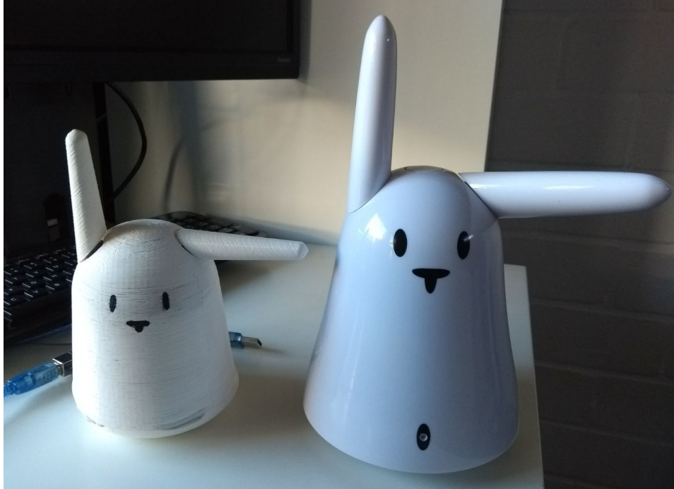
Figure 5.6: The 3D printed model of the prototype (left) next to the original Nabaztag (right).
