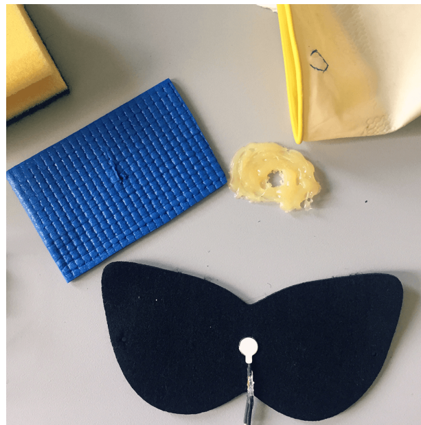
Figure III.14: Vibration dispersing felt
