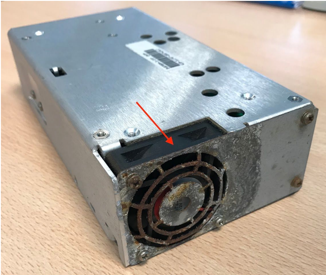
Fig. 7: Corroded power supply, TDK-Lambda sws300A-3/c02
