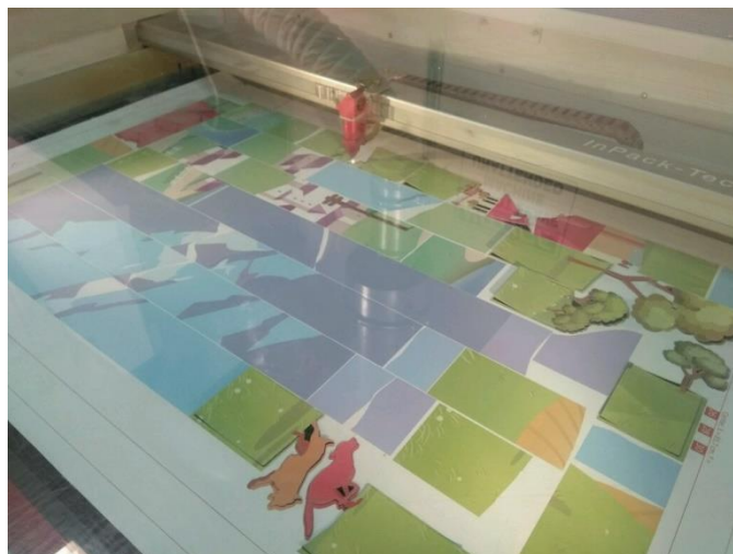
Figure 5.1.2.5- Lasercutter cutting the prints
