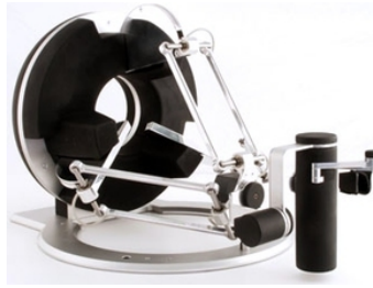
Figure 3.2: Omega.7 haptic device. From ForceDimension (2018).
