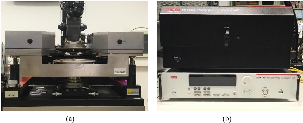
Fig. 3.2. The photo of PM 300 probe station (a), Keithley 8010 (b) on the top, and Keithley 2657A (b) at the bottom.
