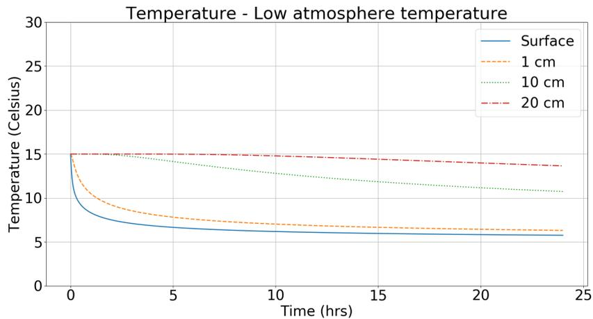
Figure 9: Temperature distribution in case there is no slab on top with an atmosphere temperature of -50 degrees Celsius.
