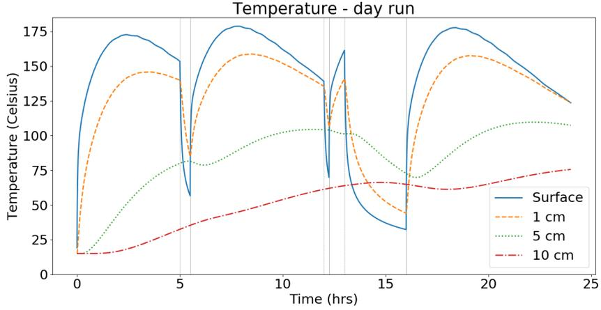
Figure 11: Heat spread in the ground as a result of hot slabs that are put onto the ground, cool down and are removed again. The used data for the surface temperatures of slabs has been obtained using another model that is available at Tata-Steel.
