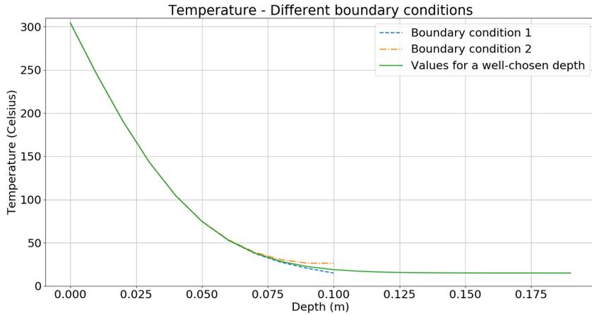
Figure 4: Surface temperature two hours after a slab with a constant temperature of 600 degrees Celsius arrives. Two different boundary conditions are used to simulate. In two cases, the bottom node is not chosen deep enough, in the third case it is.
