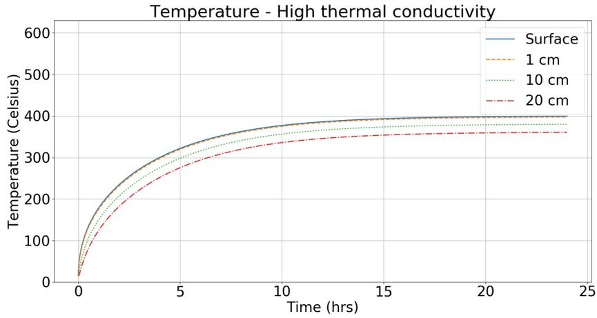
Figure 6: Temperature distribution with a thermal conductivity of  $100 \text{ W}\cdot\text{m}^{-1}\cdot\text{K}^{-1}$  and a slab with a constant temperature of 600 degrees Celsius on top.
