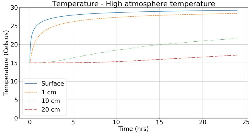
Figure 10: Temperature distribution in case there is no slab on top with an atmosphere temperature of 50 degrees Celsius.
