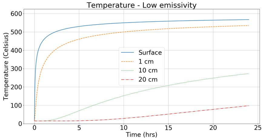
Figure 7: Temperature distribution with an emissivity factor of 1 and a slab with a constant temperature of 600 degrees Celsius on top.
