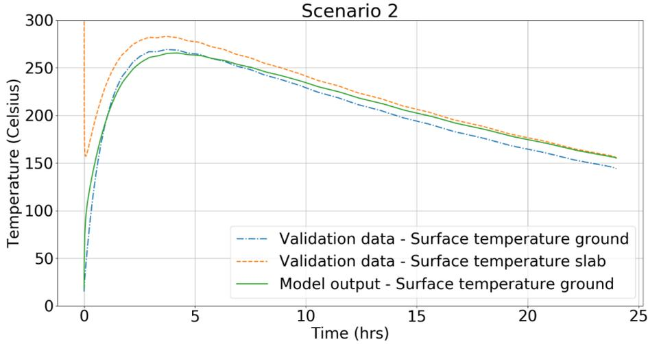
Figure 14: Model output for scenario 2, in which a stack of six slabs with an initial temperature of 600 degrees Celsius lays on top of the ground and cools down. The data is provided by a model at Tata-Steel.
