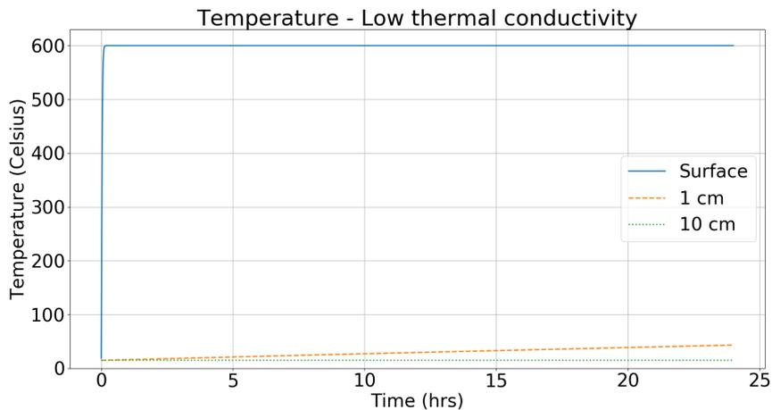
Figure 5: Temperature distribution with a thermal conductivity of  $0.0001 \text{ W}\cdot\text{m}^{-1}\cdot\text{K}^{-1}$  and a slab with a constant temperature of 600 degrees Celsius on top.
