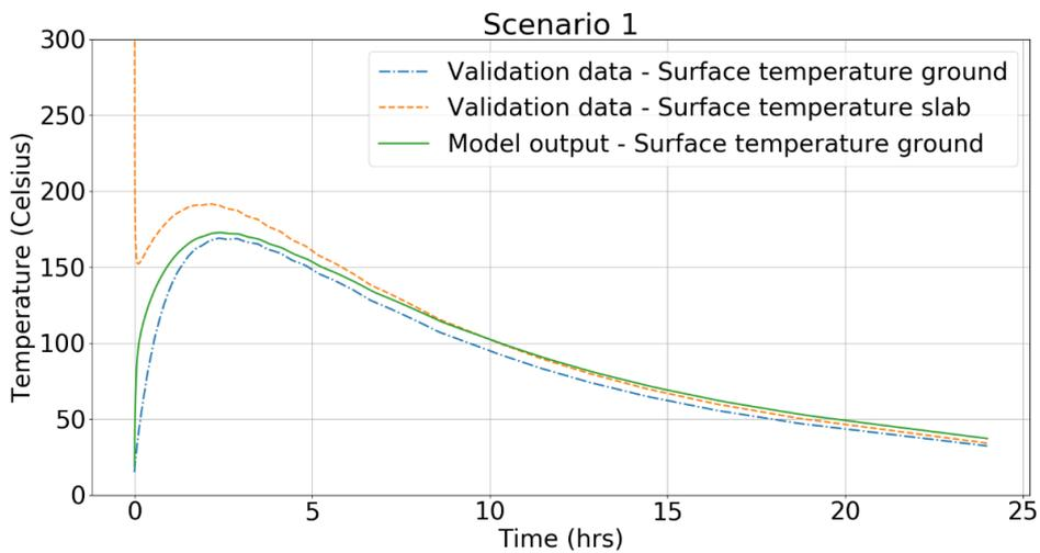
Figure 13: Model output for scenario 1, in which one single slab with an initial temperature of 600 degrees Celsius lays on top of the ground and cools down. The data is provided by a model at Tata-Steel.
