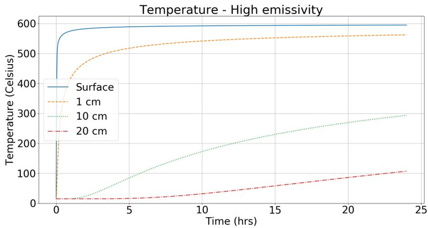
Figure 8: Temperature distribution with an emissivity factor of 0.0001 and a slab with a constant temperature of 600 degrees Celsius on top.
