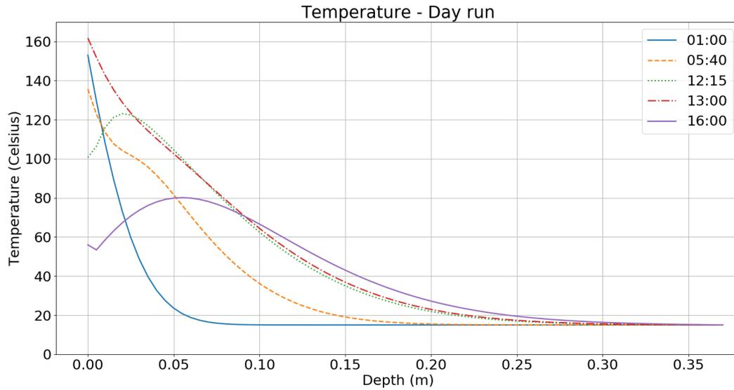
Figure 15: Heat spread in the ground as a result of hot slabs that are put onto the ground, cool down and are removed again. The used data for the surface temperatures of slabs has been obtained using another model that is available at Tata-Steel.
