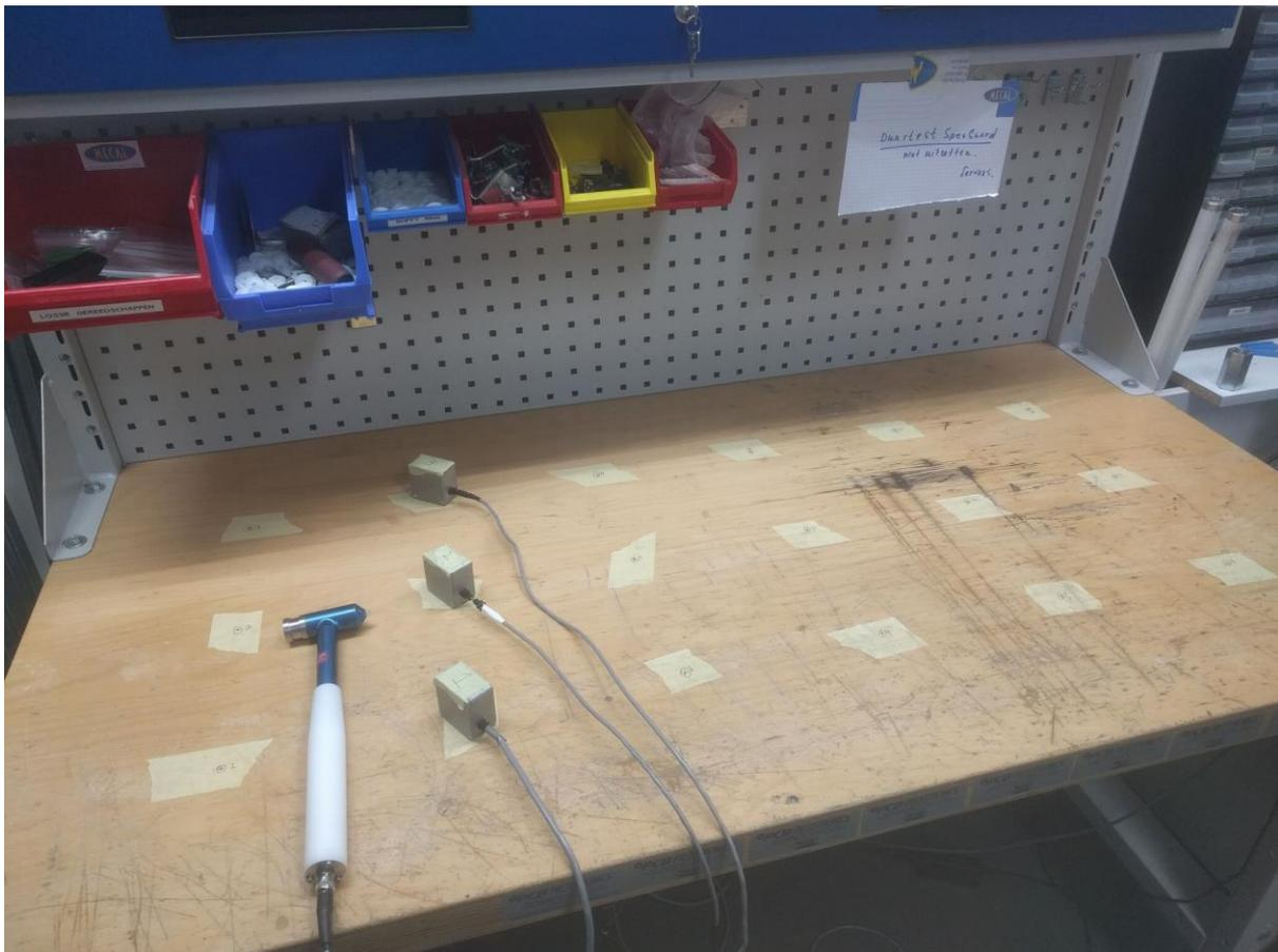
Figure 13: Test case table with SpecTest hammer and sensors
