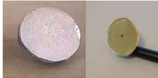
Figure 21: Proposed electrode model on the left, remade electrode on the right
