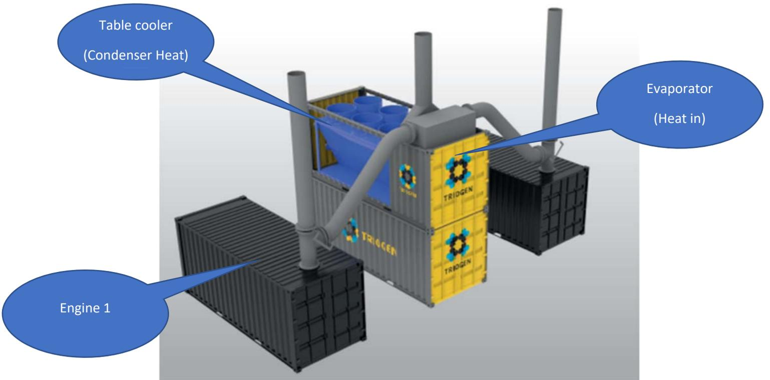
Figure 2.3: Proposed setup of the Tri-O-Gen E-box and t-box
