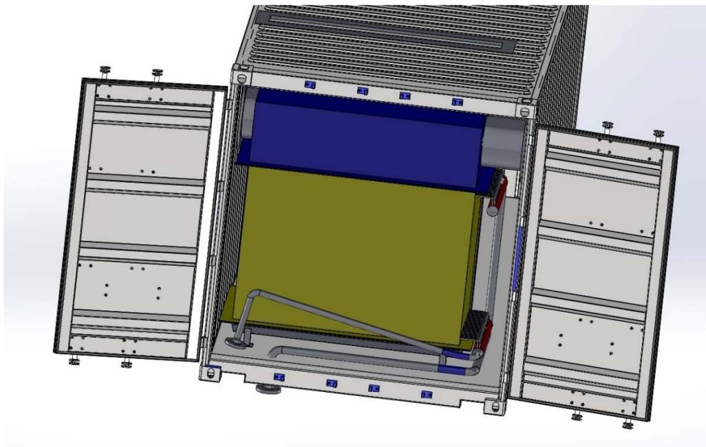
Figure 11.1: Toluene piping in transport state (L) and operation (R)
