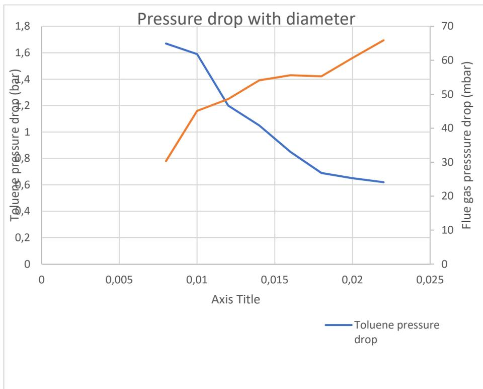
Figure D.2: Toluene and flue gas pressure drop for constant flue gas inlet area
