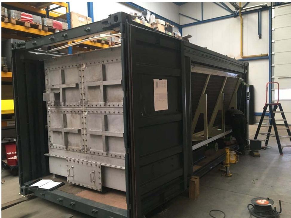
Figure C.2: Reference design without insulation in the container.
