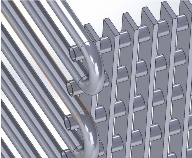
*Figure 12.1: Possible support structure*
