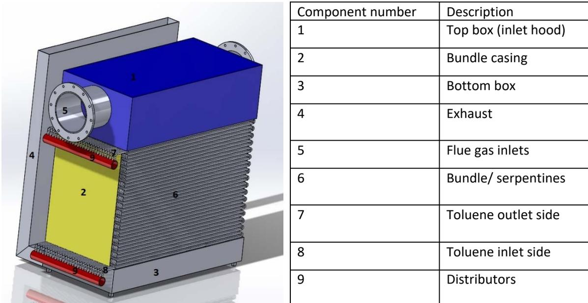
Figure F.1: Global evaporator layout and component naming
