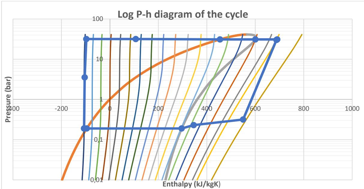
Figure A.1: log P-h diagram of the Organic Rankine cycle. Working fluid: toluene
