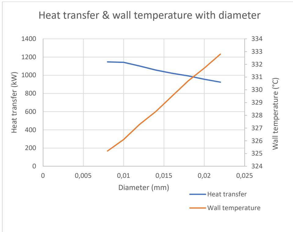
Figure D.1: Heat transfer and wall temperature for constant flue gas inlet area
