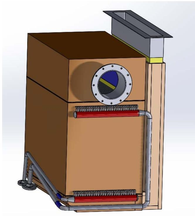
*Figure F.4: Final design with insulation. The piping is shown in transport state to demonstrate that the flanges fit next to the insulation*
