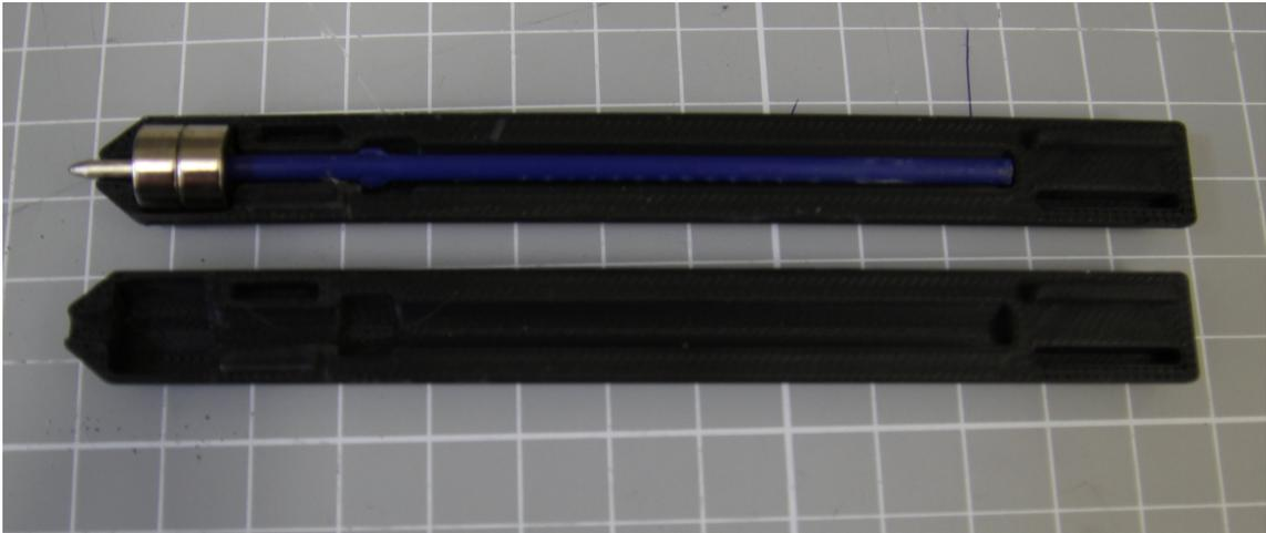
Figure 9.3: Inside of the designed pen.
