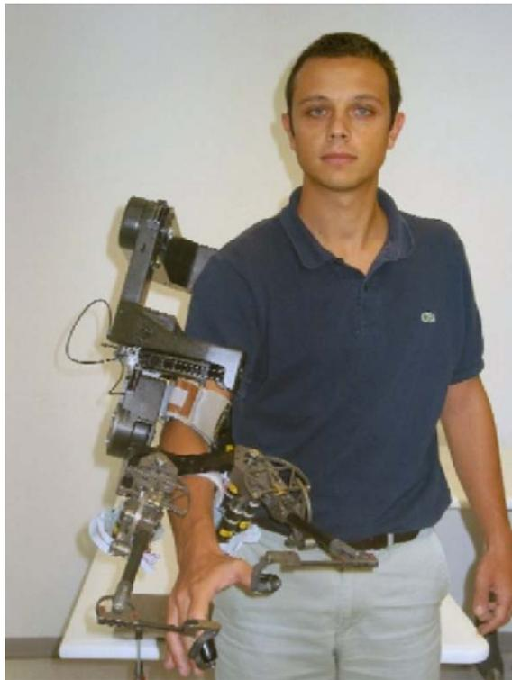
Figure 1.2: Example of an exoskeleton for rehabilitation [15].
