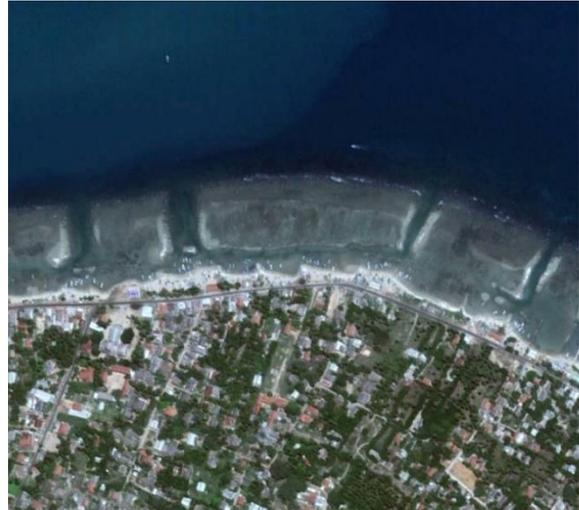
Figure 8: Sandy coastline influenced by the construction of a series of small jetties and positioned behind interrupted reefs at Point Pedro (Google Earth).
