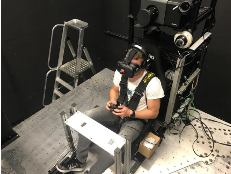
Figure 2. The setup of the experiment. The participant is placed on the motion platform while wearing an HMD, noise cancelling headphones and giving inputs using the handheld controller.
