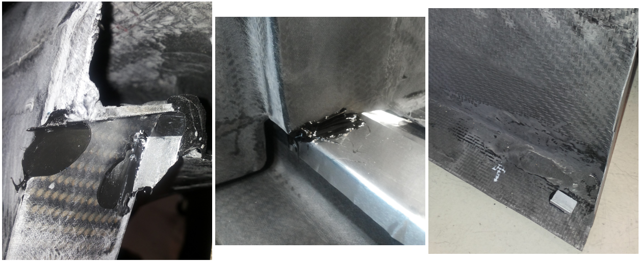
Figure 5.2: From left to right: Rear panel with glue attached to define the height and movement in horizontal plane. Second, an example of glue between the scuttle and aluminum tape on the chassis. This glue shim will define height. Last, out of experience from the assembly employees, an extra fixation in the form of an aluminum corner piece, was needed to withstand the panel from being mounted too far inwards.
