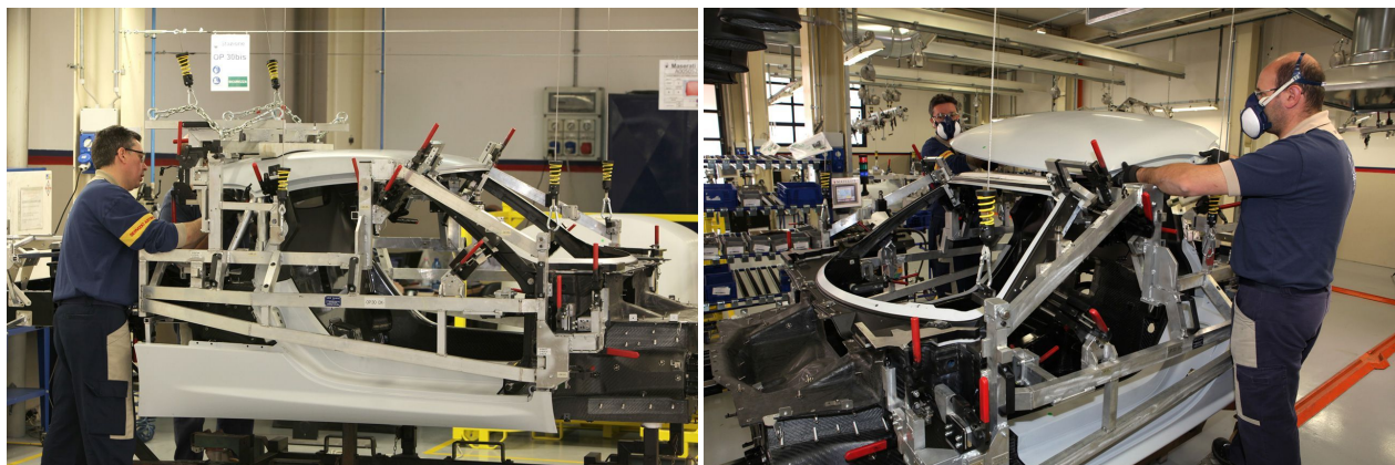
Figure B.5: Used jig during adhesion fase by Alfa Romeo [4] [5].
