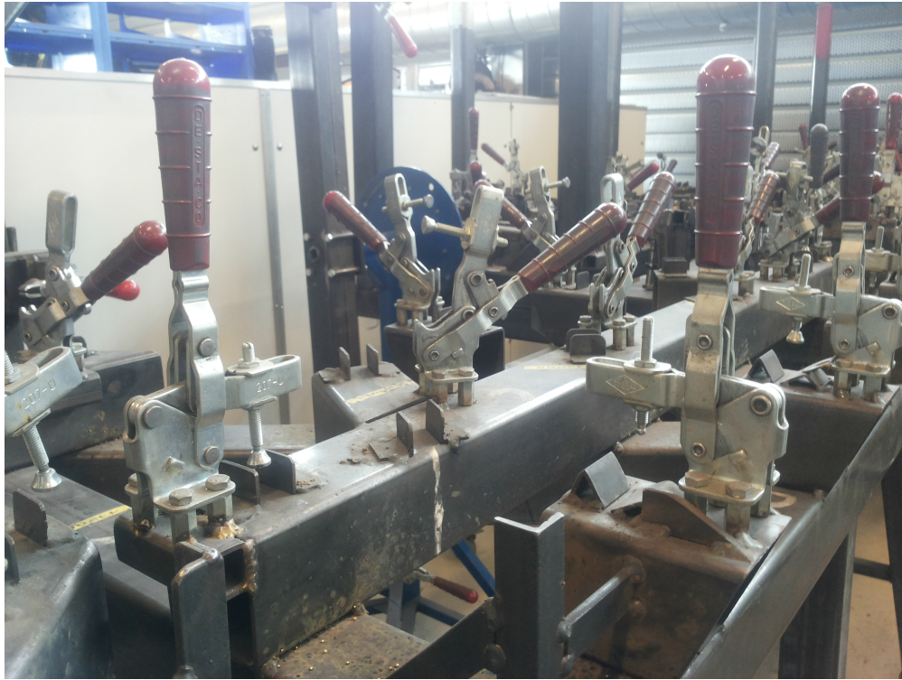
Figure 2.2: Welding jig for a section of the Donkervoort chassis.
