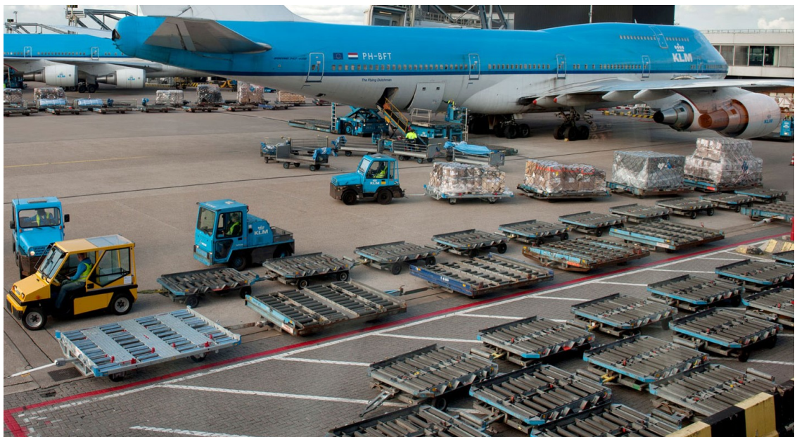
Figure 2: Ground Support Equipment at Schiphol with powered vehicles and unpowered carts [14]
