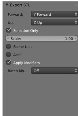
Figure 3.20: The setup of exporting the object as an `.stl` file.
