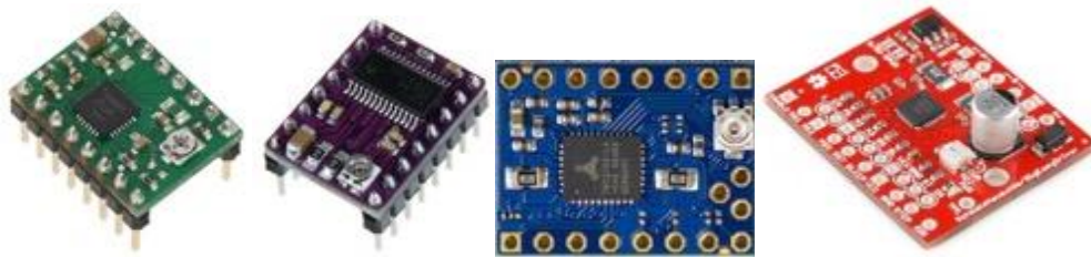
Figure 5-18: Stepper driver options from left to right; Polulu, Stickstep, Trinamic, Adafruit Big Easy driver
