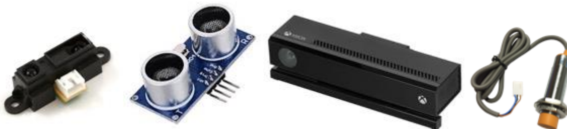
Figure 5-7: Distance sensor options, from left to right; Sharp IR, Ultrasonic, Microsoft Kinect, capacitive
