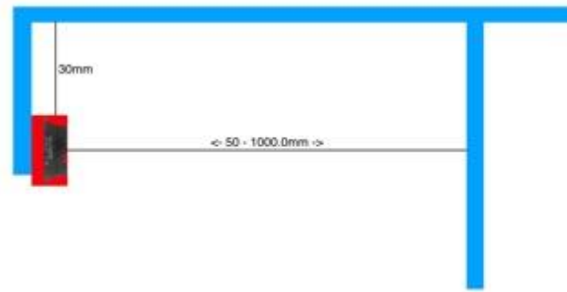
Figure 5-8: Sharp IR test setup schematic
