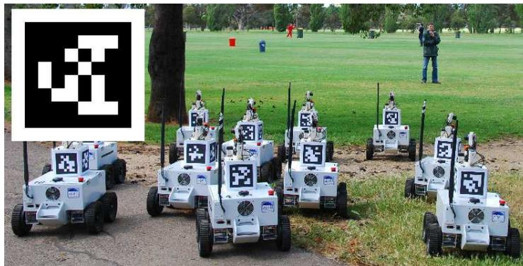
**Figure 2.12:** AprilTag markers for navigation of mobile robots (26)
