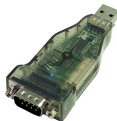
**Figure 3.3:** USB2Dynamixel: device which directly connects DYNAMIXEL motors to PC USB port (29)
