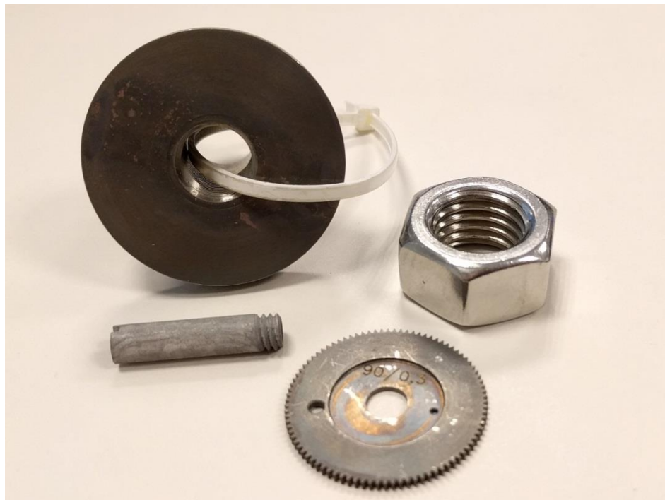
Figure 2. Examples of flash attack on stainless steel parts, compared to an A2 (~304) stainless steel nut.
