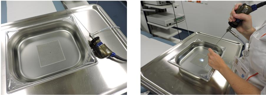
(a) Calibration plate inside metal container. (b) Overview of the calibration setup.
