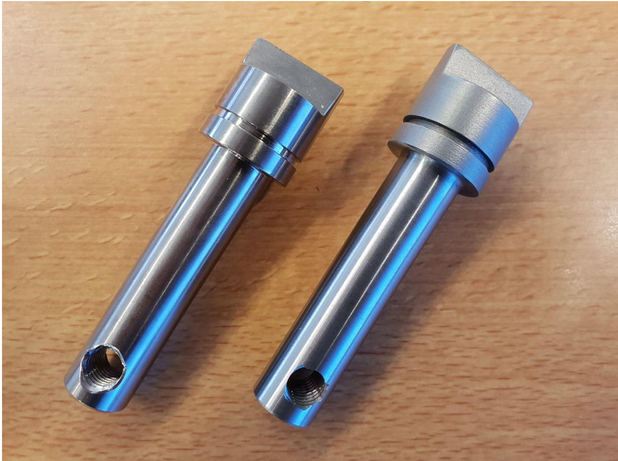
Figure X2: The original locking pin (left) and the printed locking pin (right)
