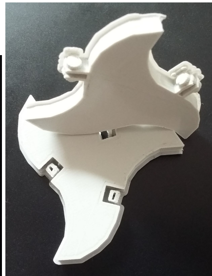
Left: Figure 18, properly aligned and well fitting hinges. Right: Figure 19, movement along the axis is possible
