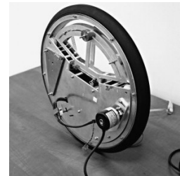
Figure 2.2.: Self-stabilizing monowheel robot prototype. [9]
