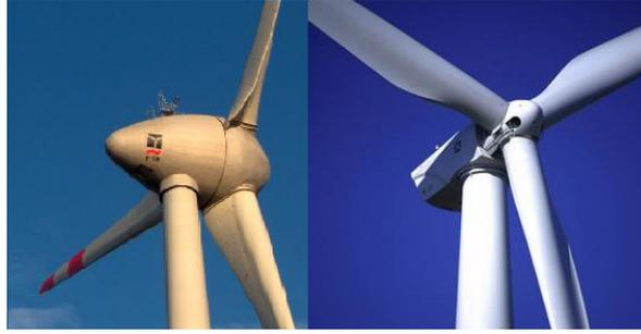
**Figure 3.24:** The hub designs in Enercon (left) and GE (right) blades [7].
