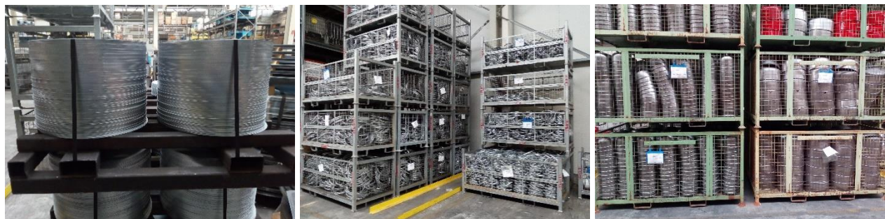
Figure 18: WIP; from left to right: discs, clamping rings and vessel halves
