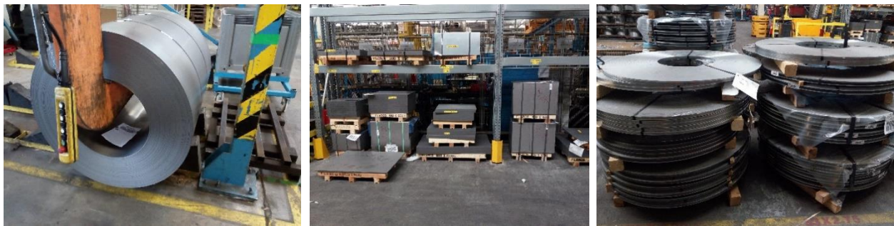
Figure 17: Raw materials; from left to right: steel for discs, mantles and clamping rings
