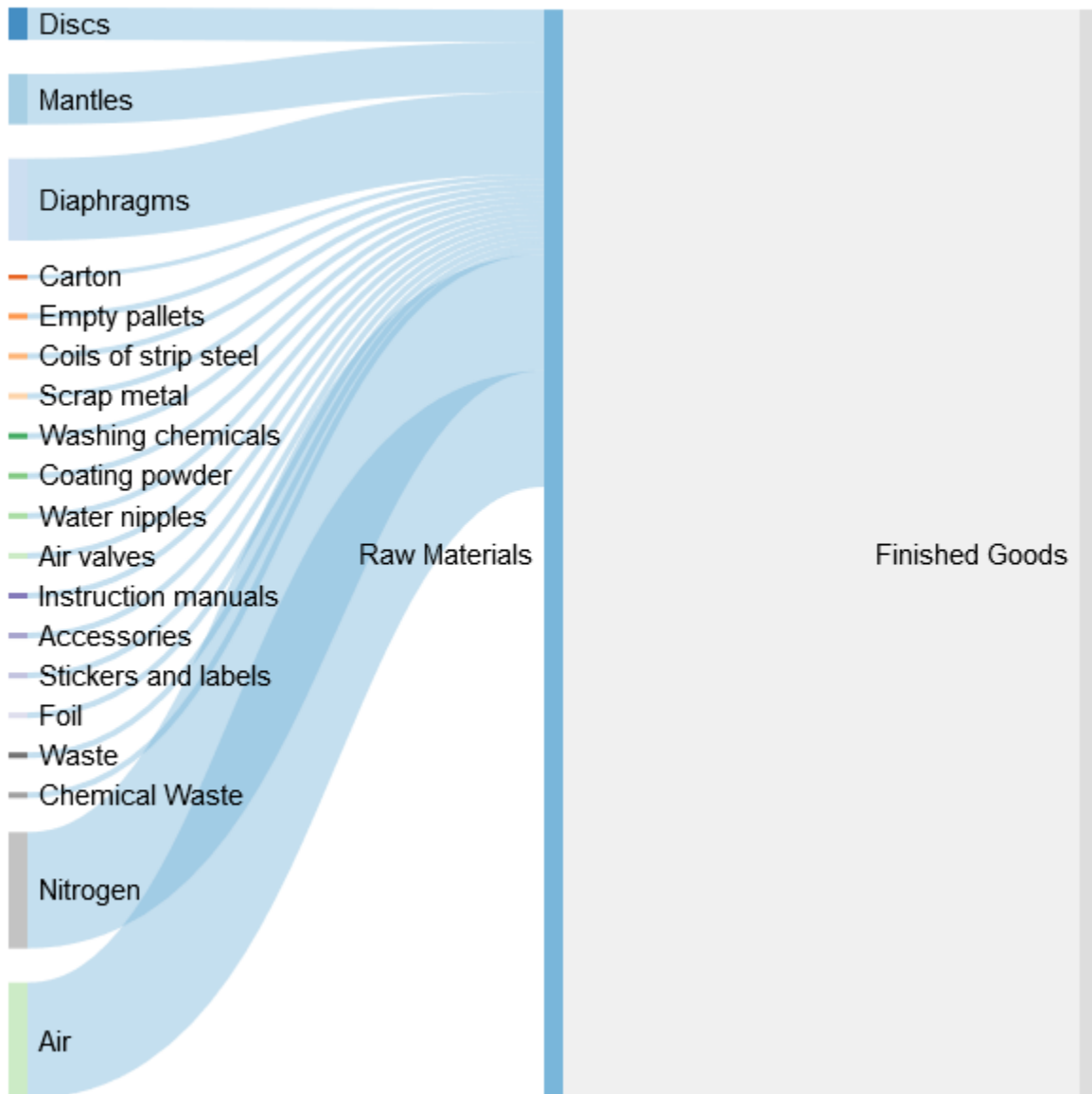
Figure 51: Sankey diagram MGV (current situation)
