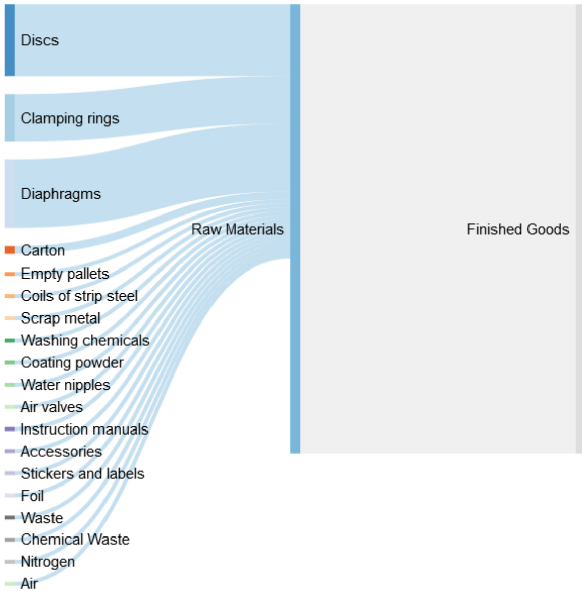
Figure 52: Sankey diagram OEM (current situation)
