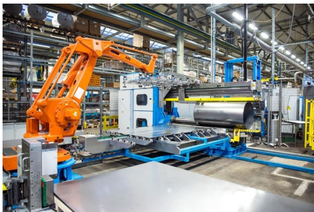
Figure 11: Impression of the Middelgrote vaten lijn (MGV); a) rolling mantles, and b) coating
