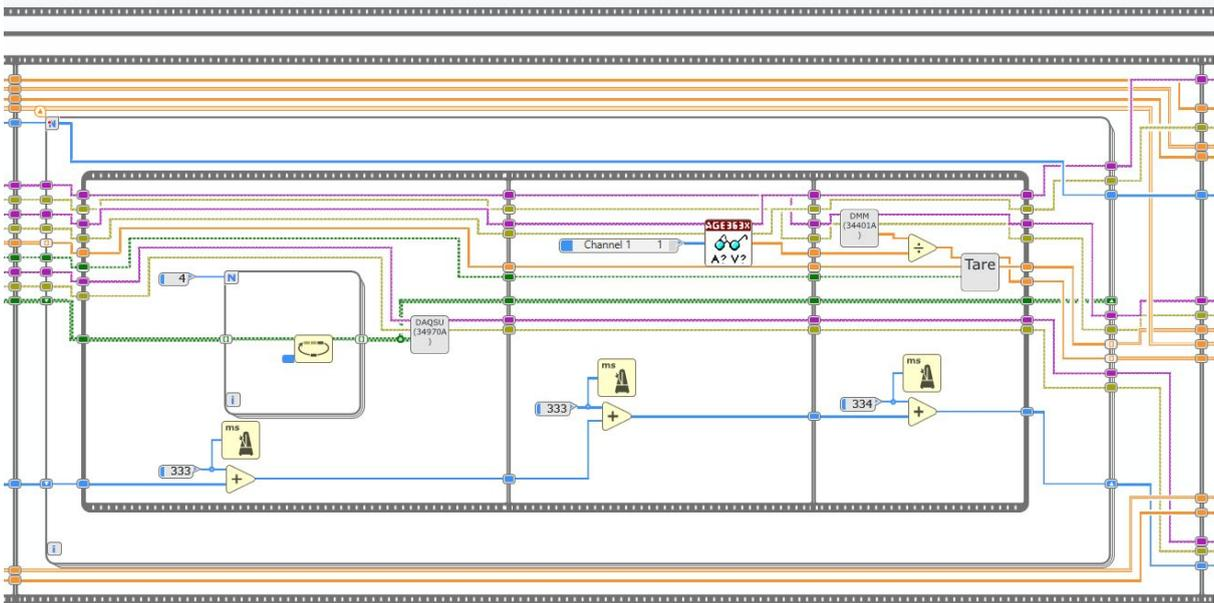
Chip measurement (switch to correct channel - read out the excitation voltage - read out chip with DMM)
