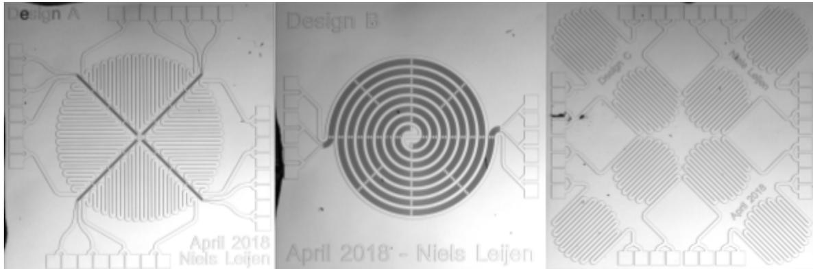
Figures 9, 10, and 11, fabricated chip designs A, B, and C (not yet bond wired)
