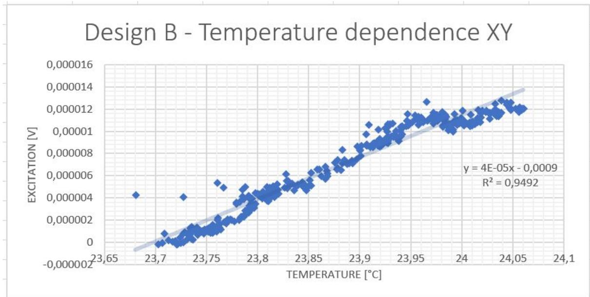
Figure 23, Temperature vs average excitation design B with linear trend line using the first 400 samples
