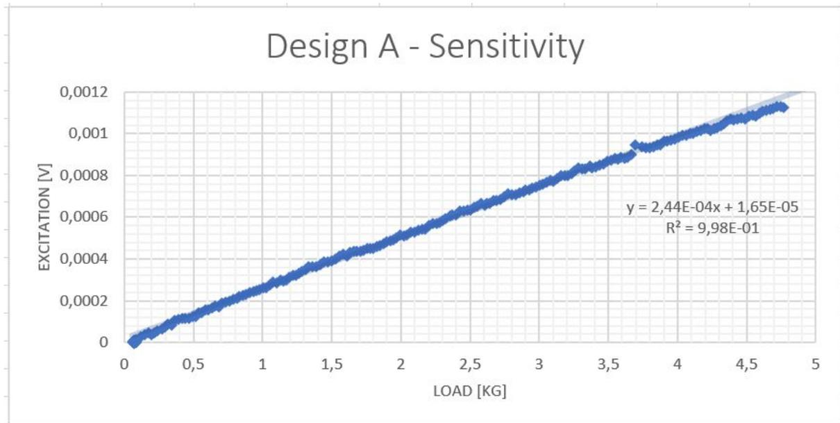
Figure 38, Sensitivity plot of design A with a loose pushing block during linear loading
