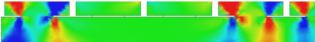
Figure 4, FEM simulation of the shear stresses of figure 3, where the green color is zero shear and the red and blue colors are  $4E1 \text{ N/mm}^2$  [MPa] of shear in the positive and negative  $z$  direction in the  $xz$  plane
