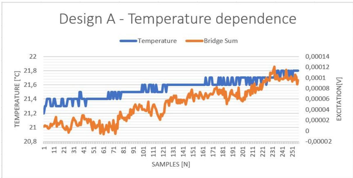
Figure 19, Temperature measurement result design A in test setup 1 with a sample time of 1/30Hz
