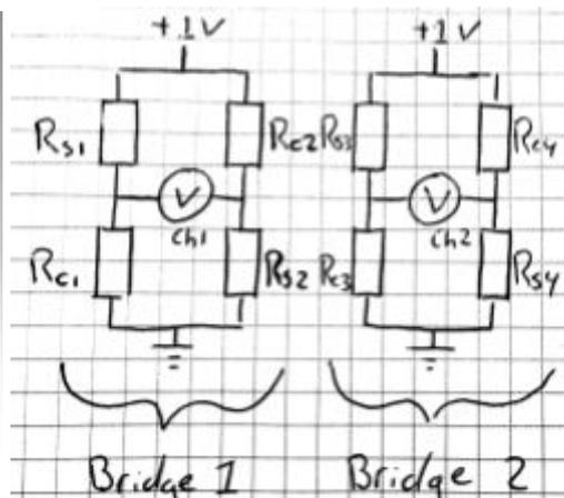
Figure 16, Connection schematic design A in Wheatstone bridge configuration
