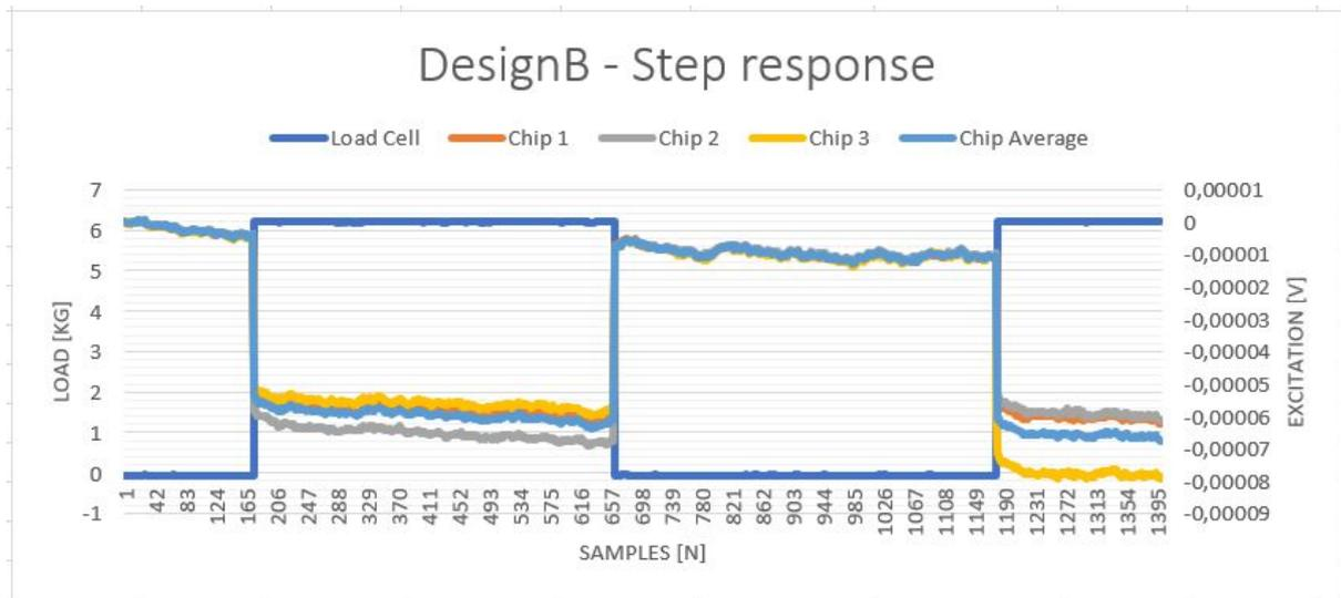
Figure 28, Step response measurement design B with a sample time of 2/9Hz
