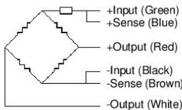
The two "sense" wires sample the bridge supply voltage at the load cell. Complete compensation of change in the lead wire resistance, due to temperature change and/or cable extension, is achieved by feeding this voltage into appropriate electronics.
