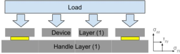
Figure 3, Tested device with one SOI wafer (1) with suspended reference gauges to prevent strain and a reference axis (not to scale)
