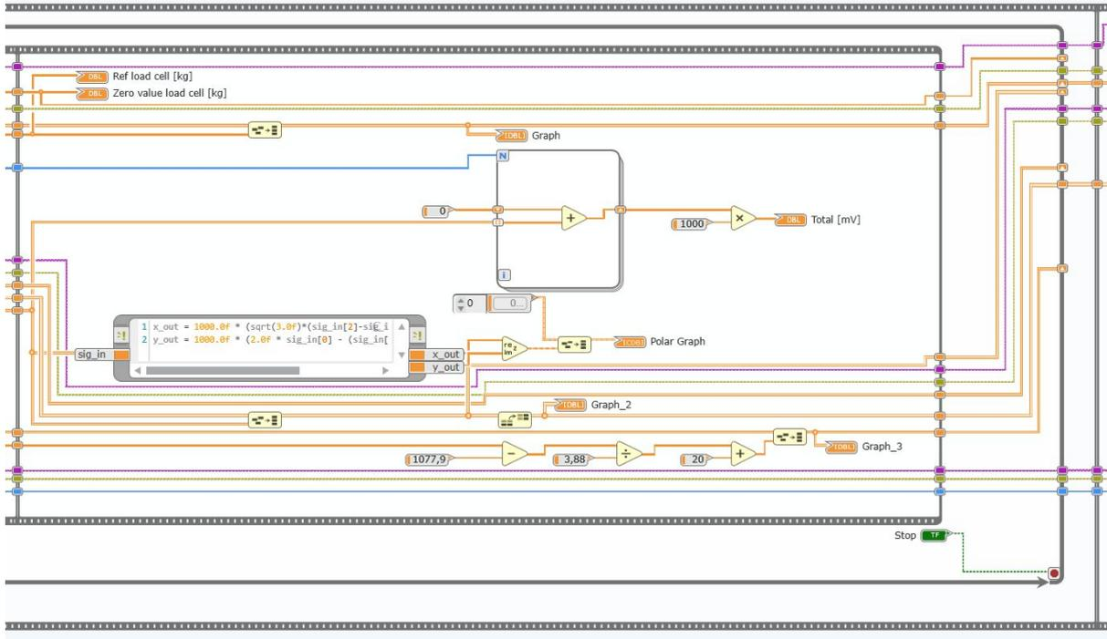
Data visualization step (puts all previously collected data in an array and/or do some calculations with previously collected data in order to visualize it)
