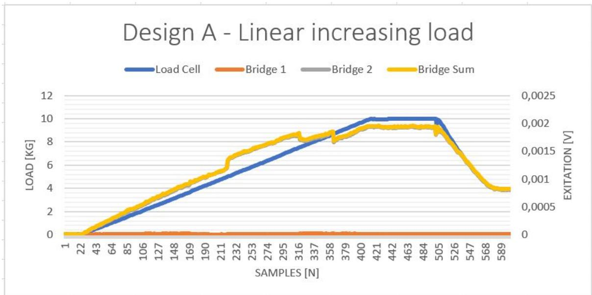
Figure 34, Linear response measurement of design A with a loose pushing block the sample rate is 1/3Hz
