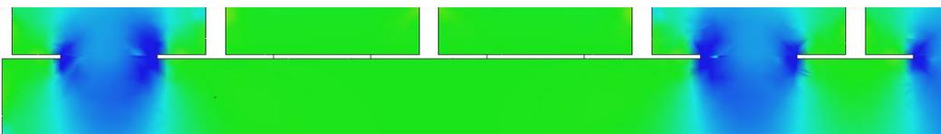
Figure 5, FEM simulation of the normal stresses of figure 3, where green is zero stress and the blue color is  $2E2 \text{ N/mm}^2$  [MPa] of stress in the negative  $z$  direction
