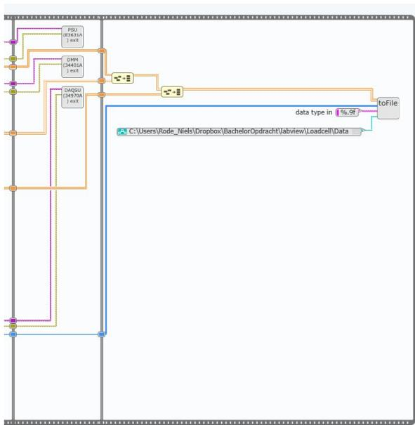
Exit step (when the stop function is called; terminate connections with measurement equipment - save collected data to file)
