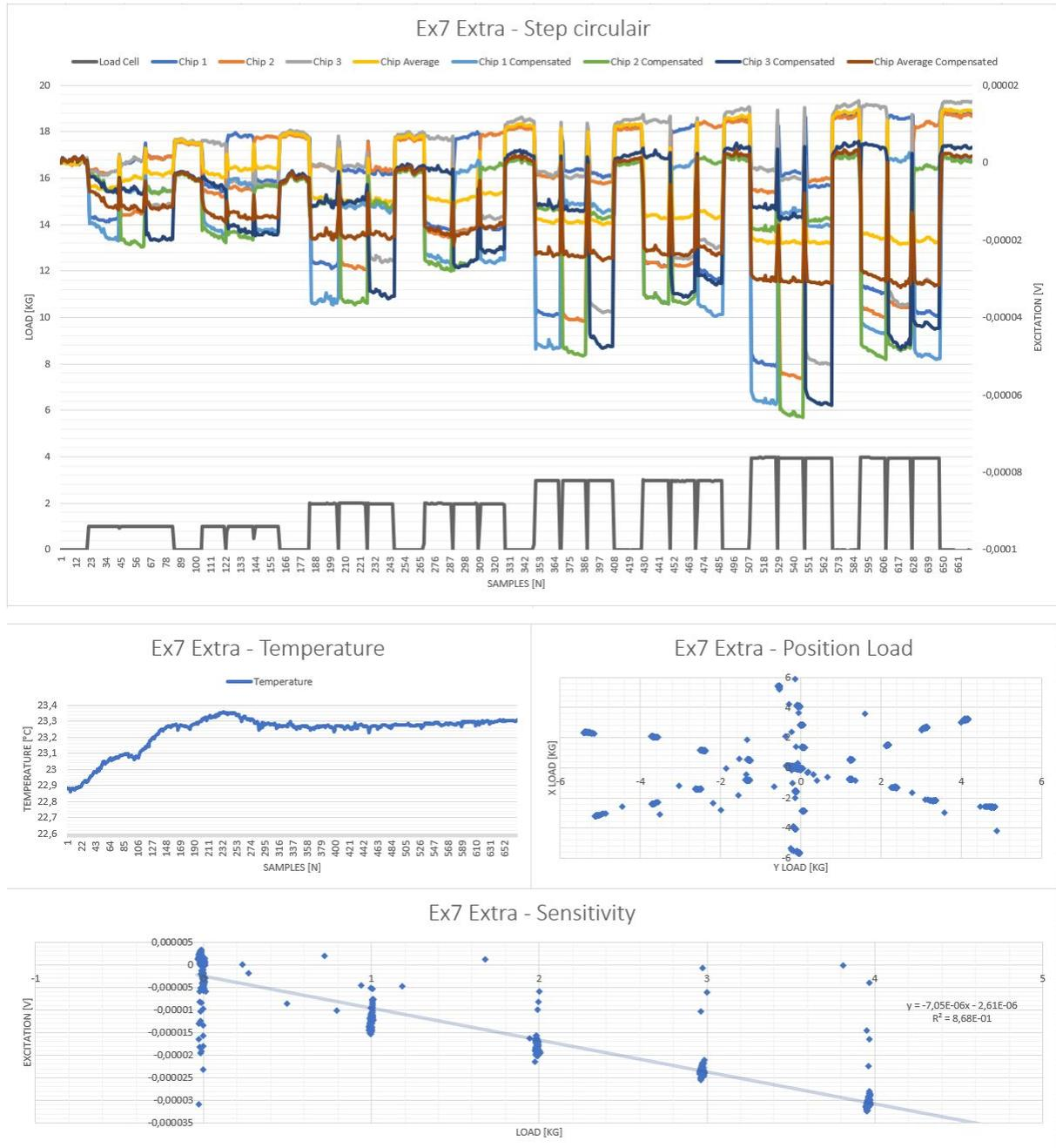
Output data of the load cell and the chips | Temperature data | position data | Excitation voltage vs load cell output with a linear trendline through the points
