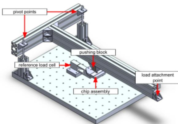
Figure 13, Render of test setup 1
