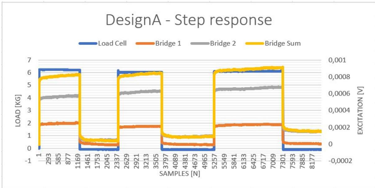
Figure 24, Step response measurement design A with a sample time of 1/3Hz
