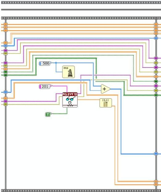
Temperature measurement<sup>9</sup> (read out the data acquisition unit)
