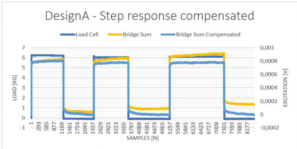
Figure 25, Compensated step response measurement design A with a sample time of 1/3Hz
