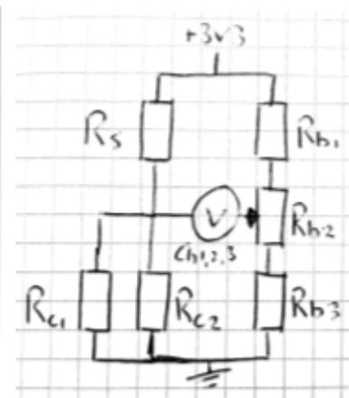
Figure 18, Connection schematic design B with external half bridge
