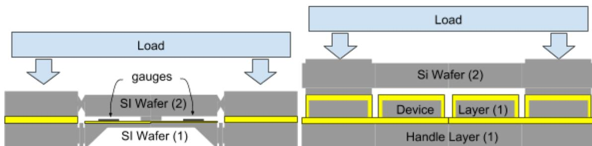
Figure 1, Wensink his device using two stacked SI wafers (1,2) using a membrane to create stress in the gauges (not to scale) Figure 2, Zwijze his device using one SOI wafer (1) and a second Si wafer (2) to prevent strain in the reference gauges (not to scale)
