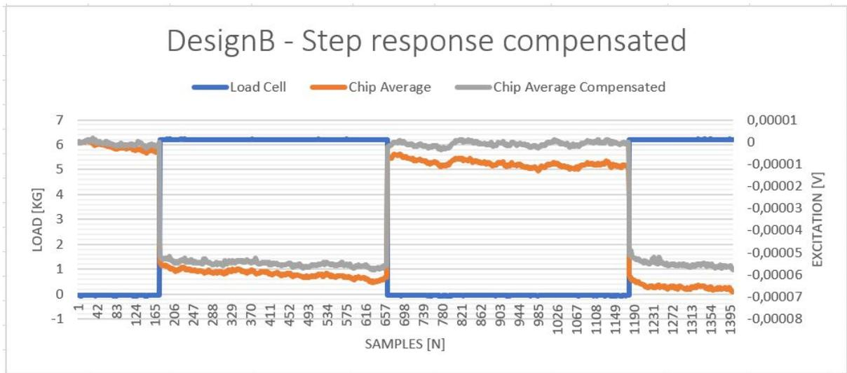
Figure 29, Compensated step response measurement design B with a sample time of 2/9Hz
