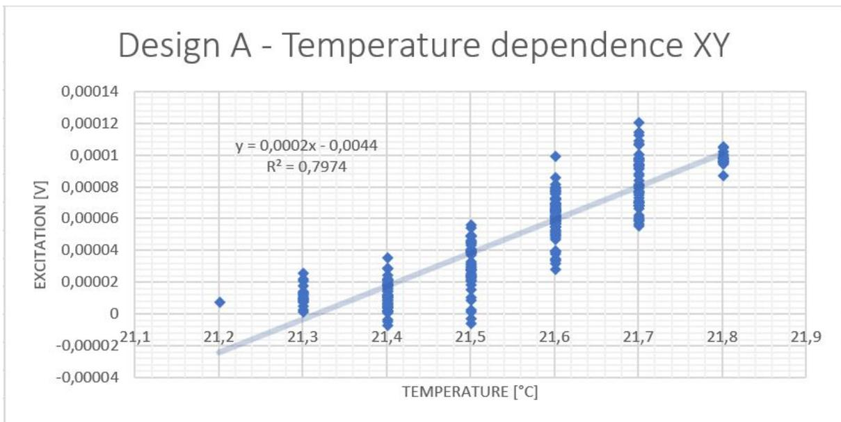
Figure 20, Temperature vs excitation design A with linear trend line
