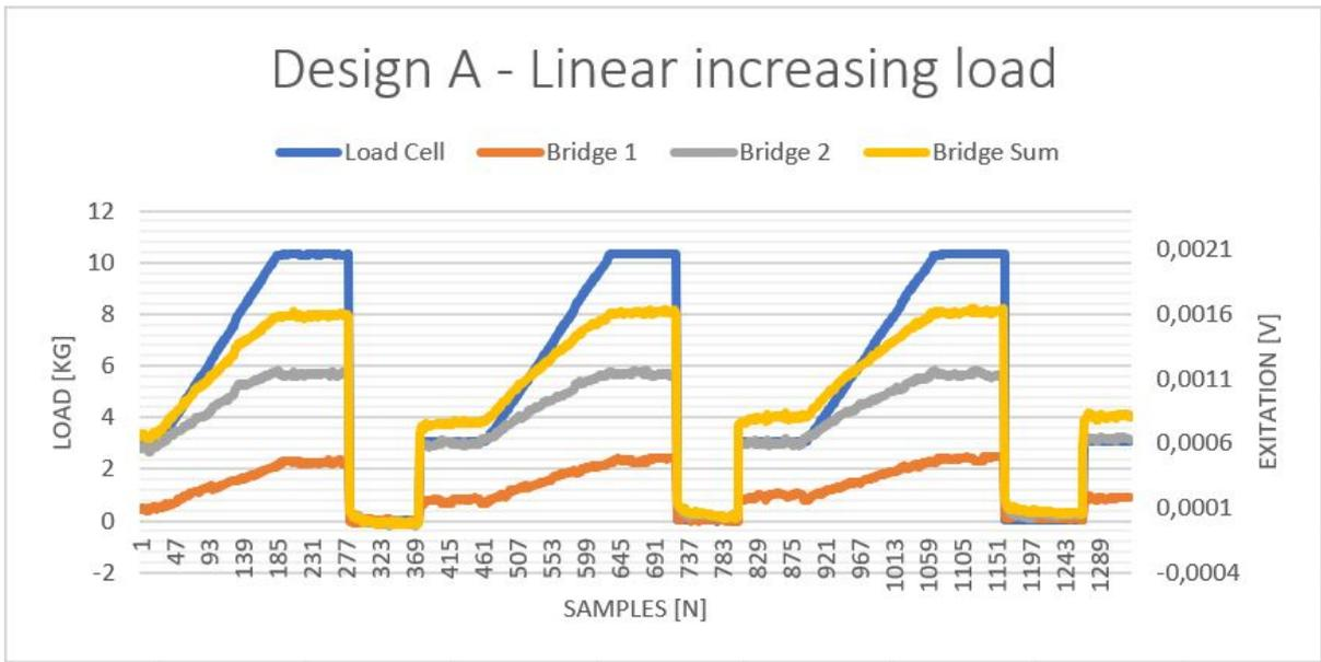
Figure 32, Linear response measurement of design A with a sample rate of 1/3Hz
