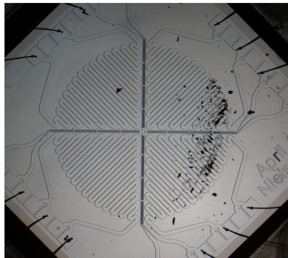
Figure 37, Design A after an asymmetric loading
