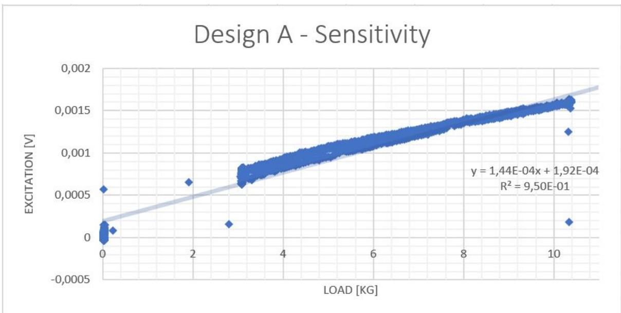
Figure 33, Sensitivity plot of design A of a linear loading
