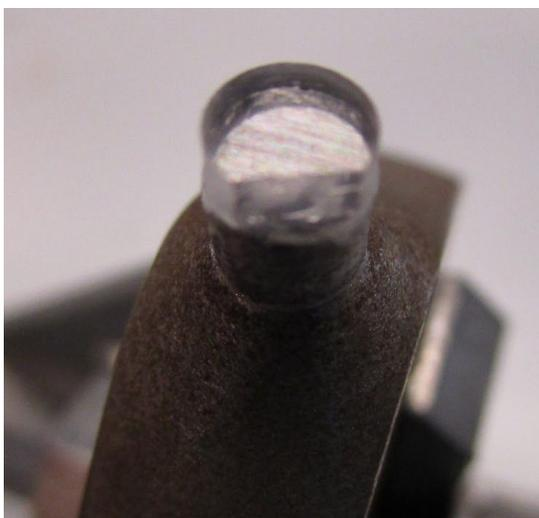
Figure 36, The glass pushing block after asymmetric loading
