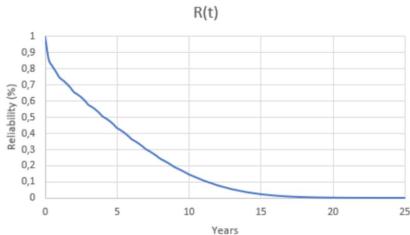
Figure 4-8: Reliability of the rotor system (considering major repair & replacement)
