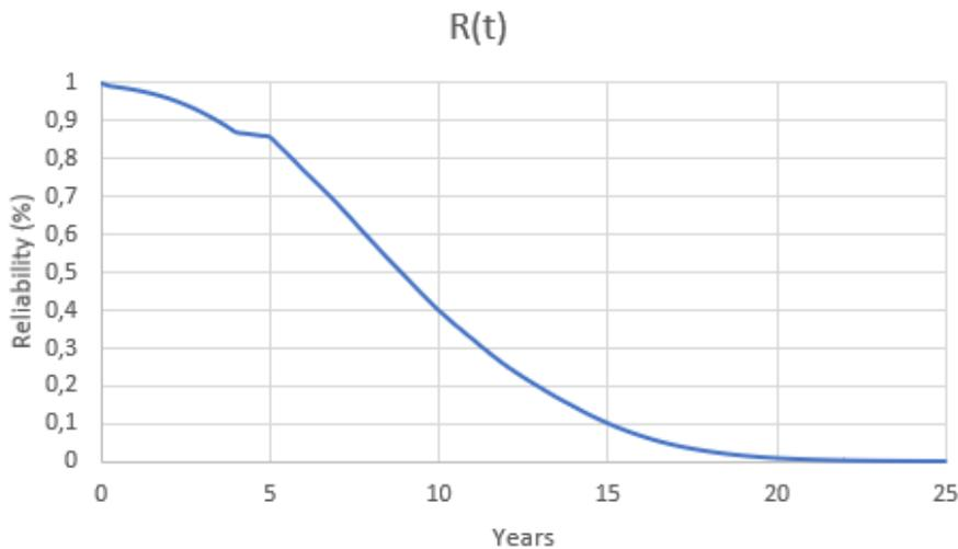
Figure 4-5: Reliability of the rotor system (only considering replacement)
