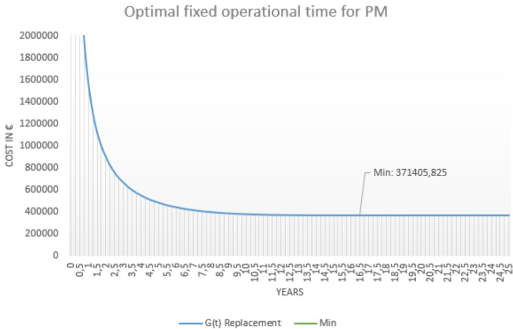
Figure 4-9: Optimal fixed operational time to schedule PM of the rotor system (major repair & replacement)
