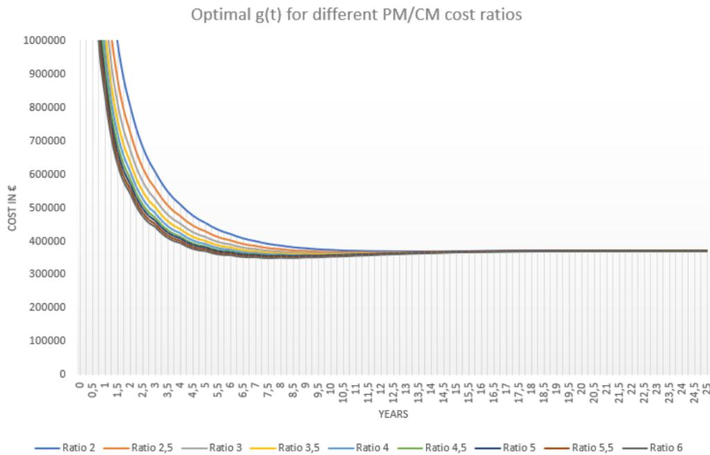
Figure 4-10: Optimal objective function  $g(t)$  for different CM/PM cost ratios (major repair & replacement of rotor system)
