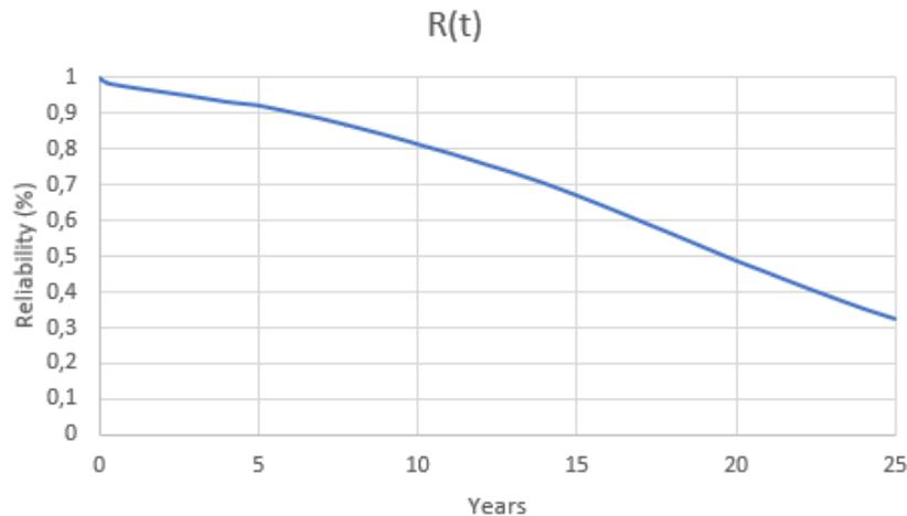
Figure 3-3: Reliability of the converter system
