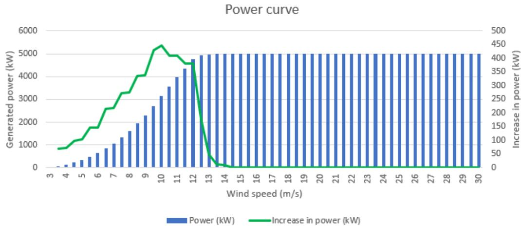
Figure 2-20: Power curve and the increase in power
