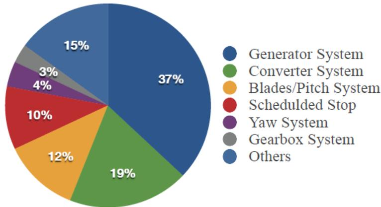
Figure 2-3: Percentage of downtime per component for two wind power plants in China (Zhao et al, 2017)
