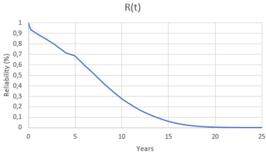
Figure 3-6: Reliability of the converter system (repair & replacement)
