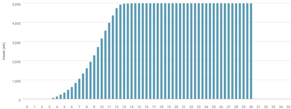
Figure 2-19: Power curve of the 5MW WT
