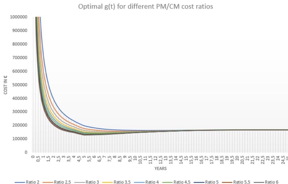
Figure 4-4: Optimal objective function  $g(t)$  for different CM/PM cost ratios (repair & replacement)
