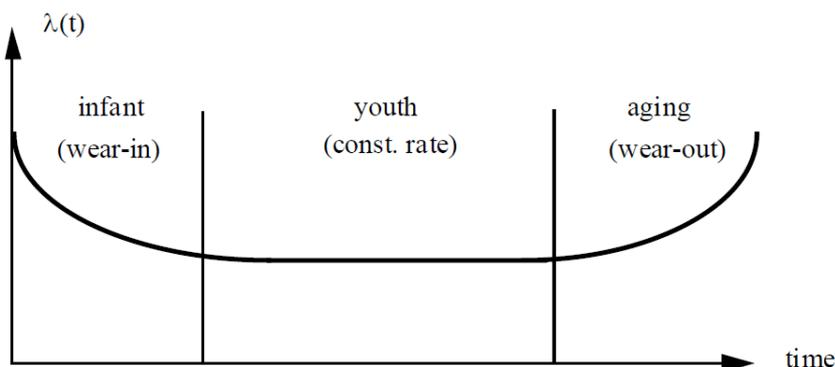
Figure 2-4: Bath-tub curve (Scheu et al., 2017)
