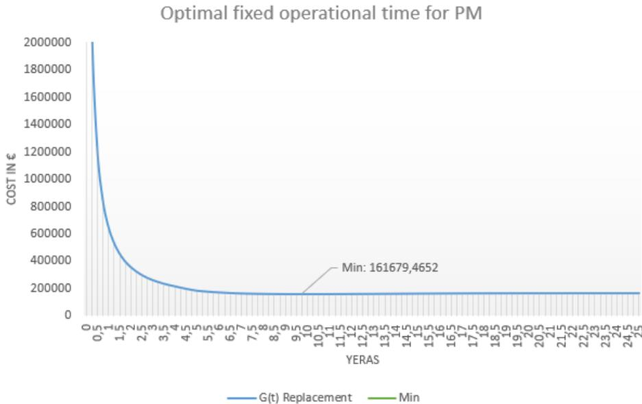
Figure 4-3: Optimal fixed operational time to schedule PM of a converter system (repair & replacement)
