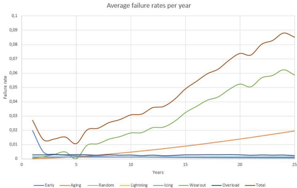
Figure 3-2: Average failure rates per year of the converter system
