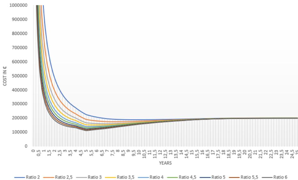
Figure 4-7: Optimal objective function  $g(t)$  for different CM/PM cost ratios (replacement of rotor system)
