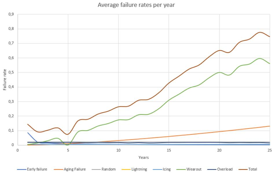
Figure 3-5: Average failure rates per year of the converter system (major repair & replacement)
