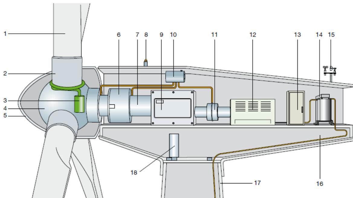
Figure 2-1: Main components of a WT
