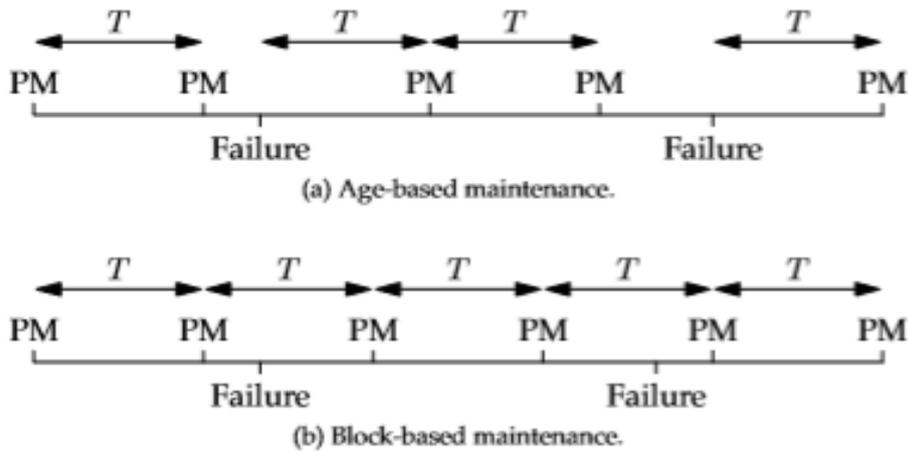
Figure 2-15: Scheme of time-based maintenance policies
