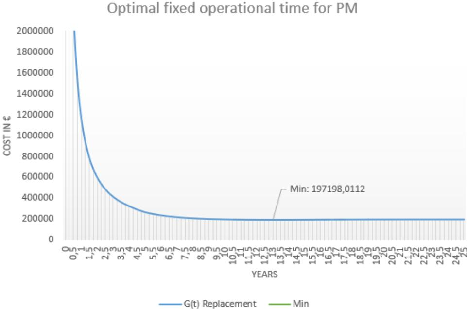
Figure 4-6: Optimal fixed operational time to schedule PM of the rotor system (replacement)
