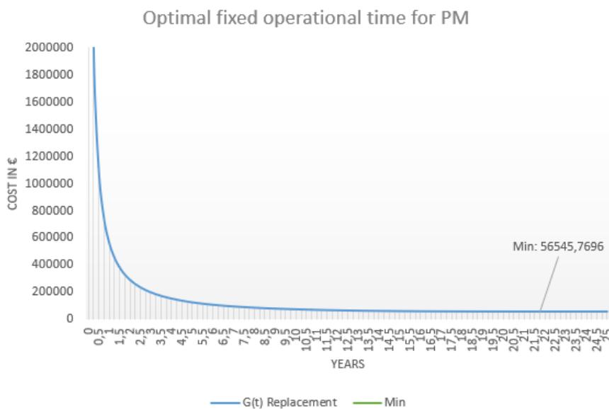
Figure 4-1: Optimal fixed operational time to schedule PM for a converter system
