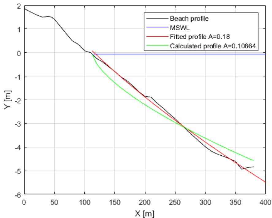
Figure II-1. Submerged profiles fitted to the beach profile. The submerged profiles were made with a fitting algorithm (red) or calculated from the D50 (green). The red profile was used.
