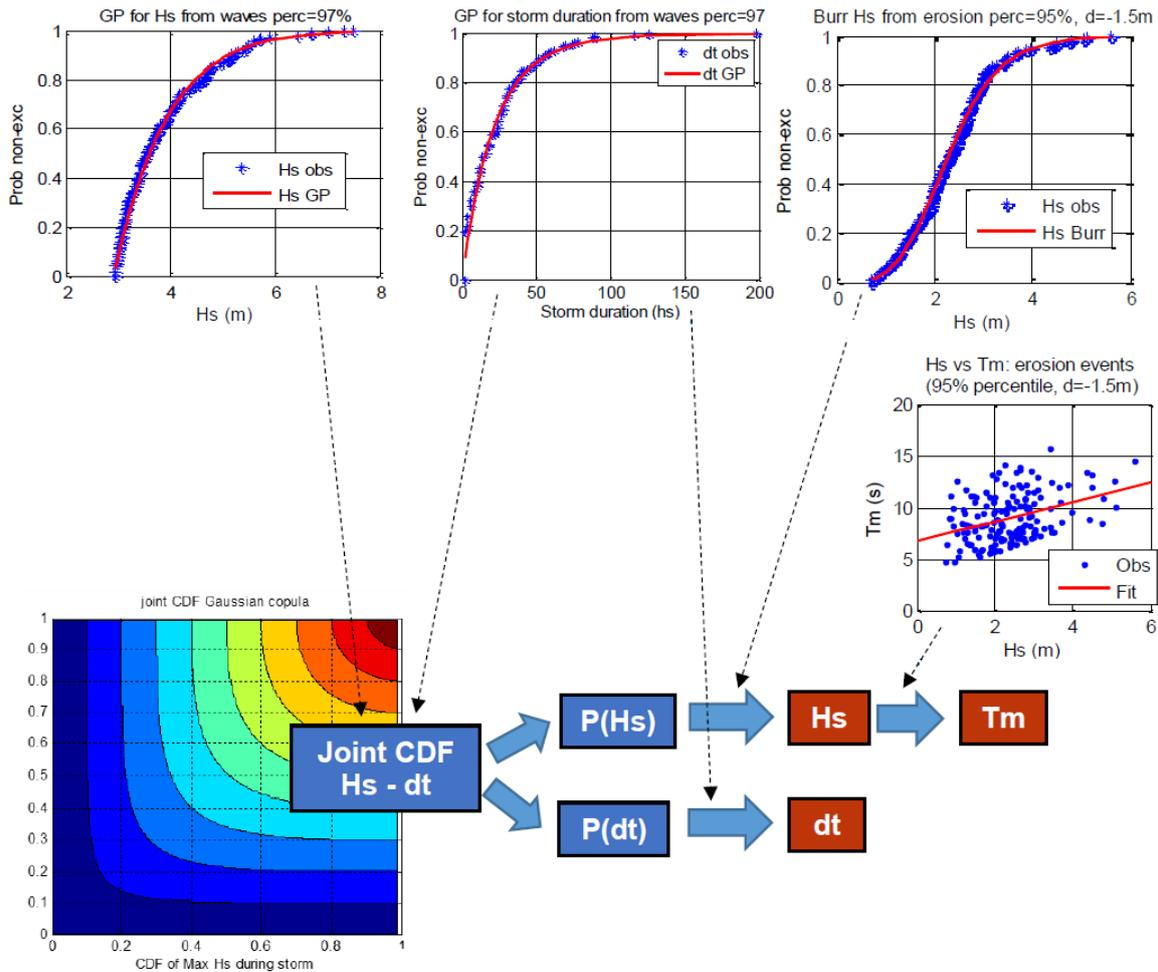
Figure 2-6. Setup for storm generation. Adopted from Da Cruz (2018).
