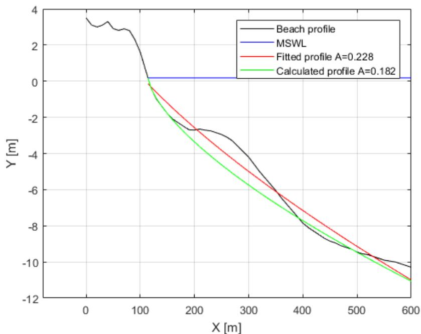
Figure II-3. Submerged profiles fitted to the beach profile. The submerged profiles were made with a fitting algorithm (red) or calculated from the  $D50$  (green). The green profile was used.
