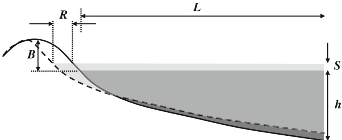
Figure 2-3. The evolution of the equilibrium beach profile according to the Bruun rule. The solid line is the initial equilibrium profile and the dashed line is the equilibrium profile after SLR. The dark grey shaded area represents accretion and the light grey shaded area represents areas where water is present after SLR. Adopted from (Ranasinghe et al., 2012)
