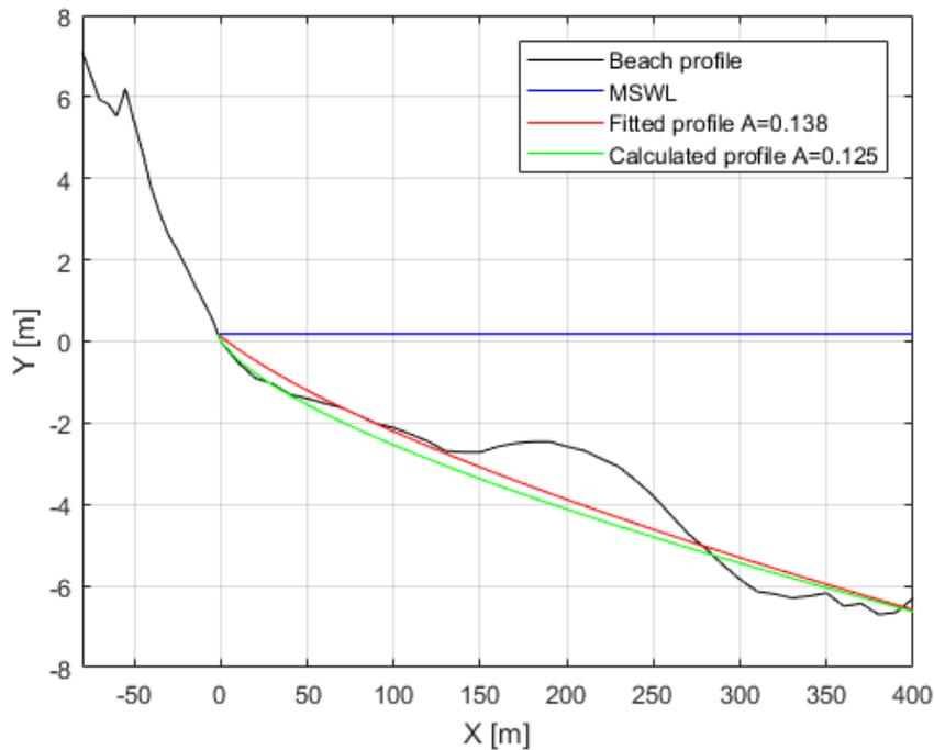
Figure II-2. Submerged profiles fitted to the beach profile. The submerged profiles were made with a fitting algorithm (red) or calculated from the  $D50$  (green). The red profile was used
