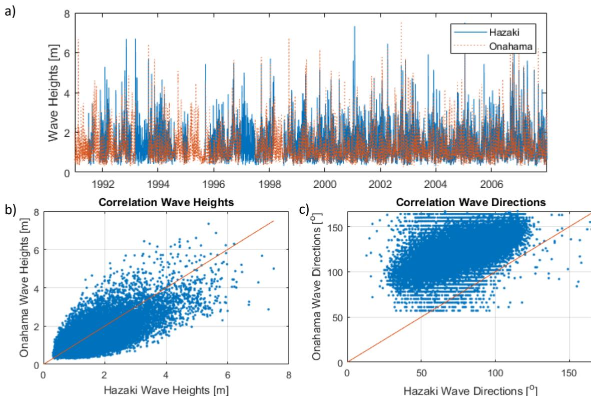
Figure 4-1. Comparison between Hazaki and Onahama. The time series were plotted a) in time (wave heights), and against each other with b) wave heights wave directions and c) wave directions (with north being 0°). The red lines in b) and c) represent the line on which the points should be if the values of both locations would be exactly equal at the same time.
