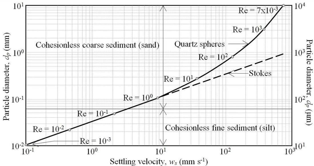
Figure 2-8. Particle diameter as a function of settling velocity for quartz spheres and Stokes law. Adopted from (Mehta, Khare, & Andrew, 2016)
