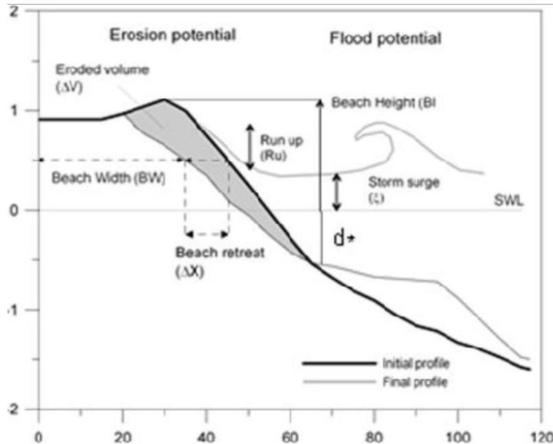
Figure 2-7. A schematisation of the storm-induced beach profile changes, according to the Mendoza-Jiménez model. Adopted from Jiménez et al. (1993) in: (Dastgheib et al., 2017).
